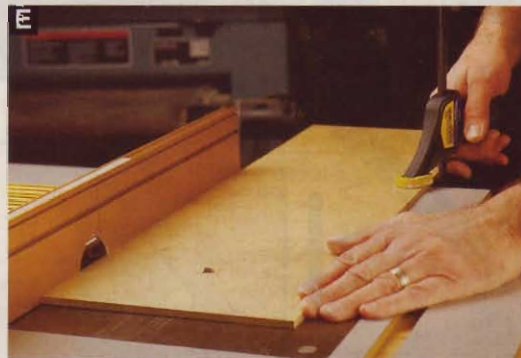
Above Clamp the panel-groove template to the router table to stabilize it when you raise the bit.
