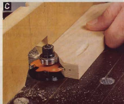
Cut the spline slots in the bottom shelf frames with a 1/8" slot cutter in a table-mounted router with fence.
