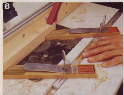
Mark the bit location on your fence. Stop routing when the stop line on the extension aligns with the mark on the fence.
