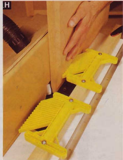
Mount featherboards on a wood bar to bear on the panel above the bit.
