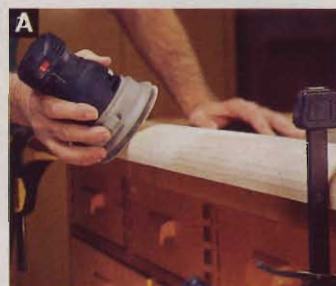
Clamp the rails to your bench, and keep the random-orbit sander in constant side-to-side motion to remove facets.
