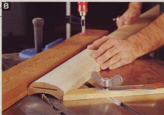
Use a feather board and a slow, but steady, feed rate to cut a consistent cove with minimal sawtooth marks.
