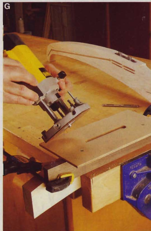
Position the fence of the bed-rail fastener mortise template on the inside edge of the leg, and align the centerlines.
