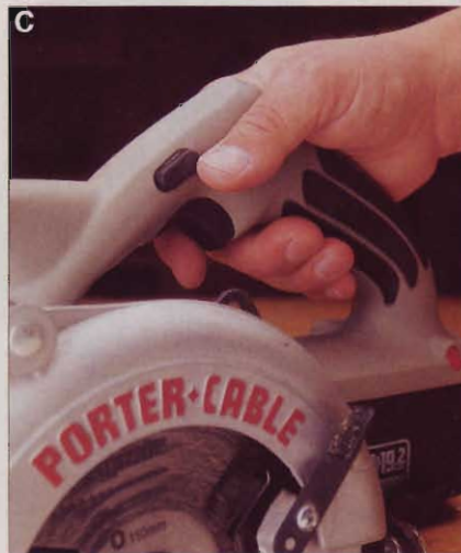
C We found the safety release button on the Porter-Cable saw difficult to reach with our hands in operating position.
