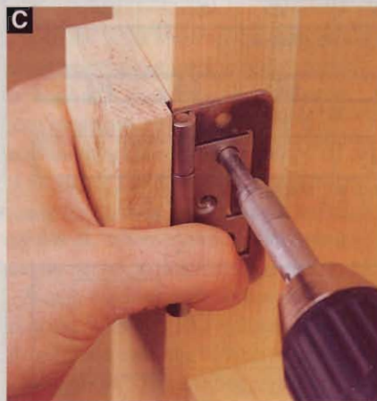
The hinge knuckles protrude ¼" beyond the legs. A simple scrapwood guide ensures accurate positioning.
