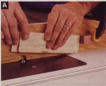
With its right end against one stopblock, lower the back (B) onto the running bit. Then move the back to the left until it contacts the other stopblock.
