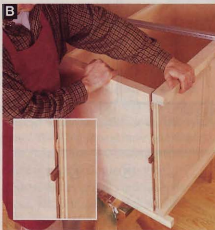
When popping the top in place, a short block of wood, inset photo, helps to lever the sides apart.
