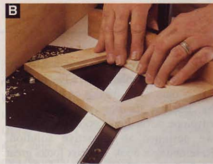
Rout the corner tab recesses, making multiple passes until the frame's corners ride against the fence.
