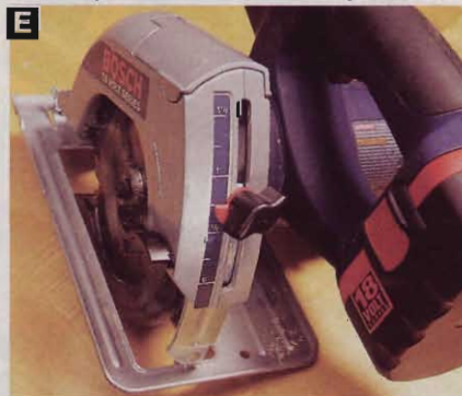
Clear markings and good location make Bosch's depth scale the best in the test. The door on top of the blade guard opens to accept a dust-collection hose.
