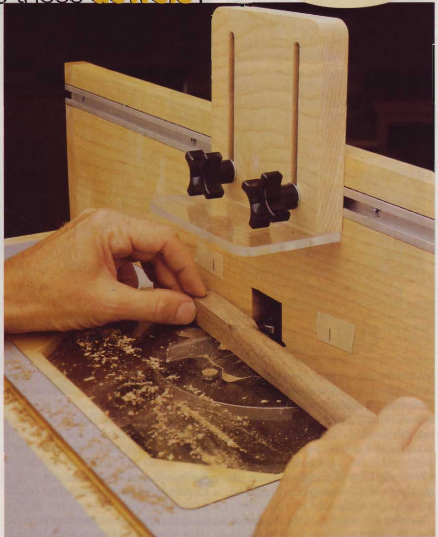
We raised the guard for clarity in this photo. Keep it low while you're making dowels, to ensure that your fingers stay well away from the router bit.
