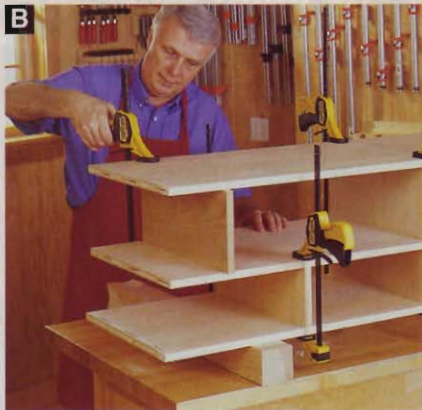
Scrap 4x4s make room for clamp heads underneath the assembly, while spacers keep the lower drawer shelf aligned.
