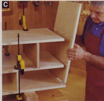
Leave the spacers in place while gluing and clamping the carcass sides. With the glue dry, remove the spacers.
