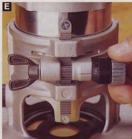
E The tool's weight makes it difficult to make fine adjustments using DeWalt's rack-and-pinion depth mechanism.
