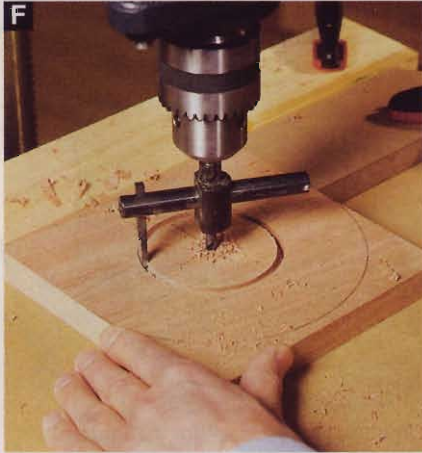
F For safety, run the circle cutter at the slowest speed on your drill press, and use a fence and stopblock to secure the blank.
