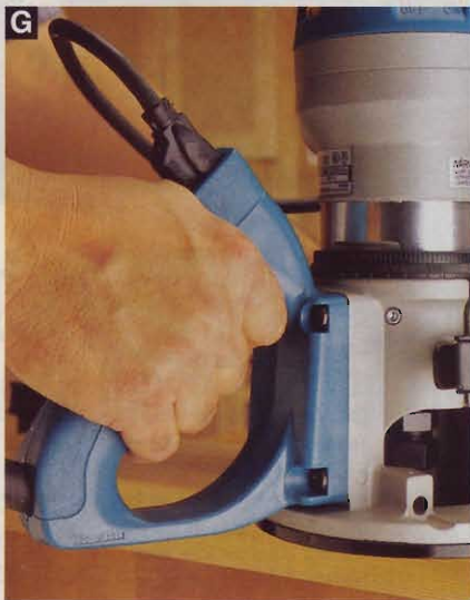
G A D-handle base puts the power switch at your fingertips and helps you control the lateral pressure for bearing-guided cuts, such as round-overs.
