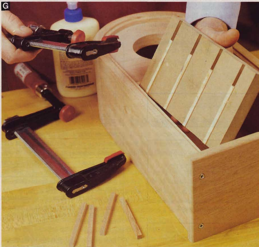
G A simple jig made by cutting dadoes in a scrap of MDF allows you to glue four drawer guides inside the clock case at one time and in perfect alignment.
