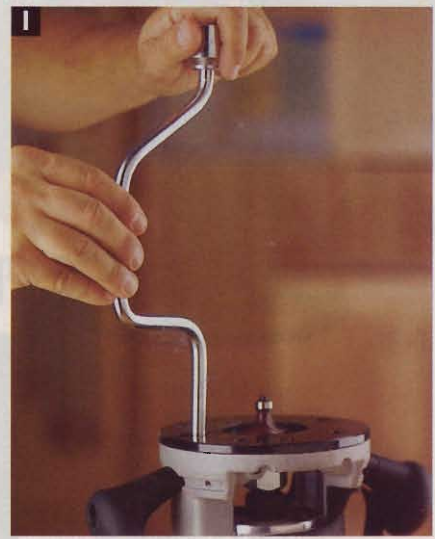
I Milwaukee's built-in, through-the-base depth adjustment is a big plus if you plan to table mount your router. (Shown out of table for clarity.)
