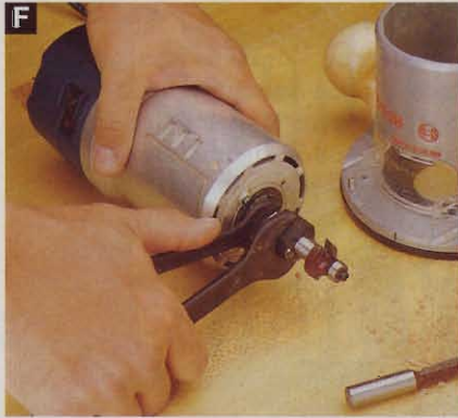
F Removing the motor from the base of the Bosch (shown), DeWalt, Makita, or Porter-Cable routers provides unlimited wrench room when changing bits.
