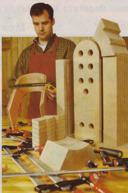
Design Editor Kevin Boyle learned a lot about cold-lamination techniques in his experiments on building the arched-top cabinet clock carcass.
