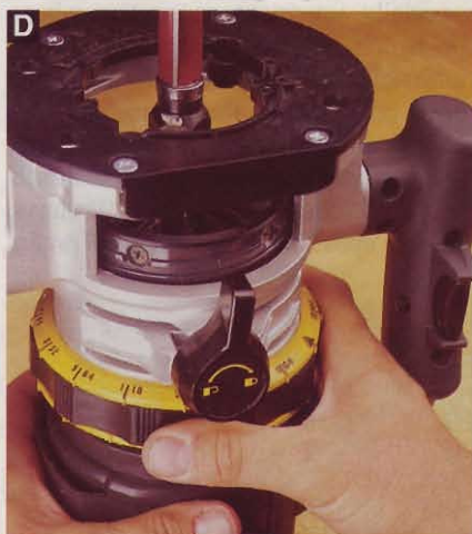
D One full turn of Craftsman's twist ring yields only 1/4" change in cutting depth, so large changes take longer.
