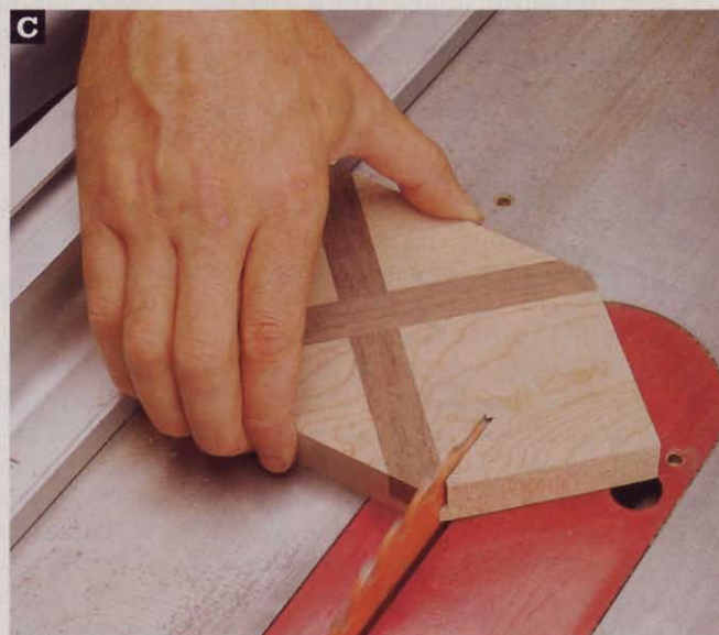
To reduce the chance of kickback when cutting short pieces, keep the blade low and hold each coaster securely against the fence as you make the cut.
