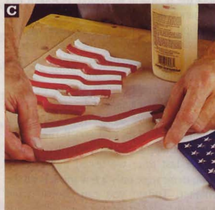
Working down on the left from the field to the flag's bottom edge, then back up on the right, glue the stripes in place.
