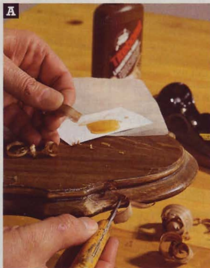
A Glue plane shavings into the crack to provide a base for the filler. A knife helps push the thin pieces into place. The crack to the left of the knife has been trimmed and sanded already.
