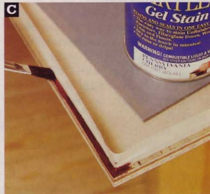
C Mask the rabbet's edge to keep the stain from accidentally bleeding onto the panel's surface.
