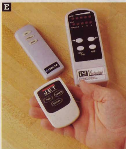
Jet's remote control is easy to tuck into a pocket (or misplace on a bench). Penn State's control can be mounted to a wall, like a wireless switch.
