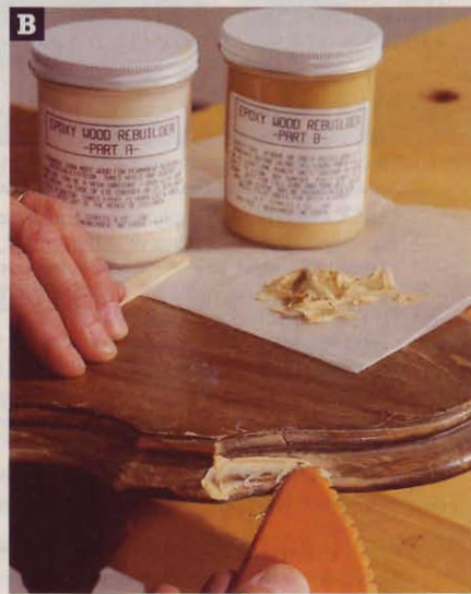
B Smooth wood filler onto the repaired area after trimming the glued-in plane shavings flush with the surface. Make sure to use a filler that will take stain. We chose a two-part epoxy product.
