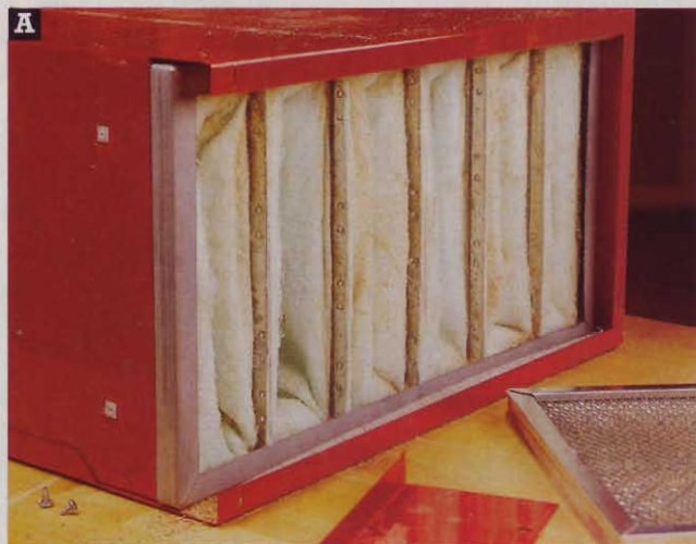
Craftsman's relatively coarse prefilter allowed large particles into the bag filter. Note that to take out the prefilter, you must first remove two screws and an access panel.
