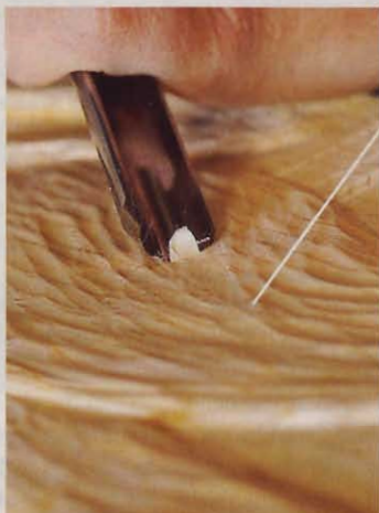
#9 sweep, 13mm gouge This blade digs shallow trenches.
