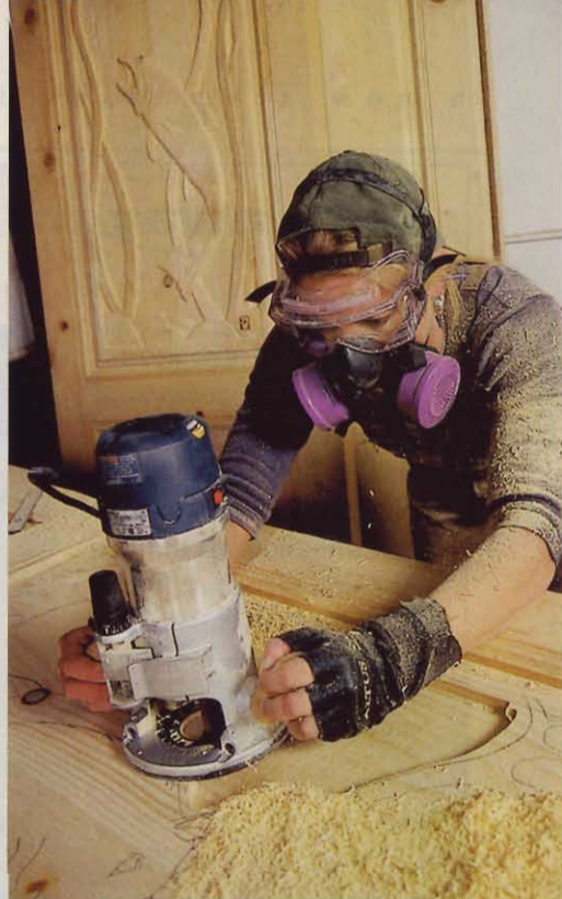
To give her relief carvings depth, Amber routs the background around the central figures 1/2" deep.
