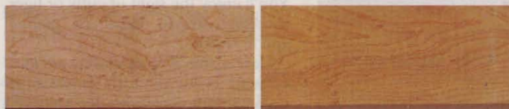
Maple with a water-based finish (left) is whiter than the amber-toned sample coated with an oil-based finish shown at right.
