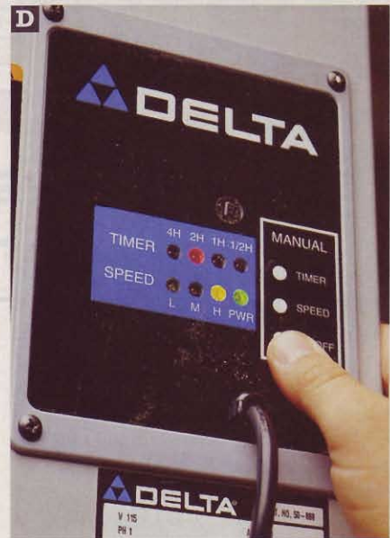
Touchpad controls are sealed from the outside to reduce dust penetration to the switches.
