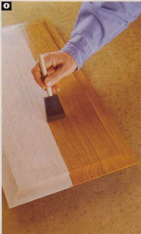
O If you plan to stain your cabinet door, do the panel before assembly. The clear topcoat can wait until after assembly.
