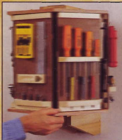
Spin the entire carousel to access each of its six tool-holding wings ...
