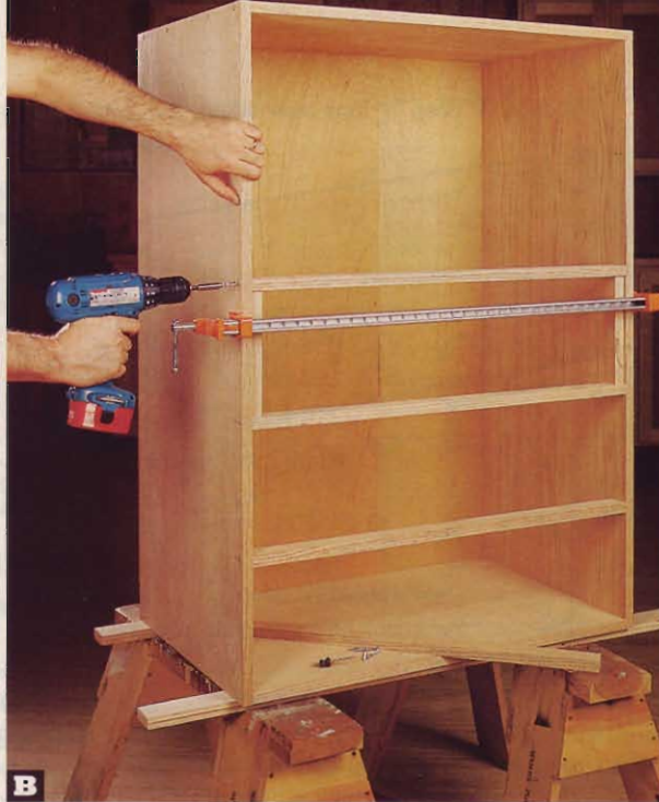
B Position the dividers in the carcass using two \frac{3}{4} \times 1\frac{1}{2} \times 8\frac{1}{8} " spacers. Clamp the carcass sides to snug the divider. Drill the holes and drive in the screws.
