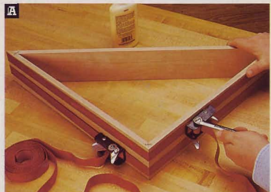
Set the assembled frame on a flat surface, and draw its mitered corners together with a pair of bandclamps.
