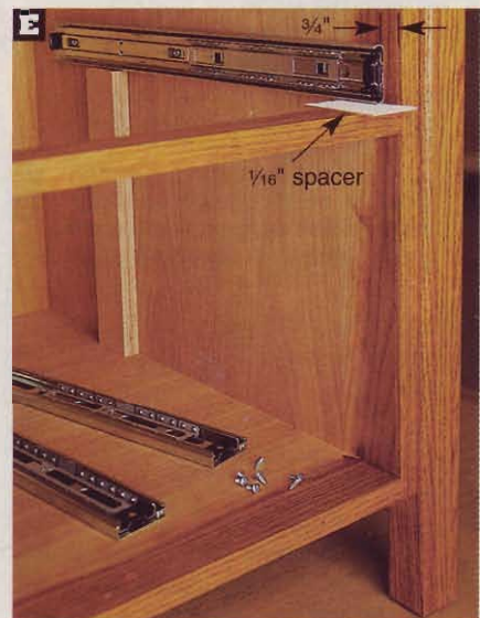
Locate the cabinet-member part of a slide \frac{3}{4} " back from the front of the carcass while supported on the wood spacer at the rear and \frac{1}{16} "-thick spacer at the front.
