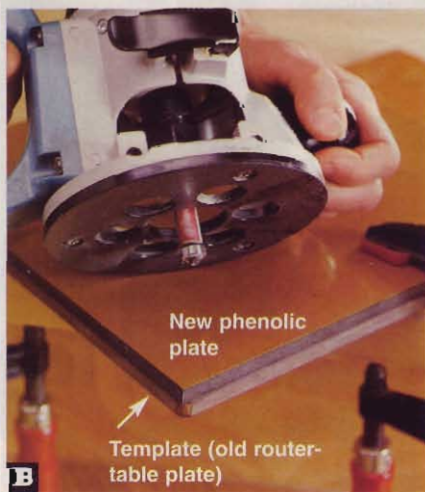
B Flush-trim router bits work great with plastic. Here we're shaping a router table insert plate from phenolic laminate.
