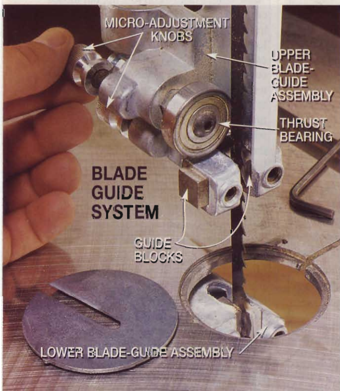
A micro-adjustment knob, like this one on the Delta, moves the thrust bearing forward or backward for precise positioning behind the blade. The lower knob controls the location of the guide blocks.
