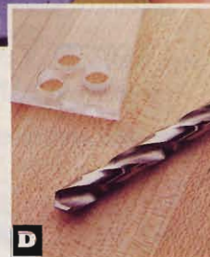
C Plastic can shatter or climb the bit when you use a standard twist bit. Grind your bit to turn it into a rotary scraper, and you can put clean holes right near the edge of a piece.
