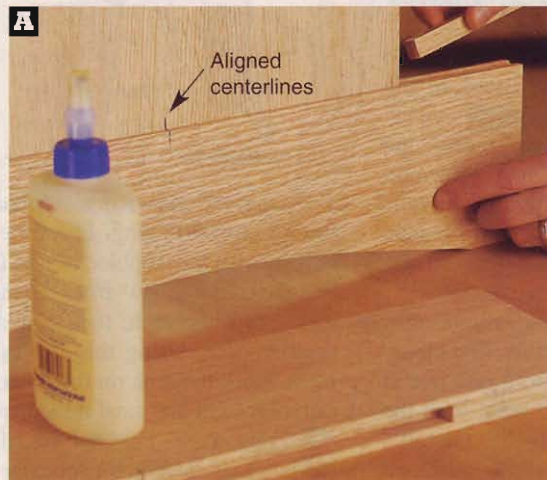
With the panel and rail centerlines aligned, glue and clamp spacers in place, tight to the panel and flush with the ends and top surface of the rail.
