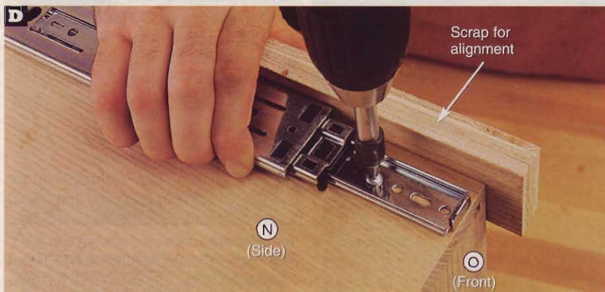
Place a slide on a drawer side flush with the bottom and front edges. You'll need to open the slide a little to drive in the screws.
