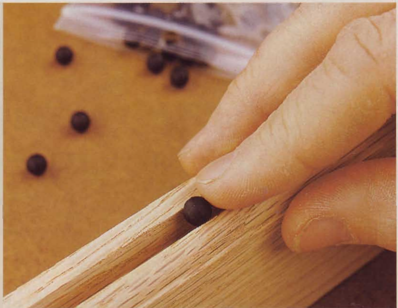
Push the Space Balls into the grooves as far as you can with your finger. The panel will seat them during assembly.
