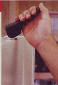
Shop Fox's tension lever rotates to adjust blade tension, then flips up to relax the tension for extended blade life.
