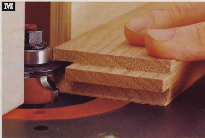
M Make the long-grain cuts on all four frame pieces. Your fingers are close to the bit, so be sure to keep your right hand at the outside corner as you push.
