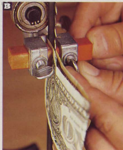
B A dollar bill wrapped around the blade helps set the saw's guide blocks.
