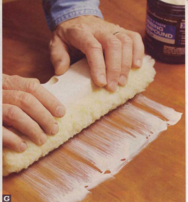
G A lamb's wool applicator like the one shown here gives you room to grip with two hands and apply pressure as you rub. The rubbing agent being used on this tabletop is a fine automotive compound.
