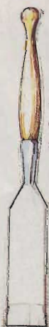
Slick: Looks like an oversize chisel but used as a plane for smoothing tenons.
