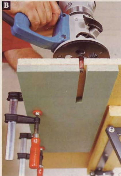
With the slot template (painted green for clarity in this photo) guiding the flush-trim bit's pilot bearing, rout the slot in the end (C).
