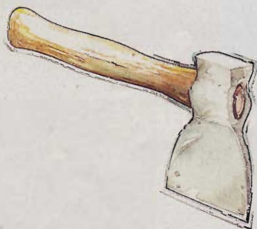
Broad ax/hatchet: For hewing and dressing timbers, plus roughing out joinery.
