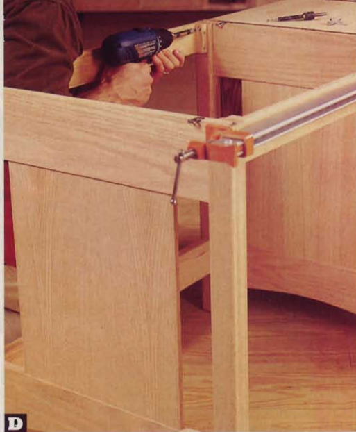
D Clamp the crossrails between the side panel and the drawer carcass. Drive screws through the cleats into the legs to secure.
