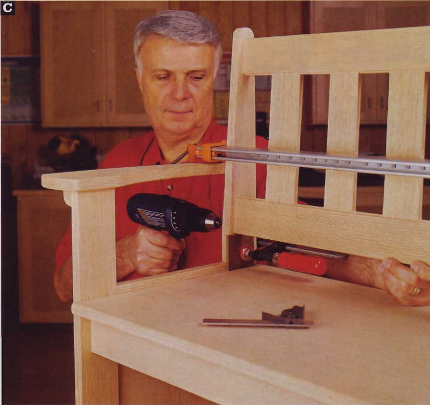
C Rest the back assembly on 2½"-wide spacers, and clamp it in place. Using the shank holes in the rear uprights as guides, drill pilot holes, and drive in the screws.
