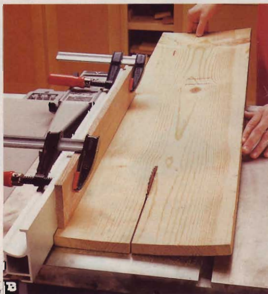
B Rip cupped boards with the convex face against the saw table. A scrap clamped to the fence guides the workpiece and holds the portion being cut flat against the table.
