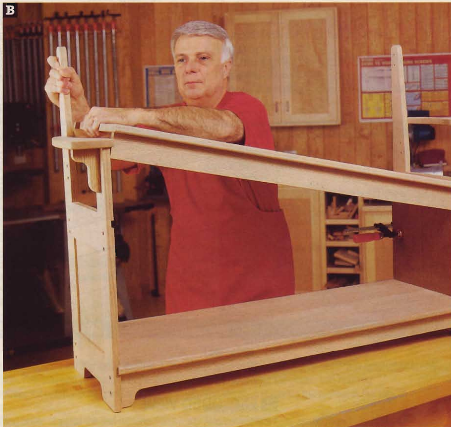
B With one end of the seat assembly resting on a spacer, flex the opposite side assembly just enough to allow you to lower the seat's other end into its dado.
