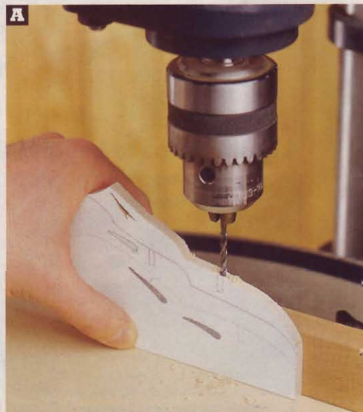
Using your fence to align the workpieces, drill the \frac{1}{8} " tree-mounting holes in the mountains, centered on their thickness.
