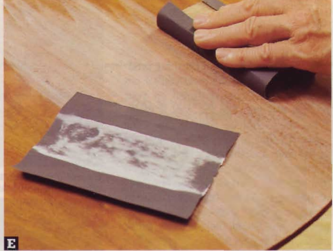
E Sanding lacquer with fine wet/dry sandpaper and no lubricant turns the top layer of finish into a white, powdery dust. Change paper often to avoid scratches from corning. When you're done with this step, clean the surface with a rag or a blast of air.
