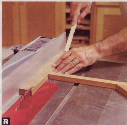
B If one pass won't produce enough spline stock, clamp a stop to the table before ripping. Slide the fence between cuts to set the board against the stop.
