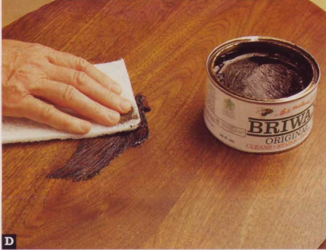
D Small scratches showed in this walnut table finished with an oil/varnish mix, so we rubbed it with an abrasive pad, using dark brown wax from Briwax. (Item number 85C28 in the Woodcraft catalog, priced at $12.50; call 800/225-1153 to order.)
