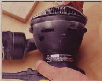
Craftsman and Ryobi sanders come with a smooth pad for PSA paper, but also include an adhesive-backed adapter disc so you can use hook-and-loop discs. Sometimes, the hook-and-loop holds better than the adhesive, and the adapter comes off with the sanding disc.
