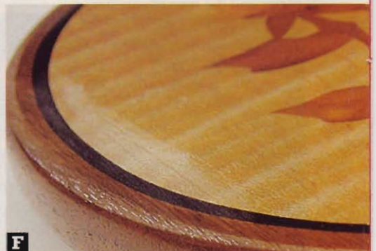
F When you don't have much finish to work with, it's all too easy to rub through it and expose the bare wood, as shown here on a handheld mirror.
