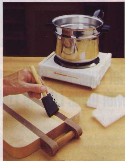
To melt wax, fill the lower part of a double boiler with water, put paraffin in the upper unit, and set the heat on low.
