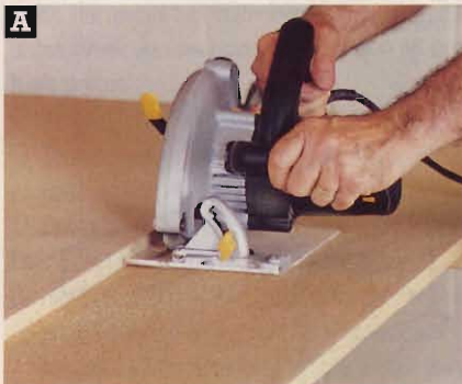
A Using the edge of a second sheet to guide your saw, cut the first part A to width. Save the cutoff for a straightedge for cutting the other parts.
