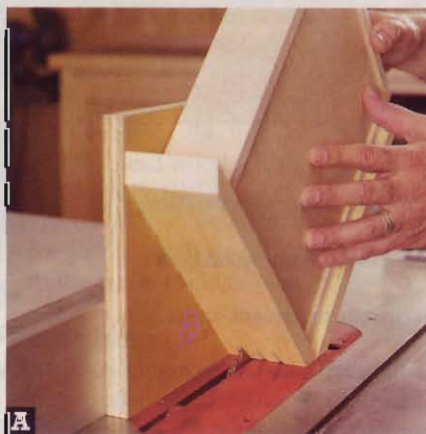
A Double-check the orientation of your workpiece before cutting. Here we're holding the bottom of the tray to the left, so the slots will point downward.
