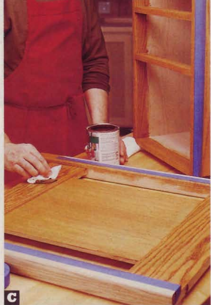
C Mask mating glue-joint areas along the front and back edges of the carcass sides and on the inside of the side-panel legs with easy-release painters' tape. Then apply the stain.
