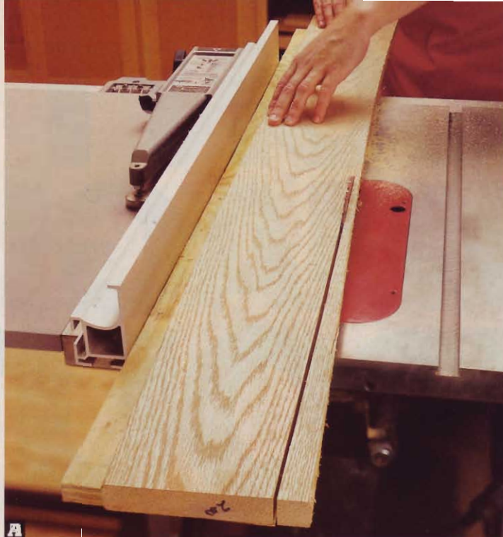
A To put a straight edge on a crooked board, stick it on a long, straight carrier, such as a strip of plywood (about \frac{3}{4} " \times 8" \times 60"), using double-faced tape. Guide the carrier along the tablesaw fence to rip off one bad edge.
