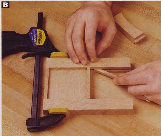
B Glue and clamp a long filler in each stile's groove, sliding it behind the bottom face-trim piece and tight against the face. Remove any squeeze-out.
