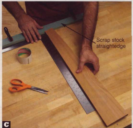
C Clamp a scrap stock straightedge to your workbench. Apply double-faced tape to the back of one center splat, and stick it to the bench so it is square to the scrap.
