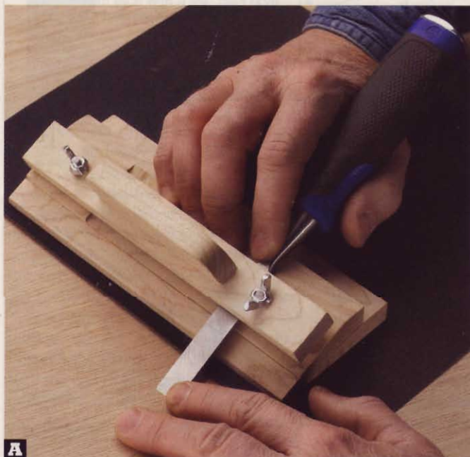
A You can place the chisel against either edge of the dado. Just make sure that it's flush with that edge, flat on the carrier, and has its beveled edge flat on the work surface.
