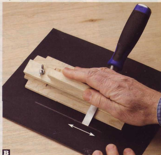
B As you begin to remove steel from the chisel, a line appears on the sandpaper. Move the jig away from the line to place the chisel on fresh abrasive. Your pressure on the jig helps keep the sandpaper in position.
