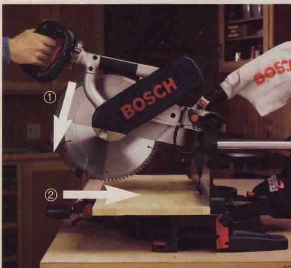
Just follow the arrows shown here for safe results on the radial-arm saw, top, and sliding mitersaw, bottom.
