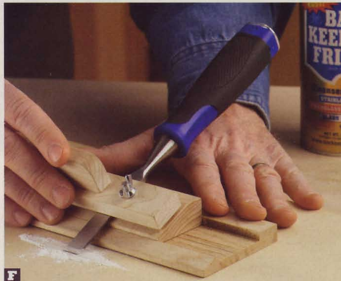
F Sprinkle some scouring powder on a flat surface, such as this medium-density fiberboard, and proceed as you did on the sandpaper. It doesn't take many strokes to thoroughly hone the edge.
