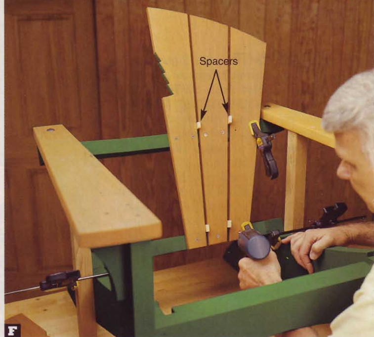
With a center splat in place, insert \frac{3}{8} " spacers, and add the rest of the slats, one at a time, drilling pilot holes and driving in the screws.
