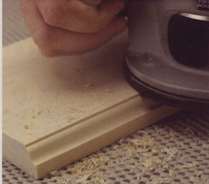
Poplar easily accepts decorative profiles and crisply holds machined edges. The wood rarely suffers tear-out or burn.
