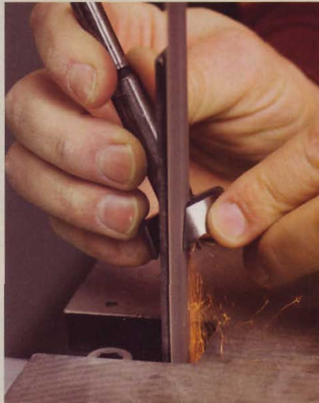
A strip sander quickly renews a dulled Forstner bit. Use 100-grit abrasive and a light touch, and keep the lifter flat against the sander's platen.
