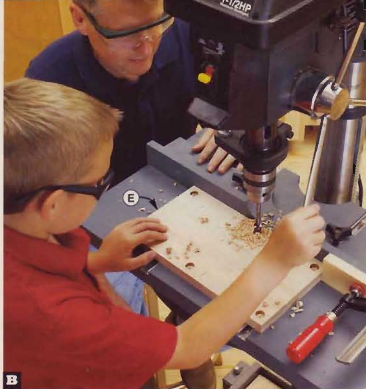
B With the stopblock positioned 5\frac{1}{8} " from the bit's center, drill a hole in the base (E), rotate the part 180^\circ , and drill another hole.
