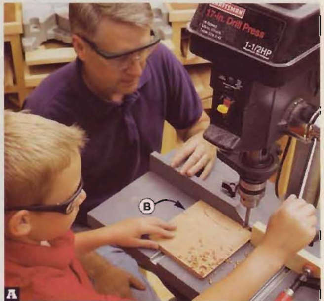
A With the case bottom (B) held tight against the drill-press fence and stopblock, drill a ½" hole ¼" deep in each corner of the part.
