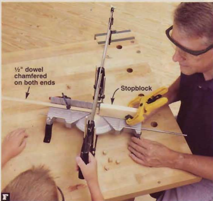
F Using a stopblock clamped to the miter-box fence, cut the \frac{1}{2} "-long feet from the chamfered ends of the dowels.
