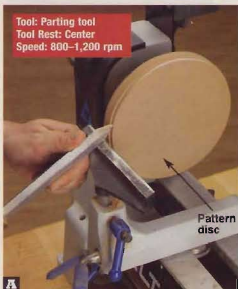
A With the pattern disc blank mounted on your 3" faceplate, use your parting tool to true the disc and turn it to a 6" diameter. As you turn, check the diameter with calipers.
