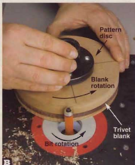
B Secure the trivet blank to the pattern disc with double-faced tape. With a flush-trim bit in your table-mounted router, trim the blank to finished size.
