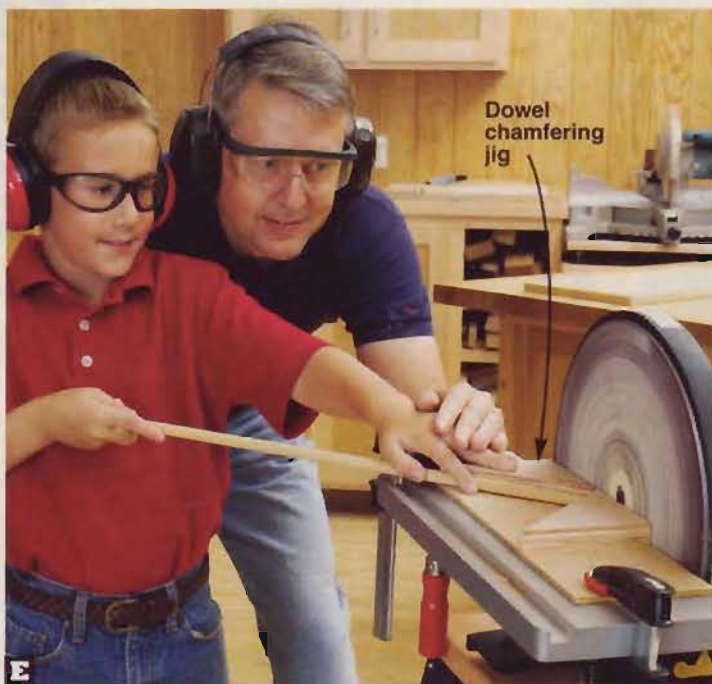
E Holding the dowel flat on the jig's base and tight against its angled stop, rotate the dowel 360^\circ to sand a \frac{1}{16} " chamfer on its end.
