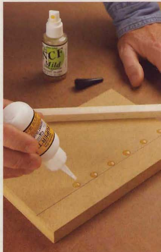
If you spread CA glue like other glues, it tends to remain liquid. Apply separate spots of CA glue, as shown here, to produce the instant bond that you want.
