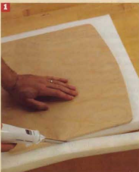
1 Adhere the oversize piece of foam to the seat with spray adhesive. Guided by the seat's edges, trim the excess foam with an electric carving knife or serrated bread knife. Be sure to keep the blade cutting vertically.
