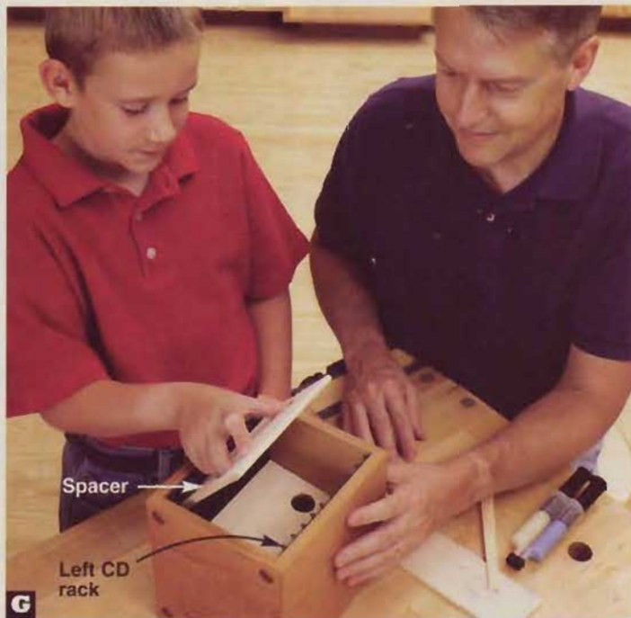
G Insert two spacers in the case, one at the back and the other at the front, to wedge the epoxied CD racks against the sides.
