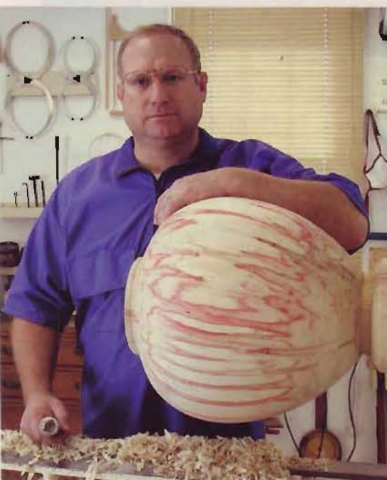
Author Bruce Hoover shapes a large hollow vessel from spalted box elder, characterized by the fungus-induced red streaks.
