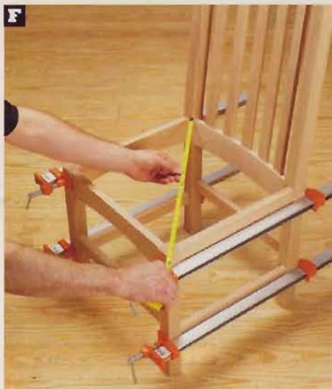
Check for equal diagonal measurements between the legs' inside corners to ensure square. Make sure the front legs are parallel to the back legs.
