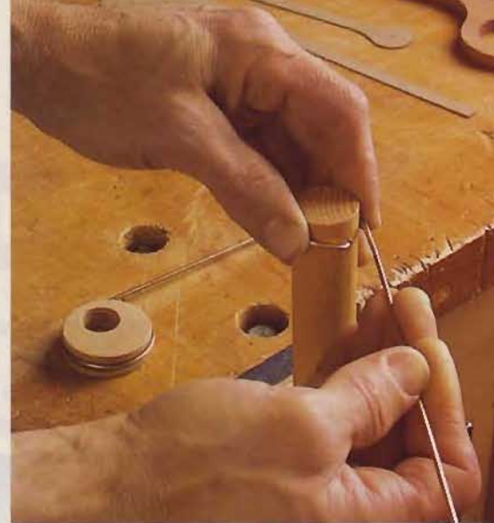
To create a brass pushrod, Mike inserts one end into a 1/8"-deep hole near the end of a closet rod. He pulls the rod around to create the radius, removes it from the pole, and nips off the starter end. The rod rides on a cam with a grooved edge, seen on the benchtop.
