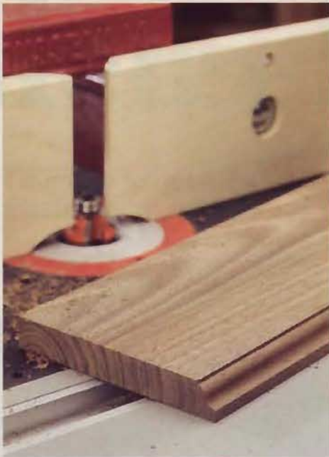
Walnut machines almost flawlessly with carbide-tipped bits and blades. The wood will blunt edges, so keep tools sharpened.
