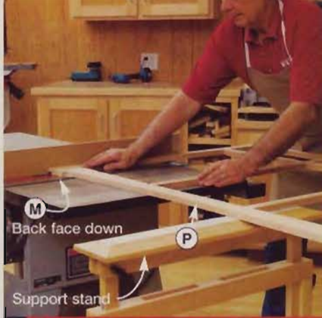
D RABBET THE FACE FRAME Keeping the face frame (M/N/O/P) tight against the saw's rip fence and supporting the frame with a stand, rabbet the back edges of the outer stiles (M).
