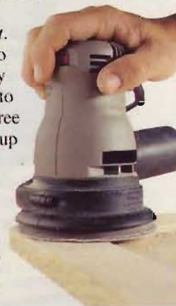
The pad on a random-orbit sander rotates and moves in an orbital motion to blend the scratches into a hard-to-see pattern.
