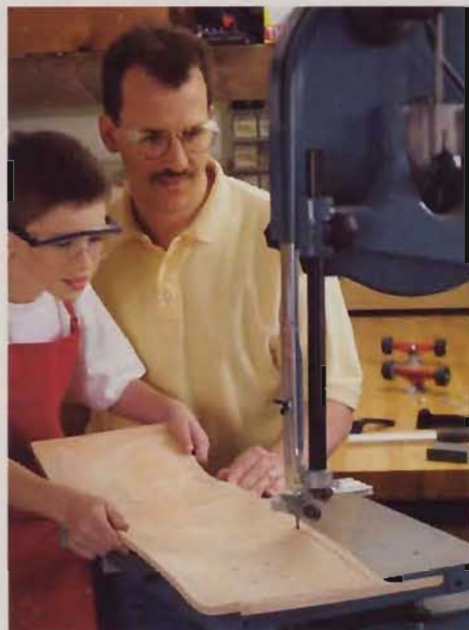
WOOD magazine's Products Editor Dave Campbell teams up with son Colby to bandsaw a skateboard wafer from a wafer blank, following the factory-drawn outline.
