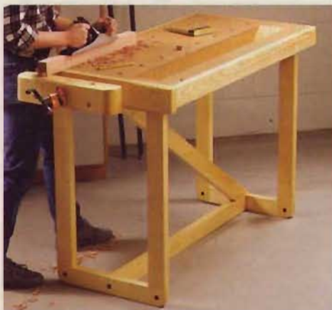
A workbench must be flat, sturdy, and stable. To make yours more useful, incorporate a vice and bench-dog holes that ease holding chores. Get plans for this easy-to-build bench at www.woodmagazine.com/workbench .
