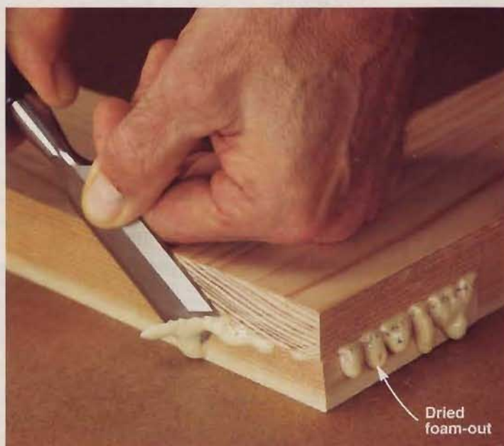
The foam produced by polyurethane glue easily fills gaps, but it doesn't produce any strength. Make sure the joints fit tightly before you glue them together.
