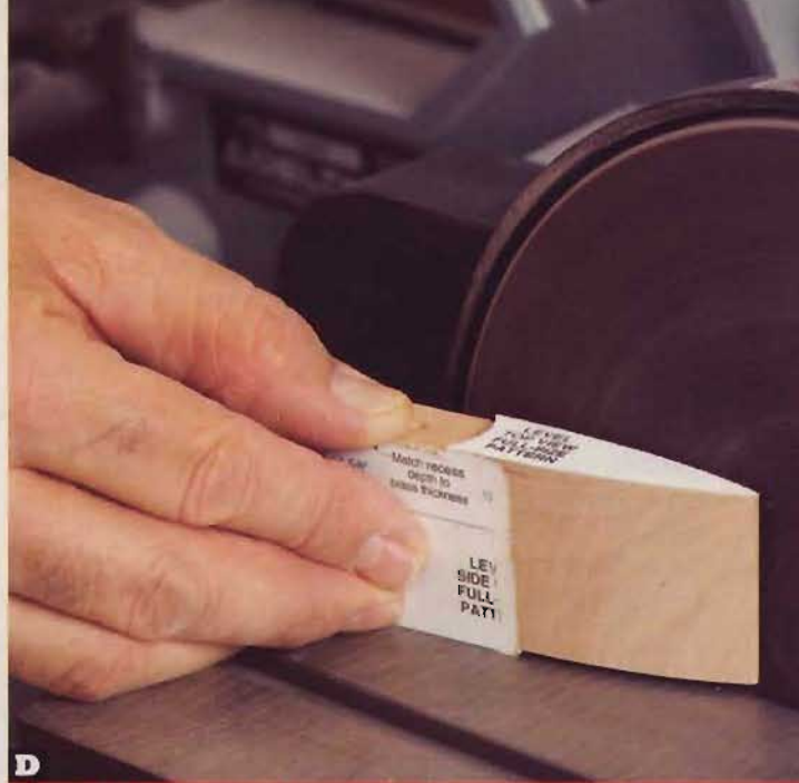
SAND THE LEVEL'S TAPERED ENDS
