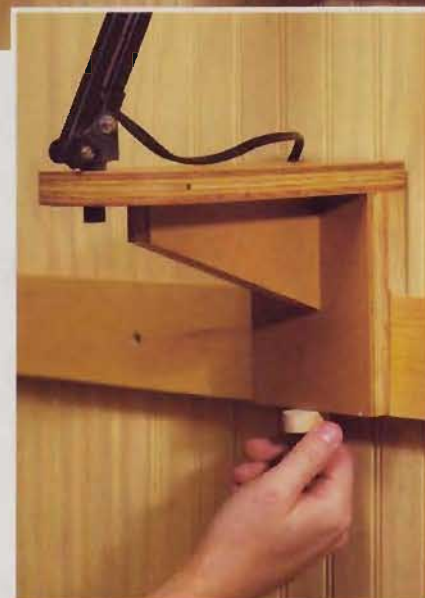
Rotate the turn button to secure the light support to the wall cleat.
