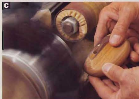
To fine tune the club head's contours, Russ relies on a flap sander. This process readies the head for final hand-sanding and finishing.
