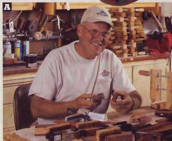
Russ Fisher epoxies a sole and face to a weighted block to create an oversize blank. He adds other pieces to create one of several different head shapes.
