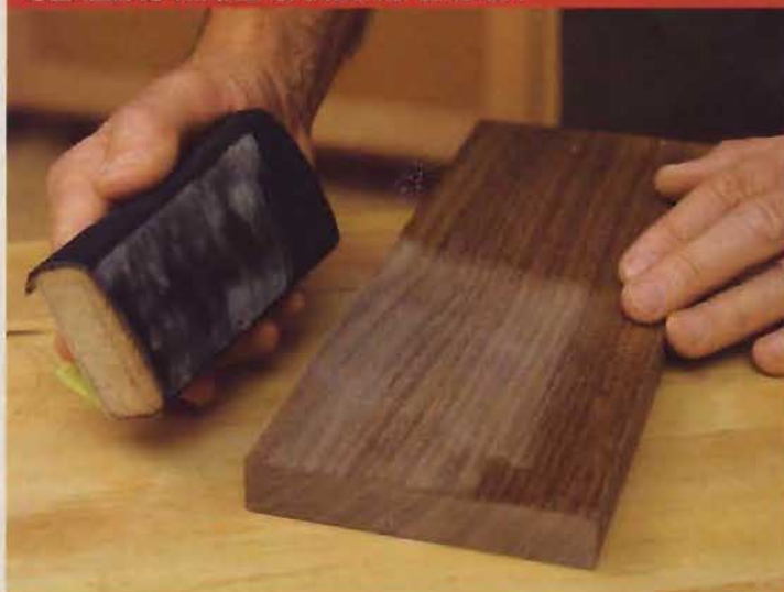
We brushed lacquer-based sanding sealer onto this walnut sample board and let it dry. Light sanding produced a powdery residue that didn't clog the 320-grit sandpaper.
