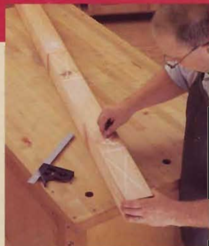
Look over your stock to find the clearest areas. Then, lay out the parts with chalk, as I'm doing here on a 4x4 post for the bench legs (A).
