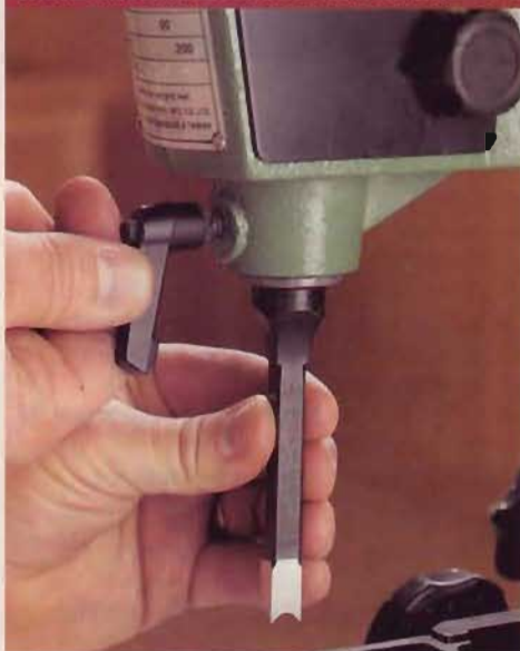
General International's handy ratcheting lock secures the chisel. The rest of the mortisers require a wrench or screwdriver.
