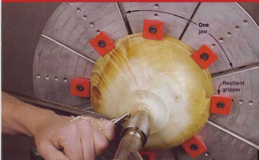
Although each manufacturer has a different name for this chuck accessory, adjustable bowl jaws all work the same. Resilient grippers hold the bowl rim to the chuck jaws. Sets cost from $50 to $140.
