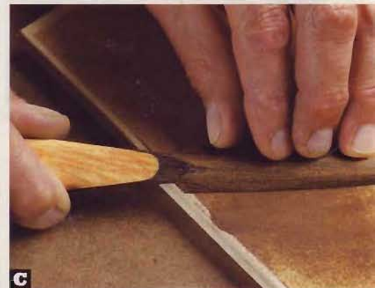
Adhere 100-grit sandpaper to a piece of plywood, and chamfer both blade edges.
