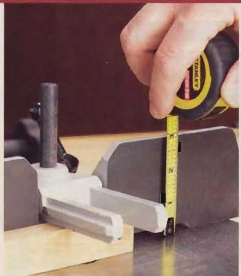
BETTER: Delta's fence stands nearly 3" tall for extra support, yet the stock hold-down works with material as narrow as 1".
