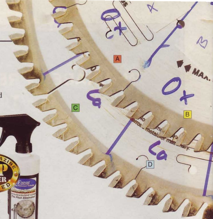
These two blades demonstrate grades A through D on the chart. An F grade indicates that the cleaner had no apparent effect on the blade grime.
