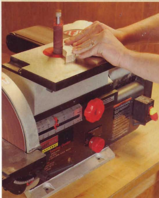
The oscillating spindle sander on the Craftsman 21516 has a \frac{5}{8} " stroke and oscillates 60 times per minute.
