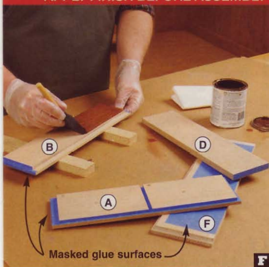
Covering the mating glue surfaces with masking tape, apply stain and then a clear finish to all the parts and assemblies. When the finish dries, remove the tape.
