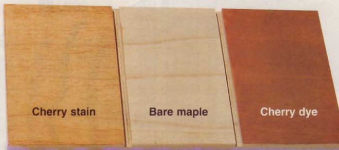
Maple has small, dense pores, so it doesn’t provide many places for stain pigment particles to lodge, as shown (left). A dye (right), colors the wood evenly, regardless of pore size.
