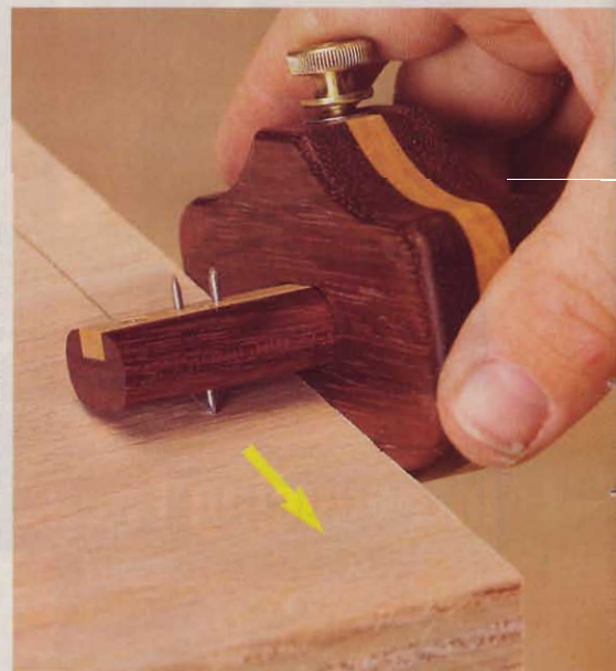
... or scribe plywood to prevent chipping when cutting rabbets.
