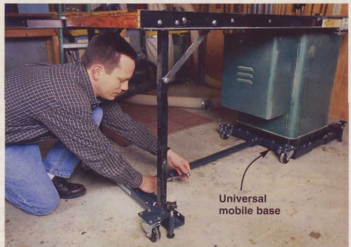
Techniques Editor Dave Stone adjusts the new mobile base that makes Jerry's massive tablesaw moveable.
