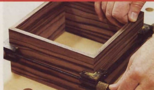
Step 4: After planing at the shooting board, recheck the joint. With just a few plane strokes, the joint fits tightly from top to bottom and creates a square corner.
