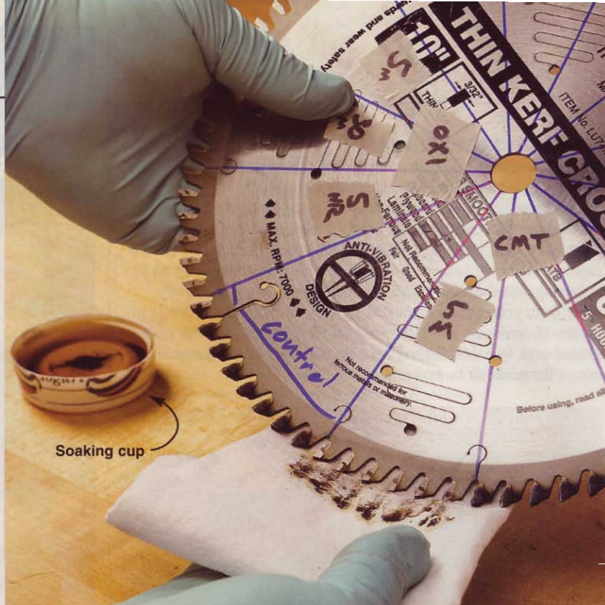
After soaking one set of teeth for five minutes (5M) in CMT 2050, most of the buildup wiped away easily. Note the dark deposits left in the soaking cup from the action of the cleaner alone. The “control” section shows the condition of the uncleaned teeth.
