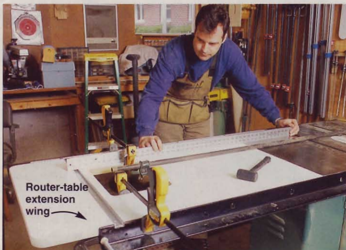
An integrated router table makes the tablesaw multi-task. Senior Design Editor Kevin Boyle makes sure it sits flush with the saw table.
