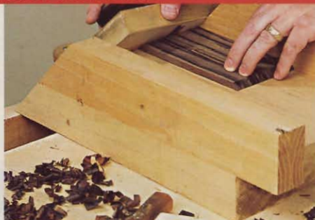
Step 3: Randy's shooting board consists of a piece of 8/4 oak with side fences. One end is cut at 45°. Placing paper shims under the workpiece allows fine angle adjustment.
