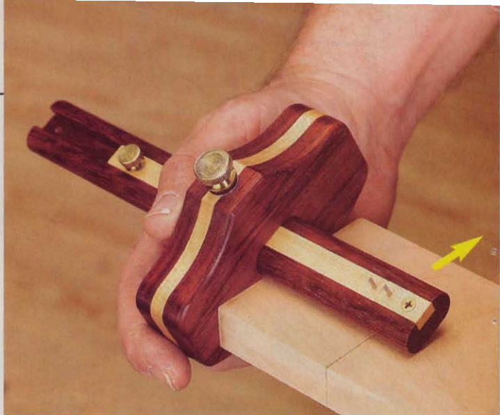
Use the single point to scribe the shoulders of a tenon...
