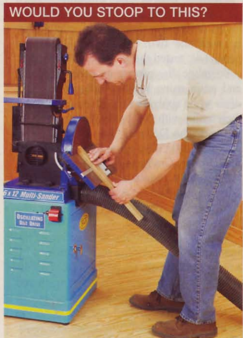
The low tables on the Craftsman/Fisch sander can test your back, especially when tilted down for sanding miters.
