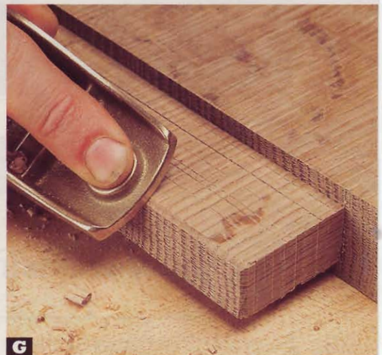
G Using a block plane or sanding block, chamfer the edges of a tenon so it slides easily into the mortise during the glue-up.
