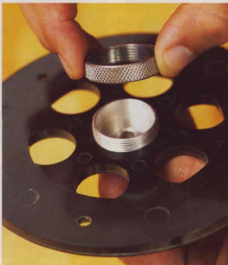
Two-piece guide bushings easily attach to your router's base.
