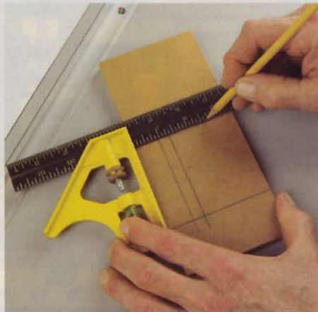
1 LAY OUT THE SLOT Draw slot boundary lines on the part, extending the end lines to the edges.
