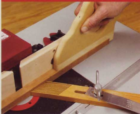
With the aid of a feather board, Carol Reed's pushstick for narrow stock keeps workpieces flat against the router table.
