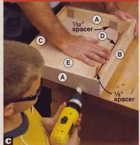
C Flip the case. Holding the lid (E) in place and positioned by spacers, drill holes through the side into the lid for the brass hinge pins.
