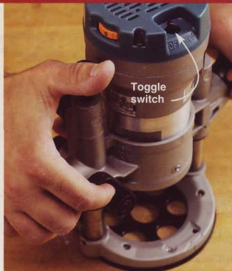
You can't reach the top-mounted toggle switch on the Makita without removing one hand from a handle.
