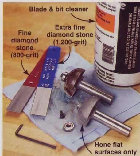
Remove pitch to keep bits cool. Diamond lapping stones (about $7 each) keep a keen edge between professional sharpenings.
