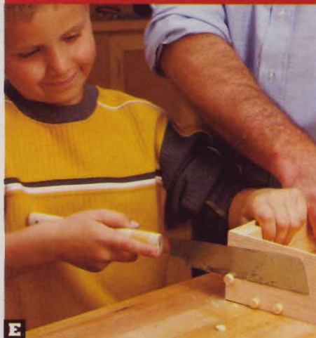
Trim the plugs flush with the sides (A) using a flush-trim saw. Keep the saw blade flat against the sides to ensure a straight cut.
