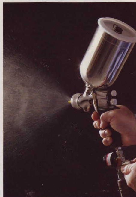
When using an HVLP sprayer, you'll get the best results by adjusting the incoming air pressure to the minimum setting that still fully atomizes the finish. An in-line pressure valve simplifies this process.
