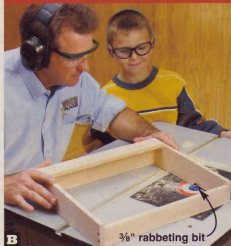
B With the rabbeting bit's bearing riding along the inside of the case, rout a \frac{3}{8} " rabbet \frac{1}{4} " deep around the bottom inside edges.
