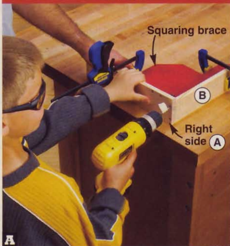
A Glue and clamp the right side (A) and back (B) together with a squaring brace. Then drill pilot holes through the side into the back.
