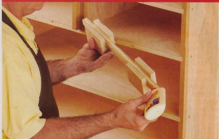
With the edge banding seated in the clamping guides, apply a centered bead of glue. To avoid squeeze-out, apply the glue sparingly.
