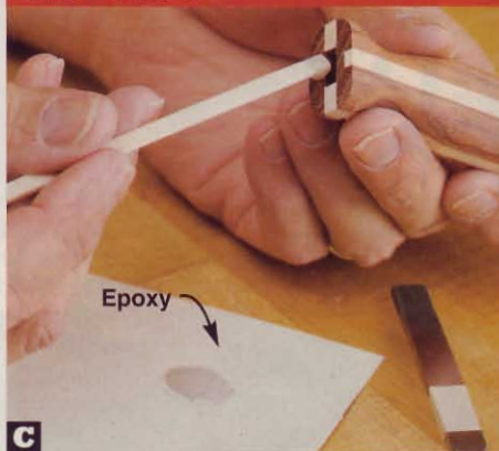
C Using a thin stick, apply a small amount of epoxy to the inside of the handle opening.
