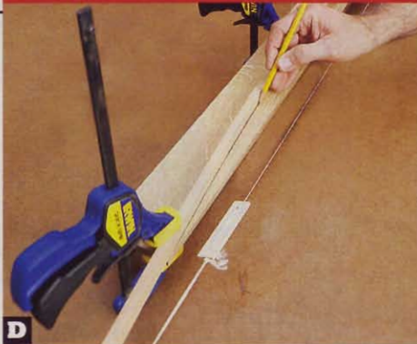
D A fairing stick is a flexible piece of wood that can be pulled into a curve to establish an arc.
