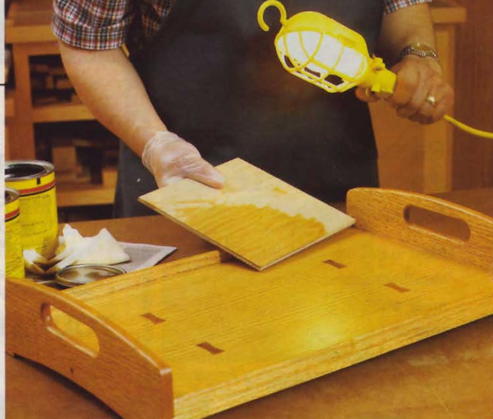
To color-match a tray that would normally be displayed beneath incandescent lights, we supplemented the fluorescent lights in our shop with an incandescent light.
