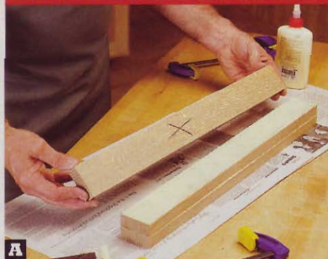
A Face gluing three 3/4"-thick pieces creates a 2 1/4"-thick blank for ripping the stiles
