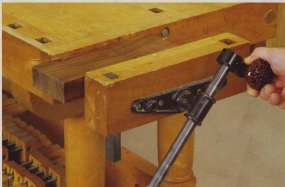
Twirling a steering wheel spinner opens and closes your bench vise quickly when it doesn't have a quick-release mechanism.
