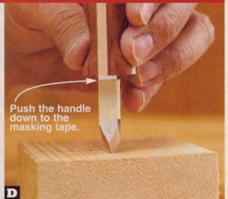
D With the blade point bearing on a scrap block, push the handle down to the masking tape.
