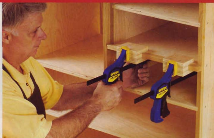
Clamp the edge banding in place. To give the far clamp jaw a surface to bear on, apply the edge bands with the case back off.
