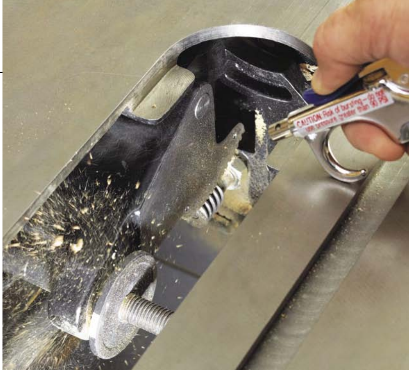
After vacuuming most of the dust, blast compressed air into the saw cabinet to dislodge the remaining deposits.
