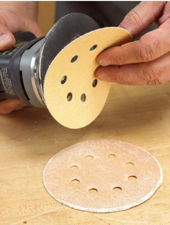
Wearing down a sanding disc to the cloth or paper backing costs you hours to save pennies. If you can't see or feel the grit working, change discs and toss out the old one.
