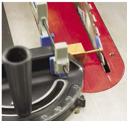
Check for equal contact against the brass screw at both the front (as shown at left) and rear positions (shown right) of the saw tooth that you've marked with masking tape.
