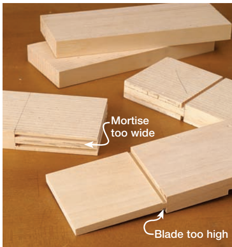
Scraps let you fine-tune fence and blade settings. Once set, make identical mortises and tenons on each frame workpiece.
