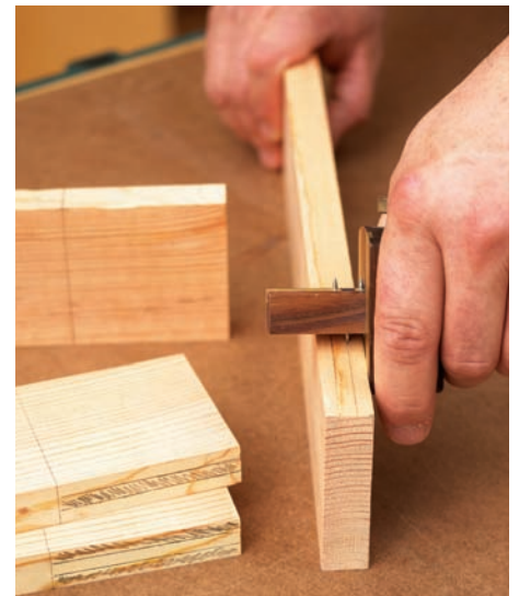
Mark all four sides of both ends on each piece. Then lay out and shade the waste areas to be removed.
