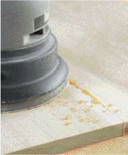
Glue globbs can scratch the surface of your work either when they break loose or become trapped on your sanding pad.
