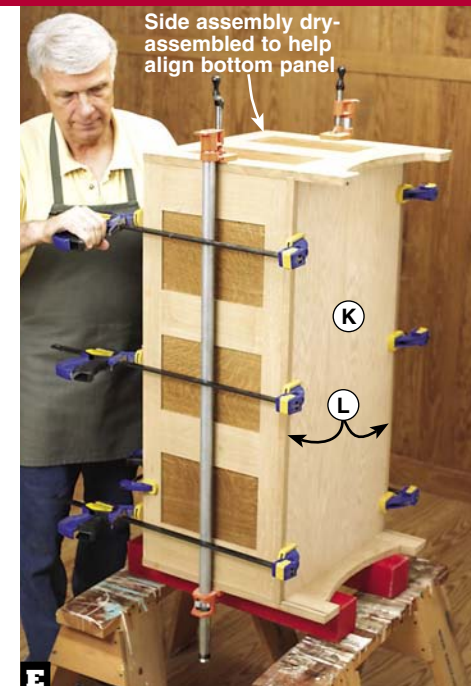
Clamp the bottom panel (K/L) to the case assembly, adding the remaining side assembly (no glue) to aid alignment.
