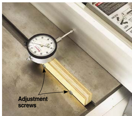
A dial indicator screwed to a shop-made block helps you check that the rip fence is parallel to the miter-gauge slot.
