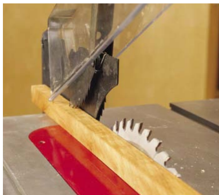
Use a straight piece of wood to check that the splitter is directly behind the blade so it doesn't interfere with the cut.
