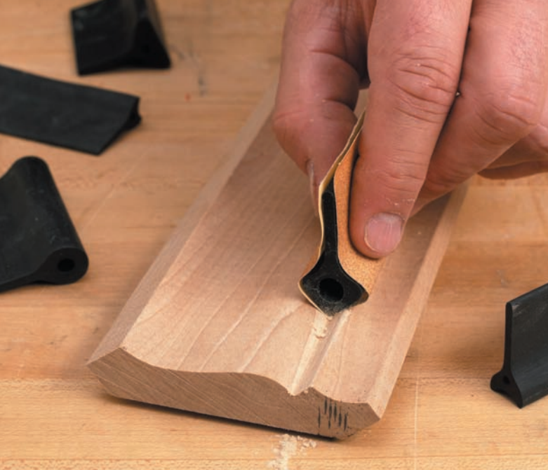
Contour pads allow you to divide complex profiles into sandable surfaces. These are from Lee Valley Tool (800/871-8158 or leevalley.com ; item #68Z82.10).
