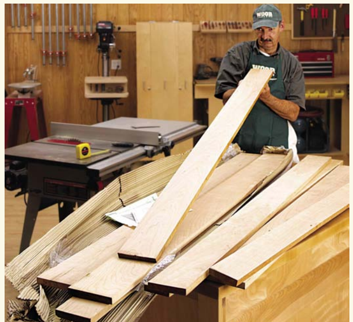
After unwrapping your hardwood, be sure to check each board for flatness and flaws.
