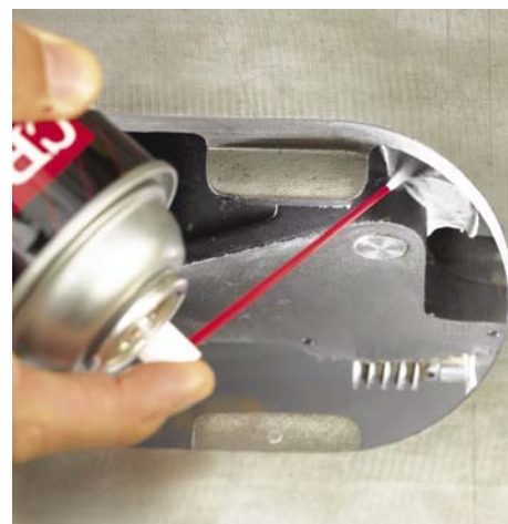
After vacuuming most of the dust, blast compressed air into the saw cabinet to dislodge the remaining deposits.
