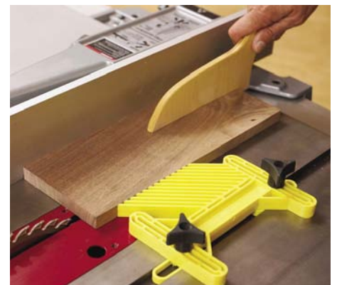
To rip stock successfully, keep it snug to the fence and saw table. Use a pushstick and feather board to help you do this.
