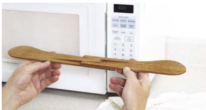
With the beveled face of each piece down, push the microwaved tongs together until they overlap approximately 5".
