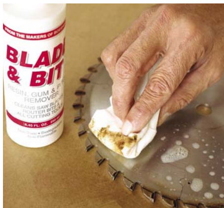
Working with a sharp saw blade, remove pitch buildup using a dedicated cleaner.
