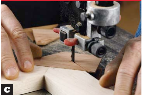
C Remove excess key stock with a bandsaw, then sand the face and edges flush using a random-orbit sander.
