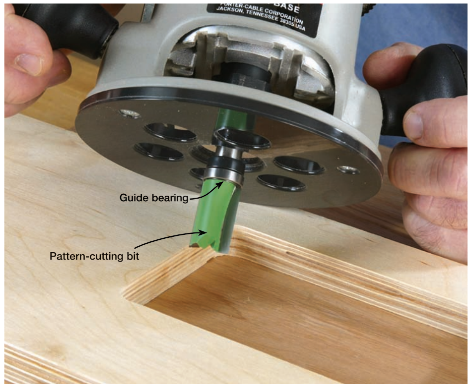
A pattern-cutting bit with a top-mounted bearing simplifies the sizing of templates. Rout counter-clockwise inside the pattern.
