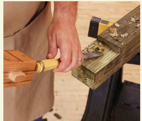
Step 3: Using a mallet and a chisel at least 1" wide, pare away the remaining material to smooth the rabbet. To avoid dig-ins, hold the chisel with the bevel facedown.
