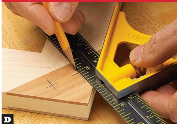
D Space the plugs an equal distance from the miter joint line. Plug locations can be adjusted to suit your key and frame sizes.
