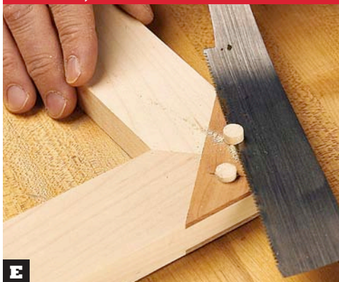
E When using a flush-cutting saw to remove plug stock above the key, cut parallel to the direction of the key grain.
