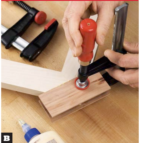
B These face keys have been planed to about \frac{1}{32} " thicker than the depth of the key rabbets in the frame stock.
