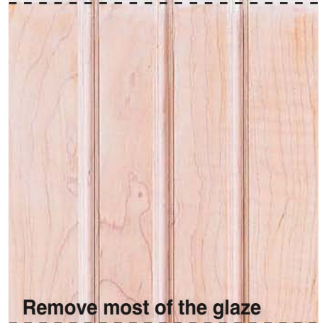
Apply glaze to the surface
