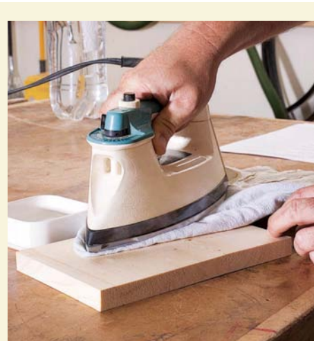
A household iron, a dampened towel, and sandpaper team up to help you make dents disappear.
