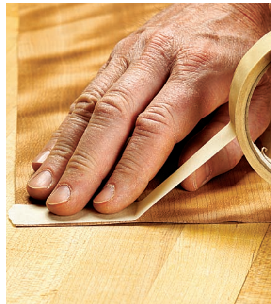
Delicate unbacked veneer tends to split along grain lines as it's handled, so apply tape to give the ends support.
