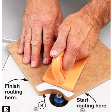
E Holding each bracket in the carrier board notch, rout the round-overs. Start and finish routing along the edge of the carrier.
