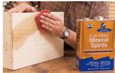
The best way to detect machine marks on a project is to rub it down with mineral spirits, using a clean, soft cloth.
