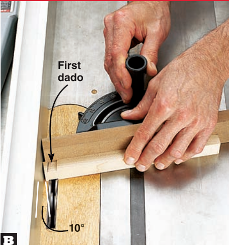
Angle the miter gauge 10° to the left. Turn the brace (A) blank over, and again with the corner touching the fence, cut the second dado.
