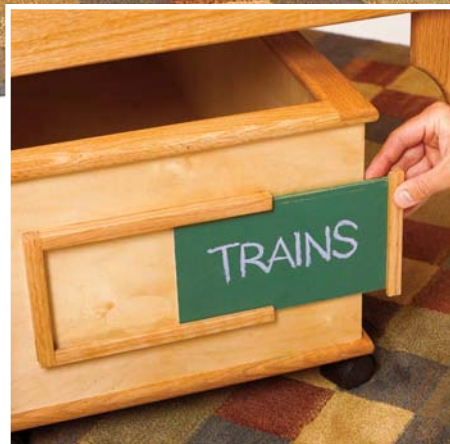
Slide-in hardboard panels painted with chalkboard paint make changing box labels easy.
