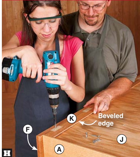
With a mounting cleat (K) tight against the top (F) and the bevel positioned as shown, drill mounting holes at the marked locations.
