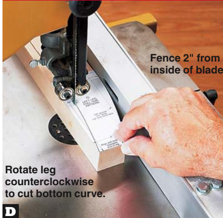
D Using the fence as a guide, bandsaw the outside edge of the left leg (G) to shape, rotating the leg, as shown, to cut the bottom curve. Fence 2" from inside of blade Rotate leg counterclockwise to cut bottom curve.
