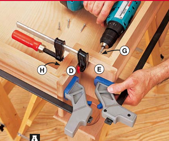
A Glue and clamp the cup holder sides (D, E) to the leg supports (G, H) with the tops flush. Drill pilot holes, and drive the screws.
