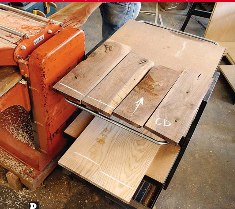
D Jeffry uses chalk lines to mark boards that plane without problems, arrows to remind him to reverse the feed direction on difficult-grained boards, and “gd” for boards that plane better against the grain.
