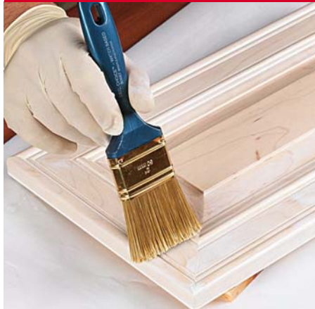
Apply glaze to the surface
