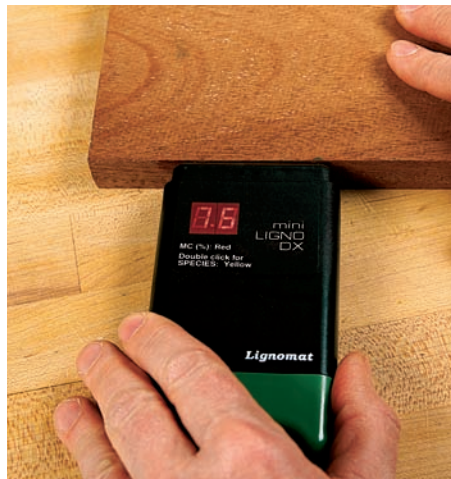
A moisture meter eliminates the guesswork about lumber condition. At 8.6 percent, this board is ready to use.
