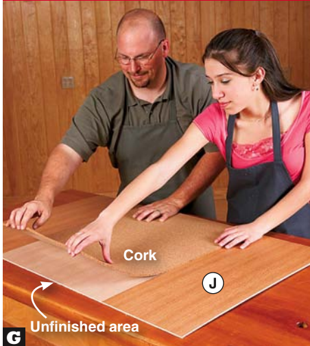
Holding the cork by the edges, align it with the bottom edge of the back (J) and the unfinished area. Then lay the cork in place.
