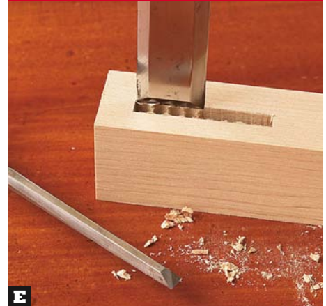
E Clean up the ends of the leg (L) mortises using a 1/4" chisel. Then pare the sides using a chisel at least 3/4" wide.
