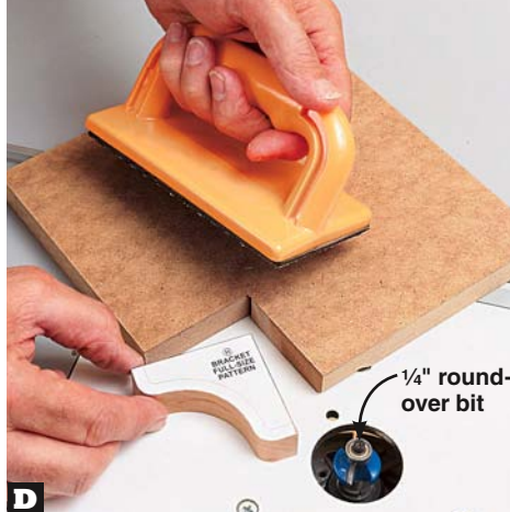
D To safely hold the brackets (K) while routing the round-overs, cut a 2½×2½" notch in an 8½×8½" piece of ¾"-thick stock.
