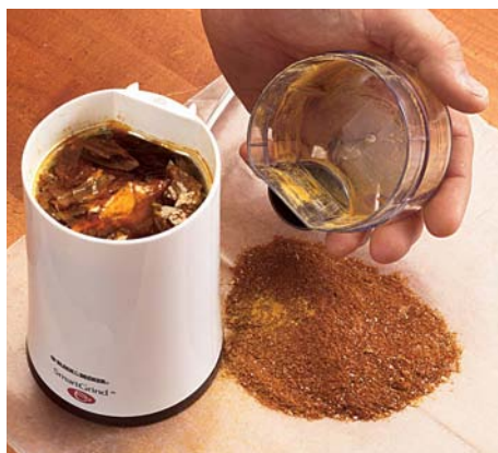
Breaking up shellac flakes in a blade-type coffee grinder helps them dissolve more quickly and evenly in alcohol.
