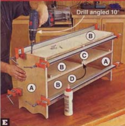
Glue and clamp the sides (A), panel/divider assembly (B/C/D), and bottom panel (B/D) together. Drill the mounting holes at 10^\circ .
