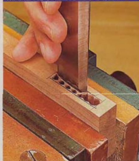
A sharp bench chisel shears off the waste left behind by the drill bit to flatten the walls of the mortise.
