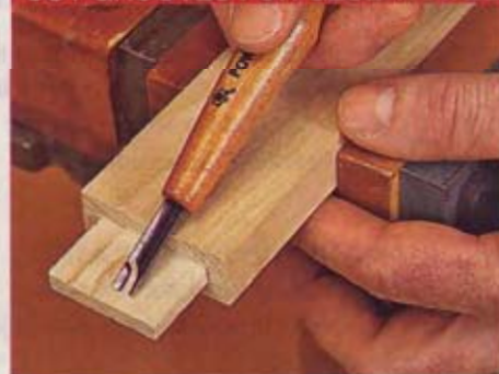
Using a carving tool or V-chisel, cut shallow grooves toward the end of the tenon to avoid an errant cut into the shoulder.
