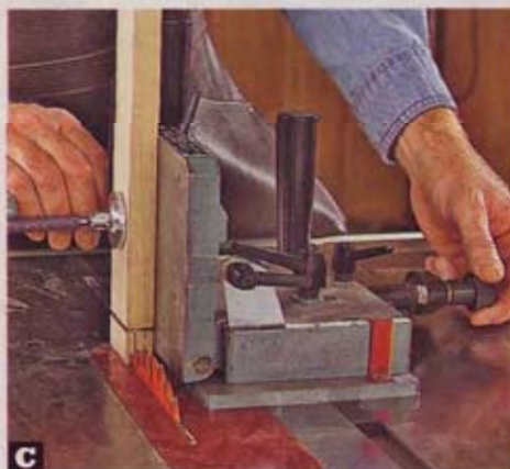
C Clamp your workpiece in the jig and line up the outside cheek. Use the fine adjustment knob (far right) to align the mark with the blade.
