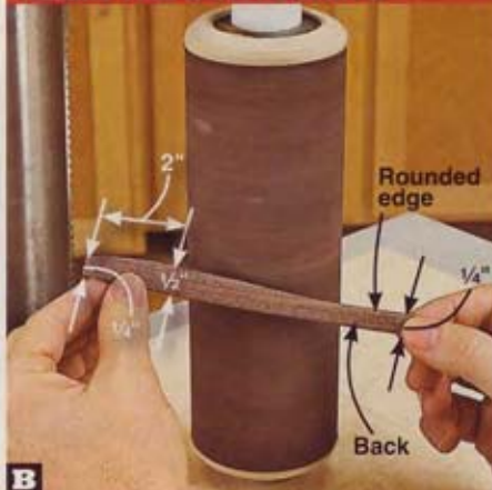
B Taper the top feather of the right wing from a thickness of \frac{1}{2} ", 2" from the left end, to \frac{1}{4} " at each end. Round over the front edge.
