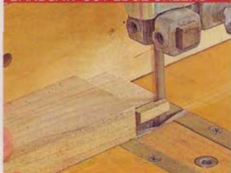
Set the fence to cut the farthest edge, avoiding pinching the cut-off piece. Be careful not to cut into the shoulders—or your fingers.
