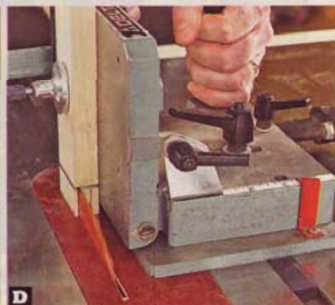
D Cut cheeks so scrap falls away from the blade, avoiding kickback. After making a cut, pull the jig back through the blade rather than lifting it.
