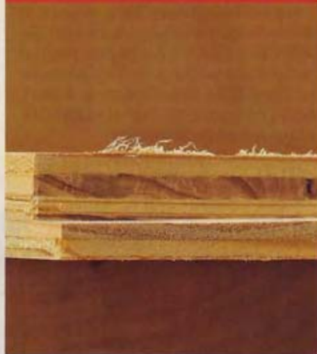
Rabbeting bits lift veneer when cutting rather than shear it cleanly ( left ), so we rely on a sanding block to remove the stringy fibers ( right ). If any fibers bend into the rabbet, simply use your sanding block to sand the vertical face of the cut. Take care to not round the edge.
