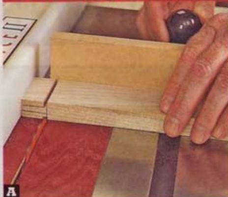
A Cutting the shoulders first results in crisp edges. Use the rip fence as a stopblock and a miter-gauge extension to prevent tear-out.
