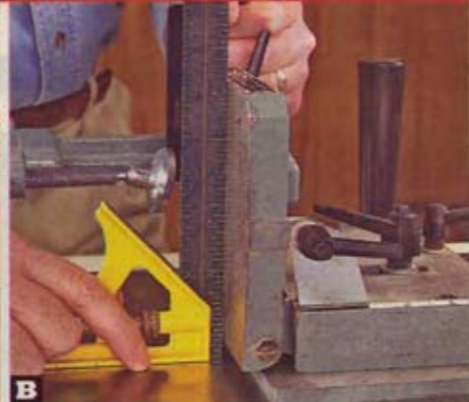
B Adjust the jig square to the table and parallel to the blade, so your tenons will be square and perfectly match your mortises.
