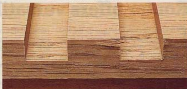
We cut these \frac{3}{4} " dados in red oak with a scrap board to back up the cut ( left ) and then without ( right ). The backer board eliminates tear-out.
