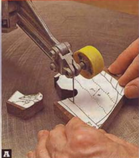
A Using a #2 reverse-tooth blade to minimize bottom tear-out, scrollsaw the parts to shape, cutting along the center of each line.
