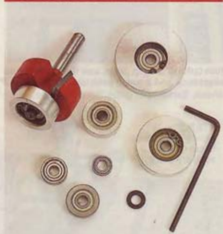
This set cuts rabbets to different widths with one bit. Smaller bearings produce wide rabbets, and larger bearings shallow.
