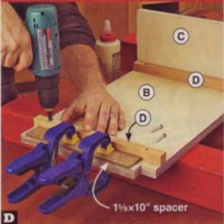
Using a spacer to position the drawer guides (D), glue and screw the guides 1\frac{1}{8} " from the ends of the middle and bottom panels (B).
