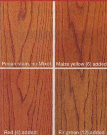
Starting with straight Varathane pecan stain (upper left), we added 1 teaspoon of Mixol in various colors to half-cups of stain to change its tint.
