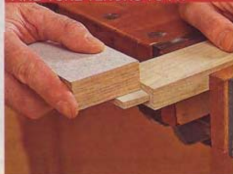
Use a sanding block to reduce the tenon's thickness. Keep the block square to the cheek and shoulder to avoid tapering the tenon.
