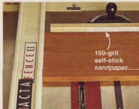
When cutting across grain, use the rip fence as a stopblock and a wood extension to reduce tear-out. Sandpaper grips the workpiece.
