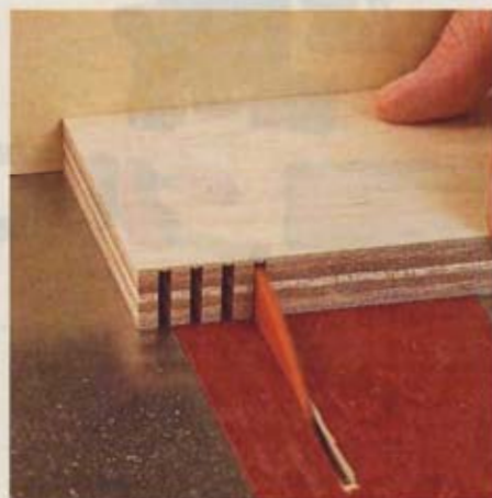
Dropping each successive saw kerf over the pin, kerf the entire length of the workpiece.
