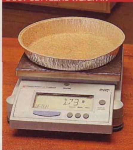
We weighed the dust that settled out of the air using a microbalance—a supersensitive scale accurate to 0.01 of a gram.
