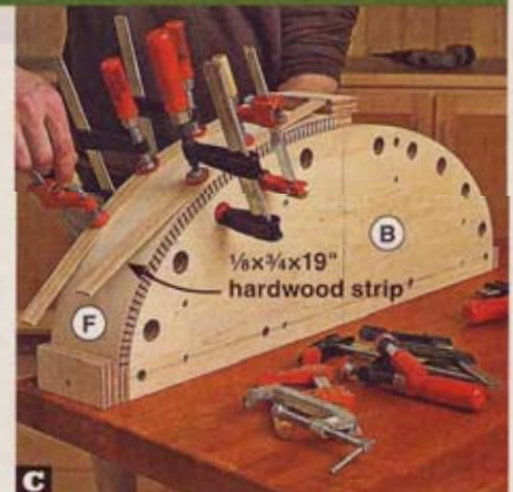
C Using hardwood strips to distribute clamp pressure and working from the center to the ends, clamp the aprons (F) in place.
