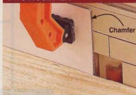
Sand a slight chamfer on the end of the laminate nearest the bit so the workpiece won't catch as you feed it through.
