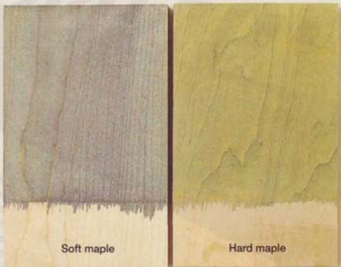
Ferrous sulfate solution applied to these sample boards turns the soft maple (left) a blue-black, and the hard maple greenish gray.
