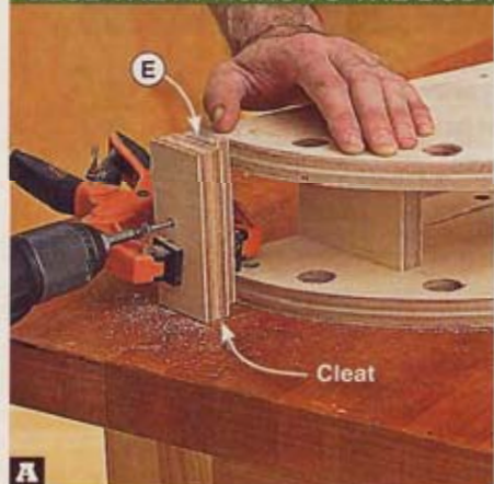
A With the cleat overhanging the leg spacer (E), drill a pilot hole into the spacer and screw the cleat in place.
