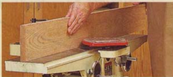
Rely on your jointer to machine a straight, square edge on a relatively straight board in just a pass or two.
