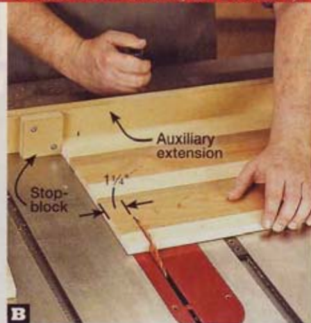
B Using a stopblock attached to an auxiliary extension on your tablesaw miter gauge, crosscut 1 1/4"-wide strips from the blank.
