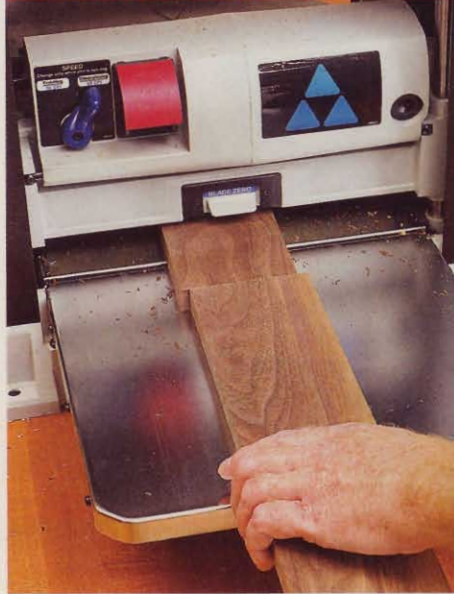
Planing boards end to end keeps the feed rollers at a consistent height, taking away the chance for snipe.
