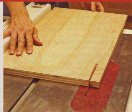
RIP WIDTH GREATER THAN 6": Hold the workpiece tight against the fence, and feed it through the blade with your right hand. Use your left hand to guide the piece.
