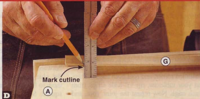
D With the free end of the cove (G) overlapping the other leg (A), place a ruler against the leg and mark a cutline on the cove.
