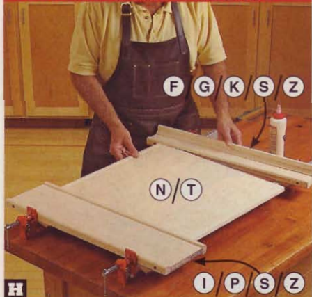
H Squeeze glue into the end lower rail (I/P/S/Z) and end upper rail (F/G/K/S/Z) grooves, and clamp the panel (N/T) in place.
