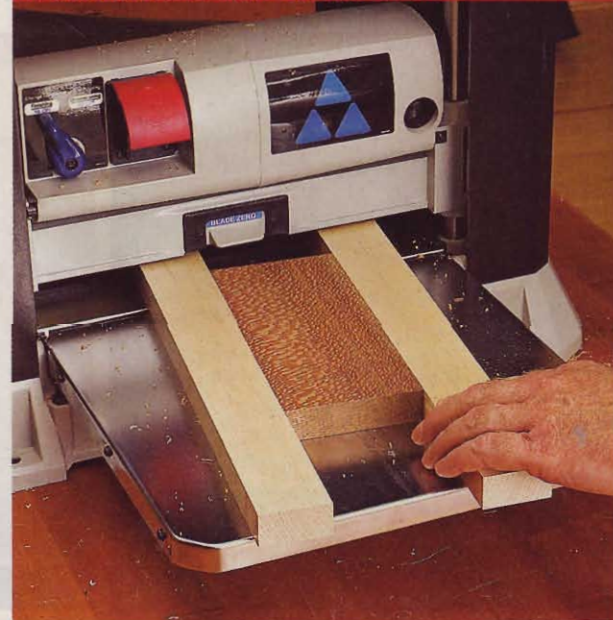
Scrapwood runners help you get use from cutoffs, like this 8" piece of leopardwood.
