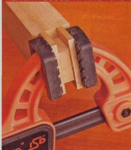
Sand one side of each patch, and then glue and clamp it to the tenon. Make sure the patch's grain orientation matches the tenon's.
