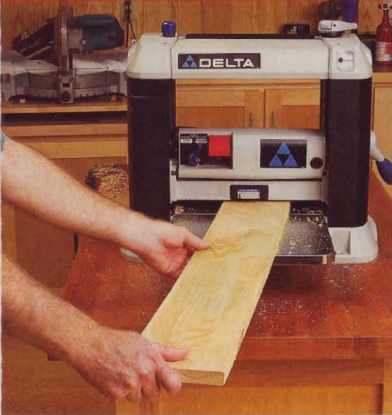
Feeding boards at a slight angle not only reduces surface chip-out, but also helps limit any snipe to one corner.
