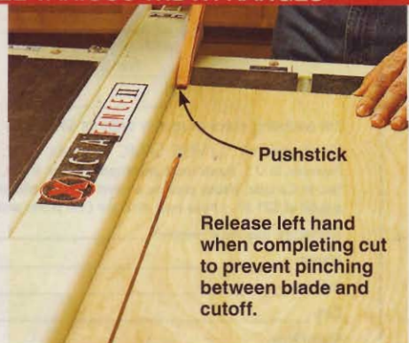
RIP WIDTH BETWEEN 2" AND 6": Feed the workpiece through the blade using a pushstick in your right hand. Again, use your left hand as a guide.
