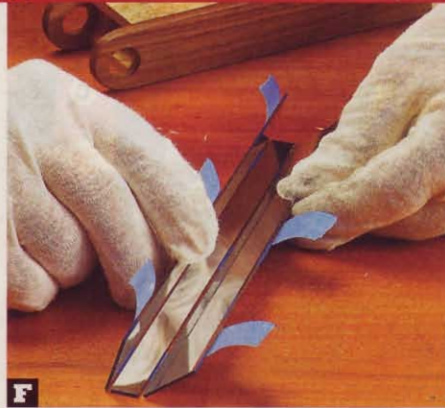
F Flank the narrow mirror with the wide ones, leaving \frac{1}{8} " gaps. Remove the film, and fold the mirrors into a triangle.
