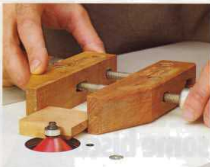
A wooden handscrew clamp serves as a safe extension of your hands, gripping the small part firmly while sitting flat on the table surface as you rout its edges.
