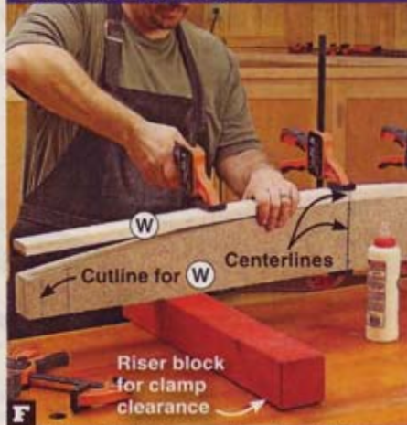
F With the glued strips centered on the form, clamp them in place, working from the center to the ends, keeping the edges flush.
