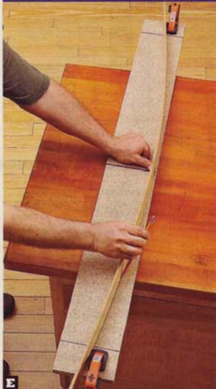
E With the curve center- and endpoints marked on a form piece, bend a fairing stick to connect the points and draw the curve.
