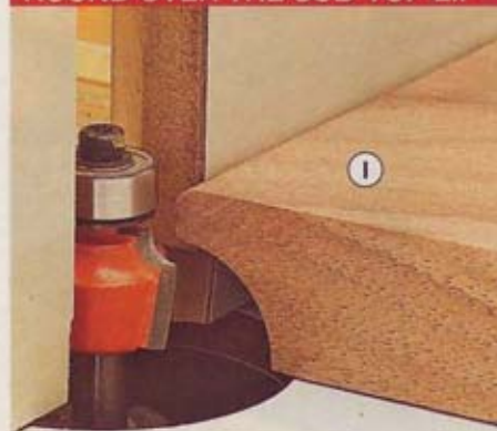
B Using a \frac{1}{8} " round-over bit, rout along the ends and then front edge on the bottom of the sub-top (I) coved lip.
