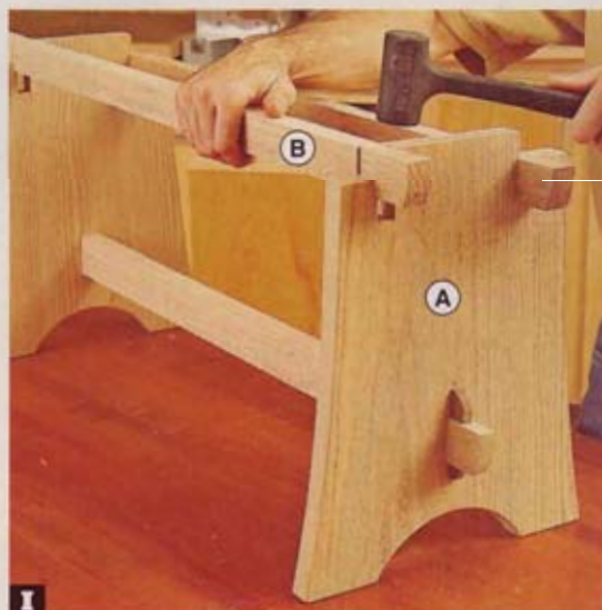
I Spread glue in the upper stretcher (B) dadoes, and tap the stretchers into the notches in the legs (A).
