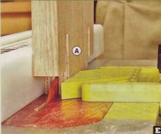
Cut a centered \frac{1}{8} " groove \frac{3}{4} " deep in the tenon at the top of each leg (A) to receive the wedge (E).
