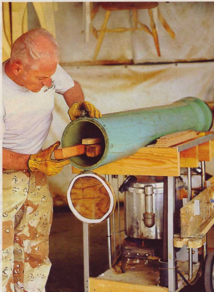
Opposite page: Russ inserts one end of workpiece into a hold-down built into one end of a form and secures it with a wooden wedge. Above: The steam chamber, water tank, heat source, and form holder ride on a cart for easy setup and storage.
