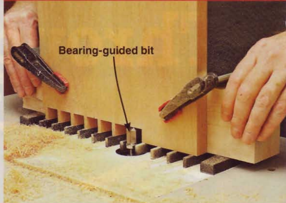
Visibility of the cutter improves and the chips blow away from you when routing tails and pins on a router table.
