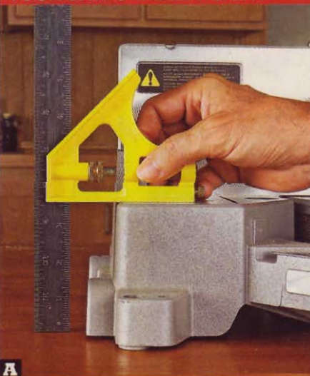
A Using a combination square, measure from a flat surface to your miter saw table to find the width of the platform rests/handles (B).
