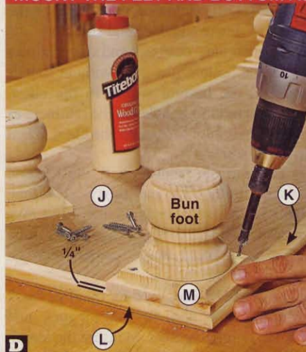
D Glue each foot support (M) assembly to the bottom panel (J/K/L). Drill mounting holes angled at 10^\circ , and drive the screws.
