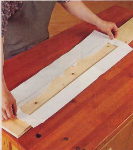
Paper windows let you rough out the position of cuts for a balanced pattern.
