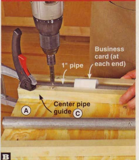
B With a business card bent around a 1" pipe at each end for a spacer, mount the center pipe guides (C) to the bottom platform (A).
