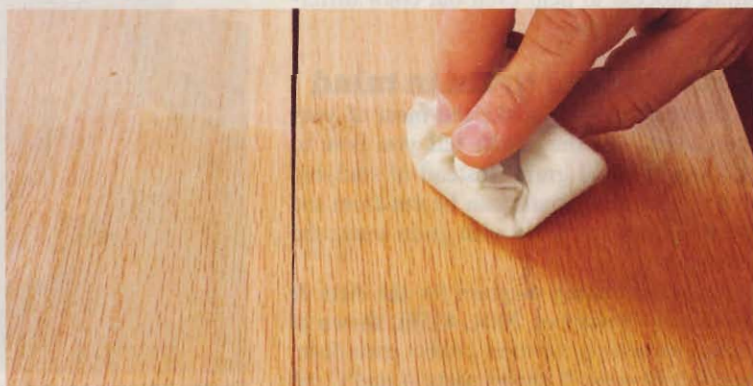
A moist cloth reveals grain and color as it will appear after finish is applied.
