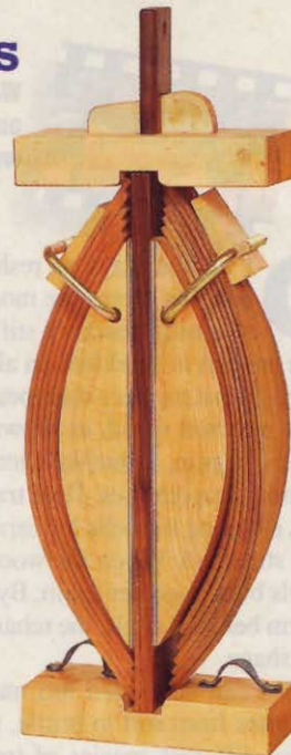
The top form makes compound curves using a mix of screw-down brackets and straps plus a compression strap. The right end of the form holds the compression strap handle in place. The lower form creates a simple curve, using two U-bolts and wedges. The maple and walnut slat form at right is modeled after one used in the middle to late 1700s.
