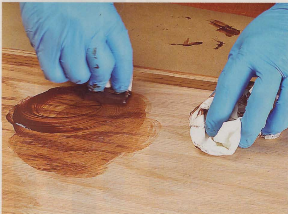
Apply stain with a circular motion to work pigments into the pores. Then wipe with the grain and remove any surplus.
