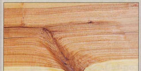
Dogwood Cornus florida Found: All over This hard wood gets smoother with use, making it perfect for mallets and handles.
