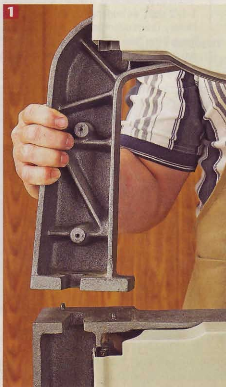
1 Remove the bolt that holds the saw arm to the base. The arm simply lifts off, but be prepared—it's heavy and awkward.
