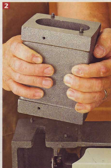
2 The typical riser block includes indexing holes on the bottom and matching pins on the top, so it's self-aligning. If your riser block has no pins, align the outer edges flush with the base. Reinstall the saw arm, as shown in the photo at the top of the page.
