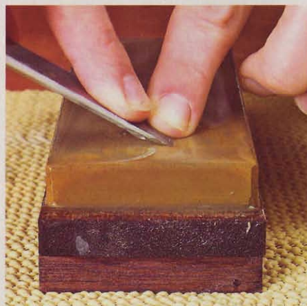
Stones are designed to work only with water to create a slurry for honing.
