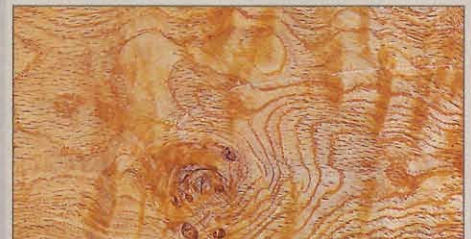
Bur Oak Quercus macrocarpa Found: All over A dead ringer for white oak; you'll want to sand or scrape the wild grain to avoid tear-out. This sample shows curly figure.
