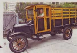
Chuck spent 100+ hours restoring the wooden cab, box, and wheel spokes of his 1923 Model TT truck.
