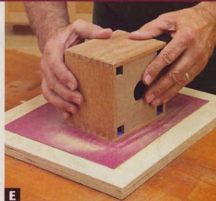
E To prevent rounding of the corners and edges, adhere sandpaper to a flat surface, and finish-sand the outsides of the boxes.
