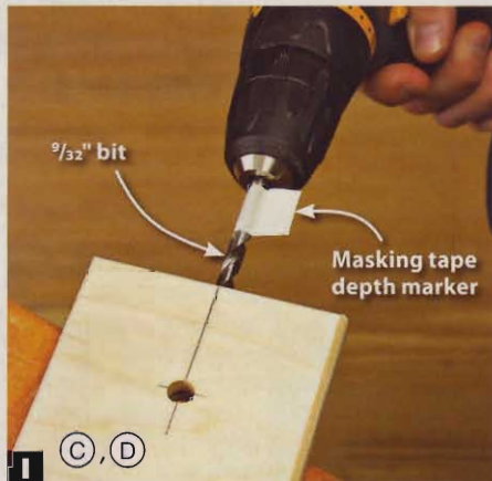
I After removing the dowel jig, chuck a \frac{3}{32} " bit into a handheld drill, enlarge the \frac{1}{4} " hole, and extend it to a depth of 3".
