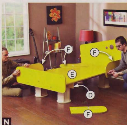
N Fasten the sides (F) to the stretcher (D) ends and panel (E) edges with cross dowels and connector bolts.
