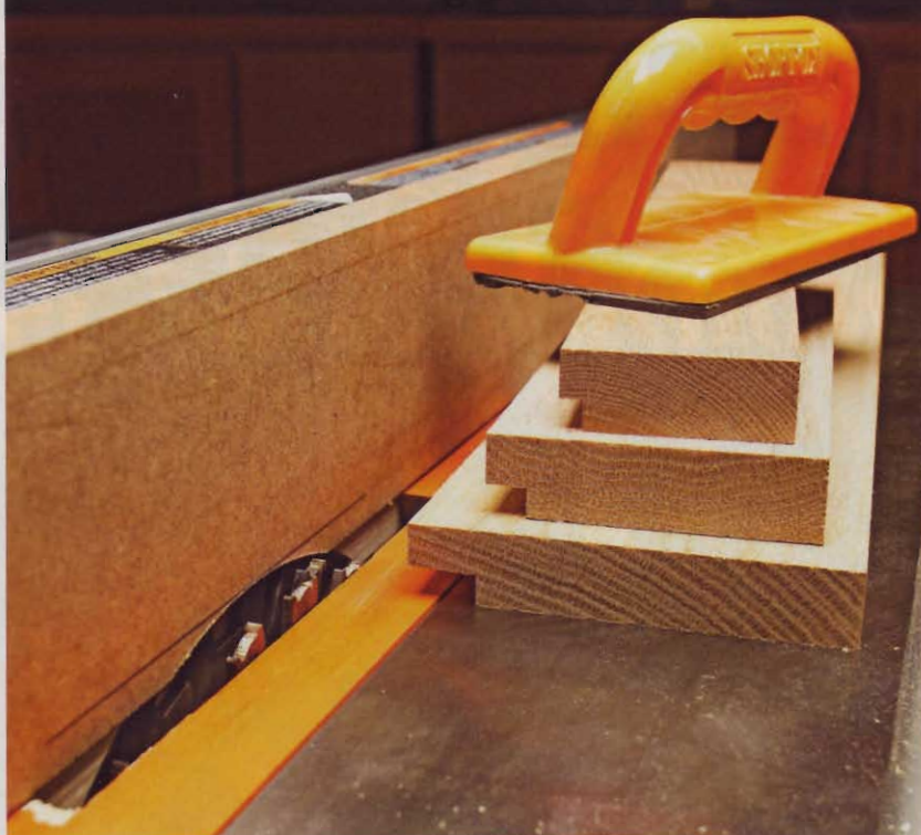
These three \frac{5}{16} "-deep rabbets were cut in three different widths with a \frac{3}{4} " dado blade. Housing the blade in an auxiliary fence makes it easy.
