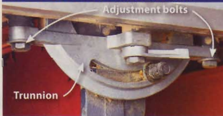
The small forged-steel trunnions on this saw secure to the top rather than the base, making top-to-blade alignments trickier.
