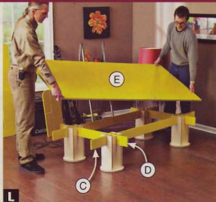
L Place the panel (E) onto the base (A/B/C/D), aligning the edges of the panel with the ends of the stretchers (C, D).
