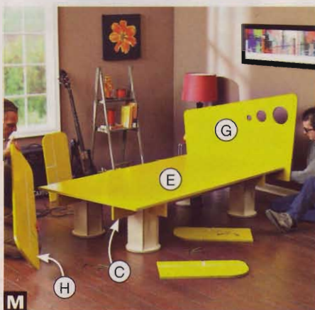
M Fasten the headboard (G) and footboard (H) to the stretcher (C) and panel (E) ends with cross dowels and connector bolts.
