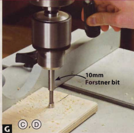
G After marking the cross-dowel hole center with an awl, drill the hole on the drill press with a 10mm Forstner bit.
