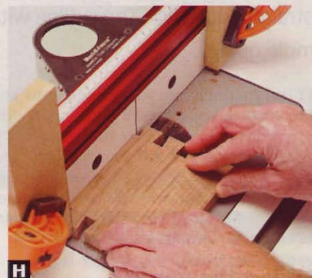
H Move the workpiece from right to left on a router table. Rout it the opposite way, and the router could yank it from your grip.
