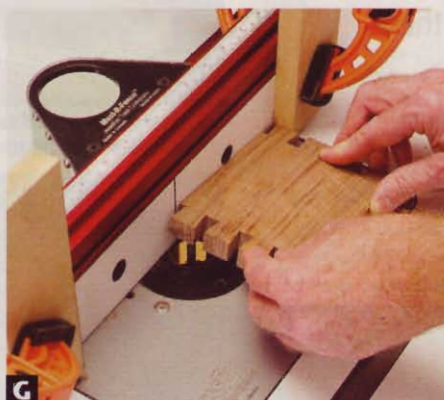
G Wiggle the workpiece right and left slightly—keeping it trapped against the fence—as you lower it onto the spinning bit.
