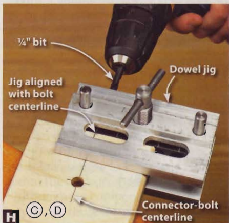
H Using a dowel jig to center a \frac{1}{4} " bit on the plywood edge and align it with the centerline, drill a hole as deep as the bit allows.
