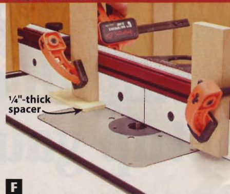
F Use a spacer to elevate the stopblocks, allowing debris to pass underneath. Remove the spacer before routing.
