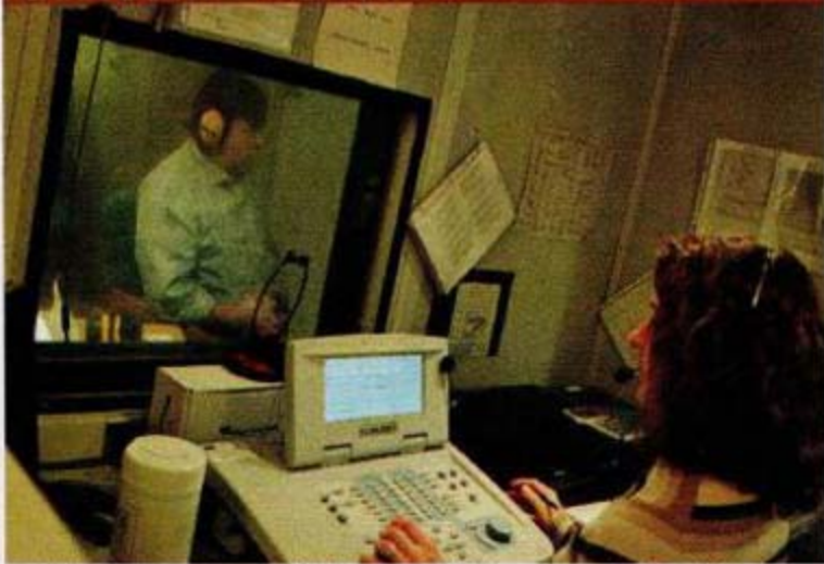
Audiologist Stephanie Fleckenstein delivers sound signals in different frequencies to Matt Seiler to test a pair of hearing muffs.
