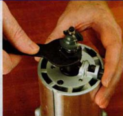
With one-wrench changes, you hold the motor as well as the spindle lock and wrench.
