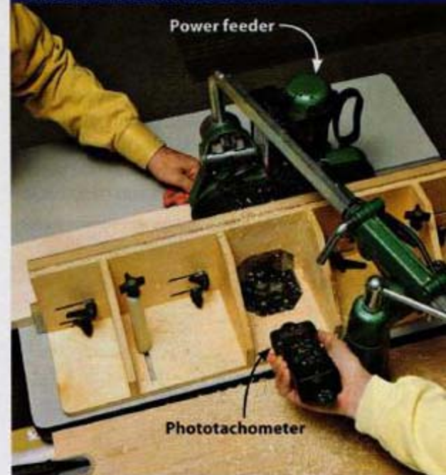
We measured spindle speed with a phototachometer as each router machined a profile in \frac{3}{4} "-thick hard maple.
