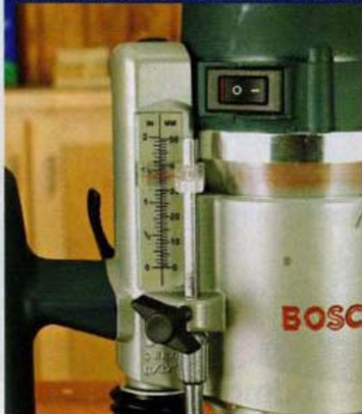
The depth scale on the Bosch 1617EVSPK is easy to see when setting plunge depth.
