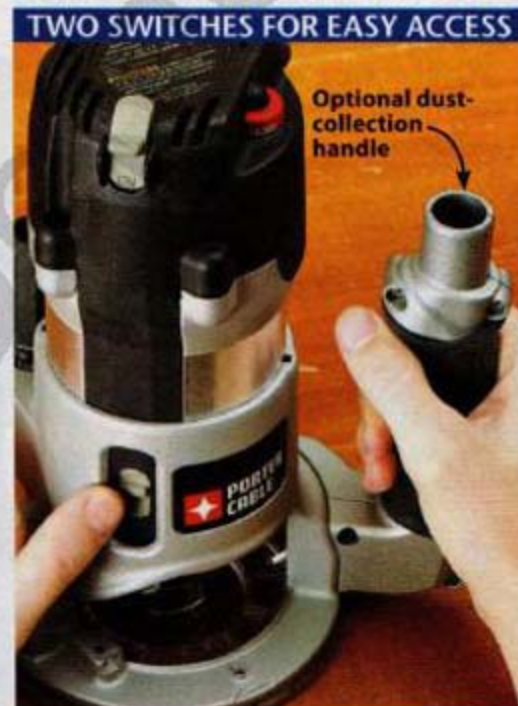
The pole-type switches on Porter-Cable's 895PK give you two options to power up and shut down.
