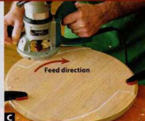
C Climb-cut the danger zones, holding the router firmly to guard against jerking.
