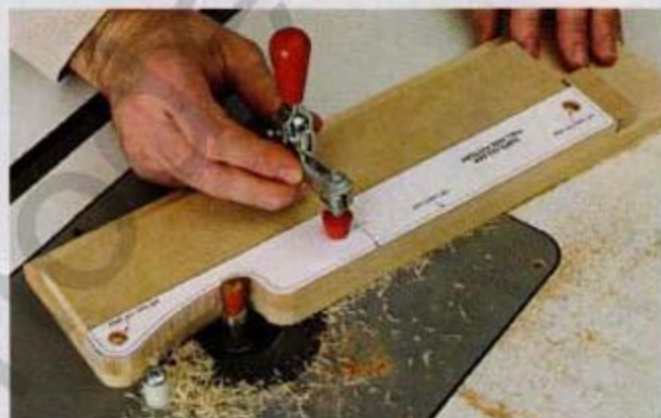
After bandsawing the knife-holder side to rough shape, clamp it into the template jig and flush-trim the piece to final shape at your router table.
