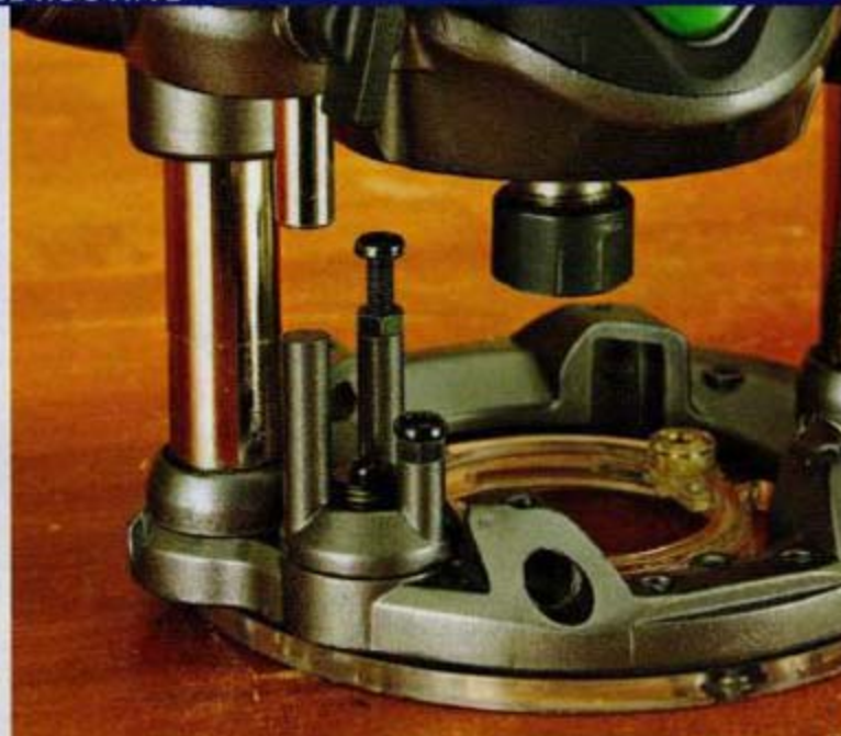
You adjust the screws on some turrets, like these two on the Hitachi, for microadjustments. The third stop is not adjustable.
