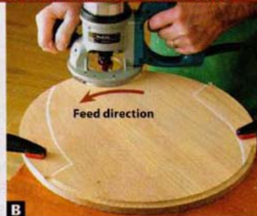
B Rout the areas unlikely to tear out before moving on to the danger zones.
