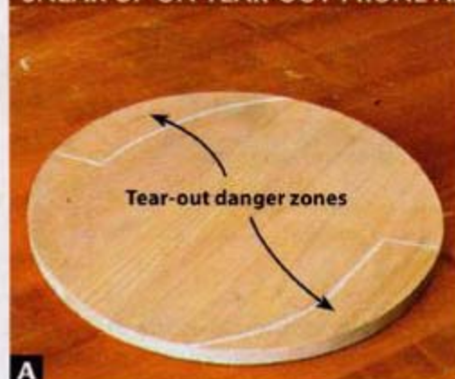
A Danger zones feature grain that parallels the edge and is prone to tear-out.
