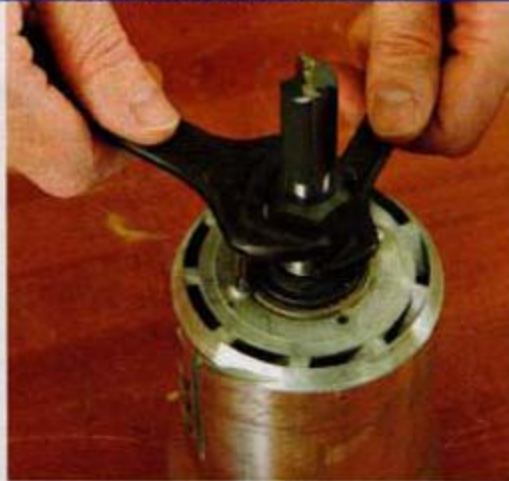
Two wrenches give you plenty of leverage to easily break loose the collet to change bits.
