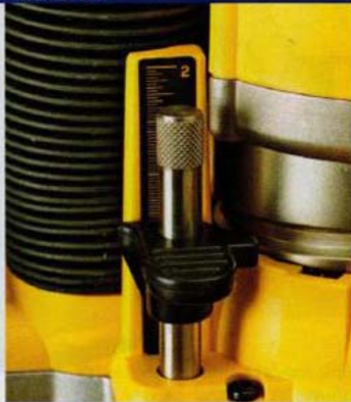
The scale markings on the DeWalt DW618PK are mostly blocked by the depth rod.
