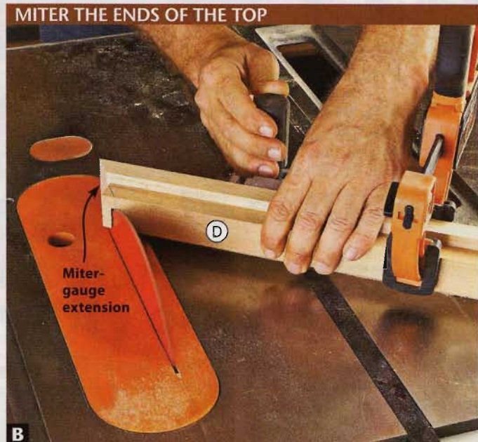
B Attach a long extension to your miter gauge and cut it off at the 37° angle to help you align the top (D) for cutting the miters.
