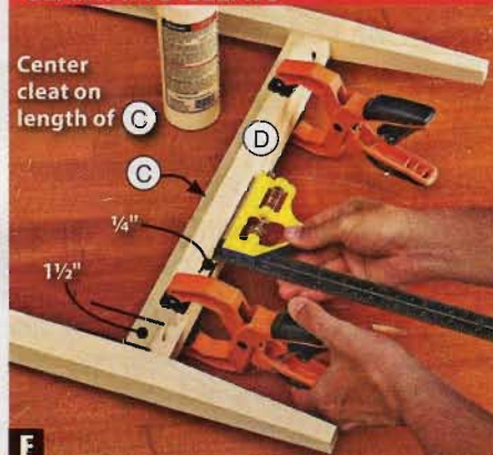
F Position the shelf support cleats (D) 1/4" from the bottom of the lower end rails (C) and centered on the length of the rails.
