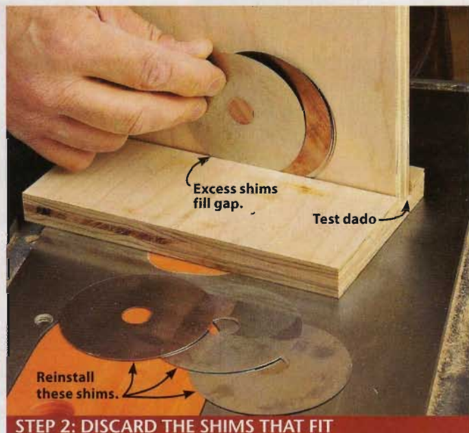
STEP 2: DISCARD THE SHIMS THAT FIT
