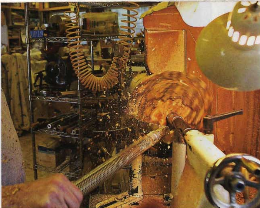
To maximize his resources, Doug uses an Easy-Core pivoting tool that allows him to salvage the waste wood inside a bowl and turn those pieces as well.
