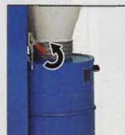
Step 1 Lift Drum Lever
