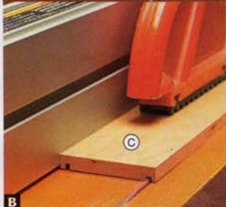
Blade kerfs in the top and bottom back edges of the top rail and top edge of the lower rail catch glue to control squeeze-out.
