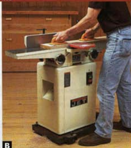
B Apply light pressure to keep the jointed portion in contact with the outfeed table. Move the piece forward with both hands.
