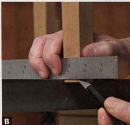
B With the other three legs down tight against the top of the tablesaw, set a straightedge on top of the saw. Then score a line on the leg along the bottom of the straightedge. Repeat on the opposite face.
