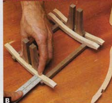
B Install both outer rests \frac{1}{4} " from the end of the feet.
