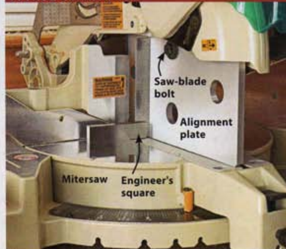
Mount a machined steel plate in place of a blade to check saw alignments. The plate is perfectly flat from one edge to the other.
