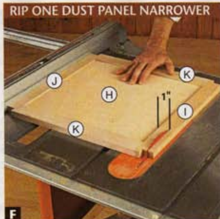
F For the shallow bottom dust panel (H/I/J/K), rip the front (cherry) rail (I) on one dust panel to 1" wide.
