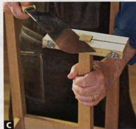
C For removing \frac{1}{16} " or more, clamp the cutting guide around the leg so its top aligns with the score lines on the leg. Hold a flush-cut saw flat against the top of the cutting guide and trim the leg along the score lines.
