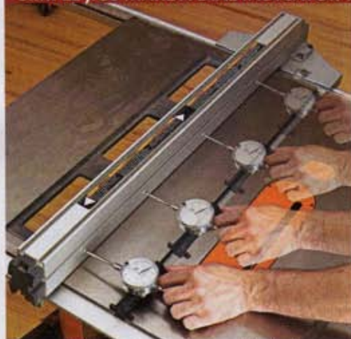
Secure a dial indicator to a jig that rides in the miter-gauge slot. Then slide it along the slot to check your rip fence for parallel.
