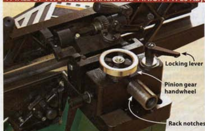
You turn a handwheel to move a rack-and-pinion fence. Rikon's model also has a rack-and-pinion adjustment for tilting the fence.
