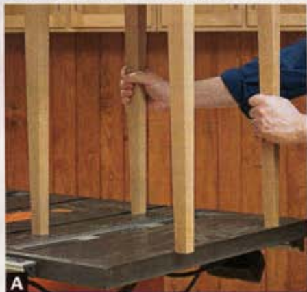
A After determining which are the long legs, hang one over the edge of a reliably flat surface. (In most shops, a cast-iron tablesaw top or large shaper table fills the bill better than a wooden benchtop.)
