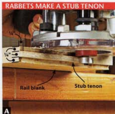
RABBETS MAKE A STUB TENON Clamp a rail blank to the bench. Rout a \frac{1}{4} \times \frac{1}{4} " rabbet along each face at both ends to create \frac{1}{4} "-thick stub tenons.
