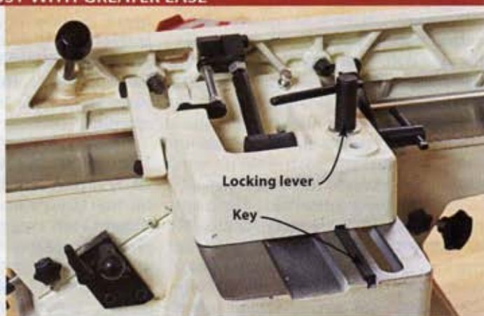
Jet's fence slides front to back manually, using a keyway slot to keep it aligned with the jointer bed.
