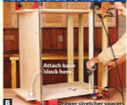
B Scrapwood spacers ensure consistent alignment while you install the stretchers with pocket-hole screws.
