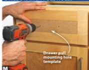
M A template ensures centered, precise holes for your drawer-pull hardware, no matter how many drawers you make.
