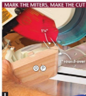
I Round the round-overs on the ends of the base pieces (O, P); then mark and cut the miters. The base ends are cut to finished length later.
