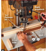
A With the center support (A/C) bottom edge against the fence and the rear end against the right stopblock, bore the front hole.
