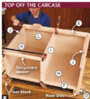
K Position the riser blocks to help align the top assembly with the rear stiles (D). A temporary spacer keeps the divider (I) from racking.
