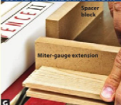
A spacer moves the fence away from the blade for cutting tenons.
