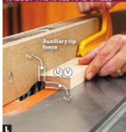
L House the dado blade in an auxiliary rip fence leaving \frac{1}{8} " exposed. Cut rabbets on the inside edge of each door rail (U) and stile (V).
