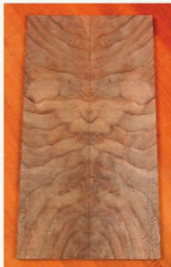
Open the resawn blank like a book. Align the grain pattern across the joint line, and glue the two halves together.
