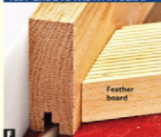
Set the fence position and blade height using scrap the thickness of your workpiece.
