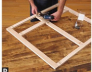
D Pocket screws eliminate the need for clamps as you assemble the frame. Screws won't show after you glue the frame to the cabinet.
