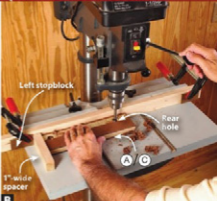
B Slide the center support (A/C) to the left, inserting a 1"-wide spacer between the part and stopblock. Bore the rear hole.
