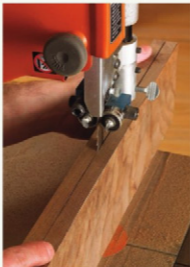
Mark a line down the center of one edge. Cut carefully to minimize cleanup of the sawn faces that could change the pattern match.
