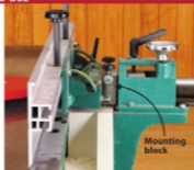
Grizzly's fence slides into a dovetailed block, secured by two locking bolts.
