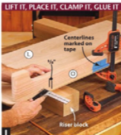
J Center the base front (O) on the length of the bottom assembly and inset \frac{1}{8} " from the front edge; then glue it in place.
