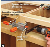
N Any clamps will hold cases together, but this clamp also holds the faces flush and provides a pilot-hole drilling guide.
