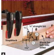
A Clamp a stopblock to the router-table fence 1\frac{1}{2} " from the left edge of the bit. Rout a \frac{1}{4} " groove in only one blank with this setup.
