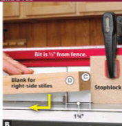
B Reposition the stopblock, and plunge the second blank onto the bit. The blanks end up as mirror images of each other.
