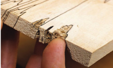
Random black lines make spalted wood attractive, but can leave soft zones unsuitable for cutting boards.
