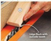
L House the dado blade in an auxiliary rip fence leaving \frac{1}{8} " exposed. Cut rabbets on the inside edge of each door rail (U) and stile (V).
