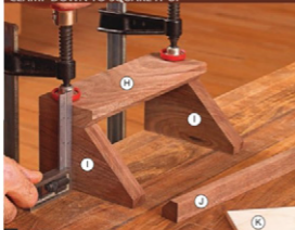
B When gluing the top (H) to the ring-holder sides (I), clamp the pieces to your bench. Check both sides for square to the benchtop.
