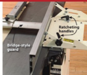
Jet's fence secures to the machine with two ratcheting-handled bolts.
