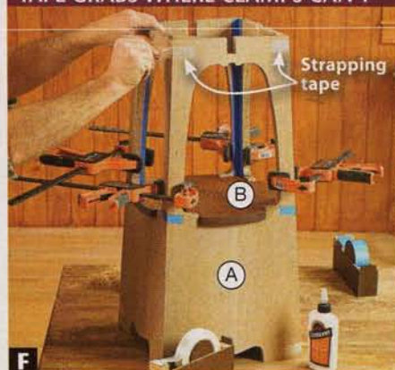
Clamp across corners of the opening where possible. Stretch strapping tape around corners where clamps won't reach.
