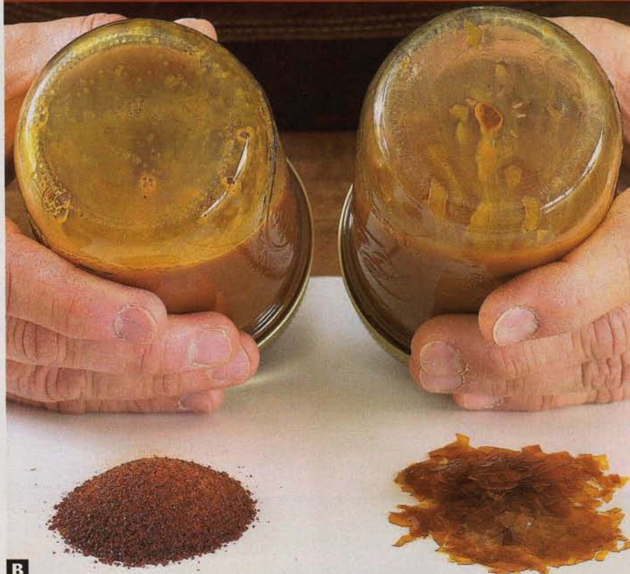
B Grinding flakes to a powder (left) helps shellac dissolve in denatured alcohol, leaving fewer globs on the bottom of the jar.
