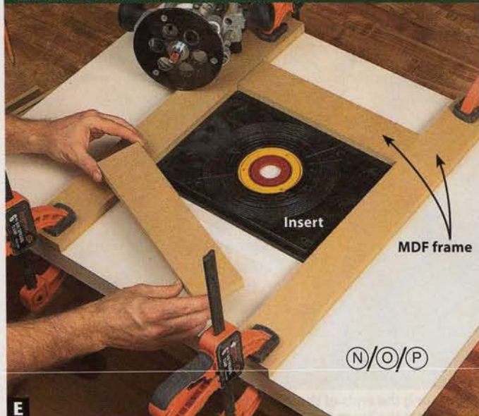
E Center the router-table insert on the top assembly (N/O/P), then frame it with MDF strips wide enough to accommodate your router base.
