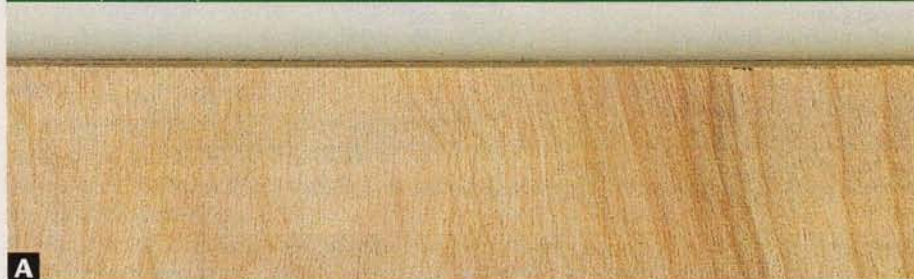
A All five rail-guided saws delivered cabinet-quality crosscuts like this in birch-veneer plywood.
