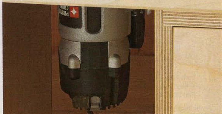
A good table-mounted router makes bit changes hassle-free. An angled wrench to hold the spindle sure helps.
