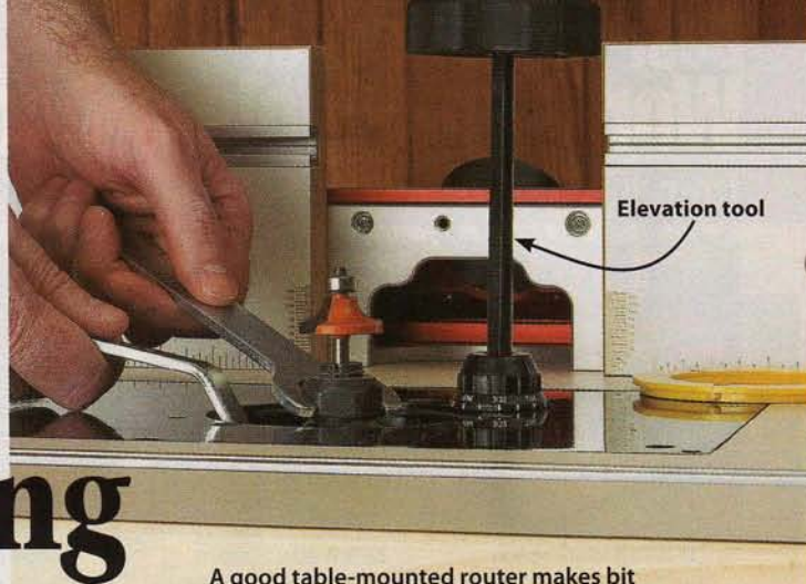
A good table-mounted router makes bit changes hassle-free. An angled wrench to hold the spindle sure helps.
