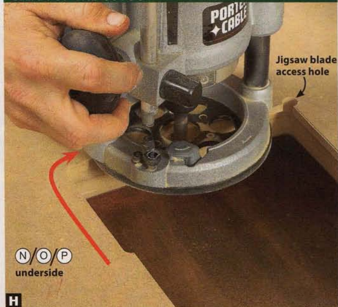
H From the underside of the top assembly (N/O/P), ride the bottom-bearing flush-trim bit against the inside edge routed earlier.
