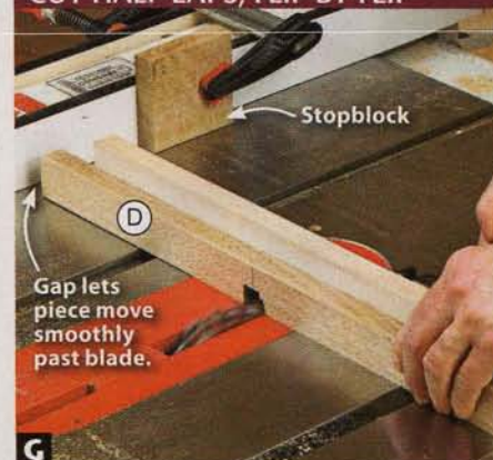
To cut centered half-laps, make a pass with each end starting against a stopblock. Move the fence as needed to widen the notch.
