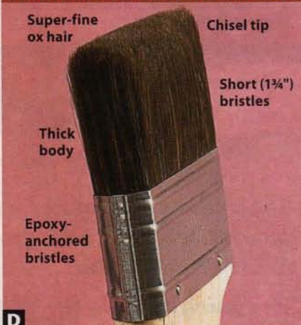
D The finer the hairs, the fewer shellac ridges a brush leaves behind. The thick, gap-free body of this brush leaves less to sand than synthetic-bristle paint brushes.
