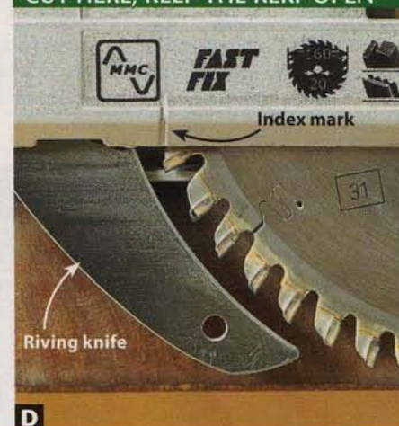
D Index marks show the exact length of the plunge cut. All saws except Makita also sport a spring-loaded riving knife.
