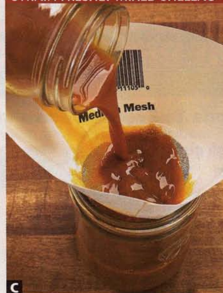
C Allow shellac to dissolve overnight in alcohol; then strain it through cloth or a medium-mesh filter to remove lumps and impurities.
