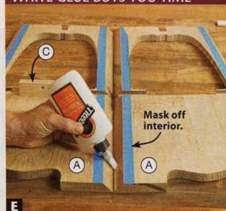
White glue allows more working time during assembly. Glue two sides together, then the other two, then join those assemblies.
