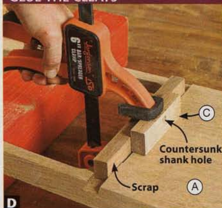
Glue a shelf cleat (C) to each of two of the sides (A), with the countersink on the shank hole facing the bottom.
