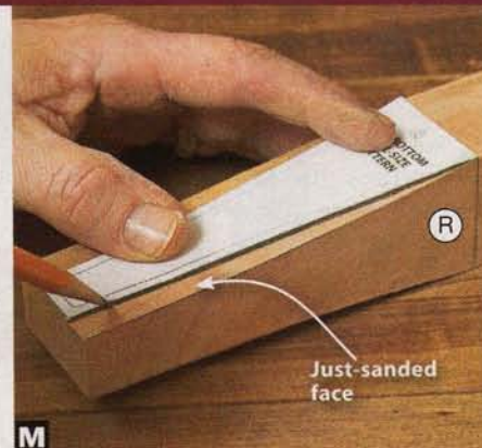
K Trace the tapers on to one face of each leg (R) (left), then cut them on the bandsaw staying just outside the lines. Sand these faces smooth on a drum sander (middle). Then trace the remaining tapers on to a freshly sanded face (right), and repeat the process.
