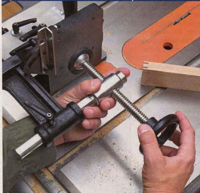
Push the spring-loaded steel button on the end of Jet's clamp arm to instantly reposition the clamp for a wider workpiece.
