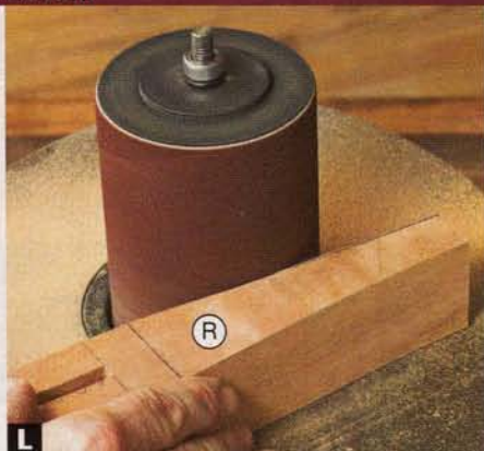
K Trace the tapers on to one face of each leg (R) (left), then cut them on the bandsaw staying just outside the lines. Sand these faces smooth on a drum sander (middle). Then trace the remaining tapers on to a freshly sanded face (right), and repeat the process.
