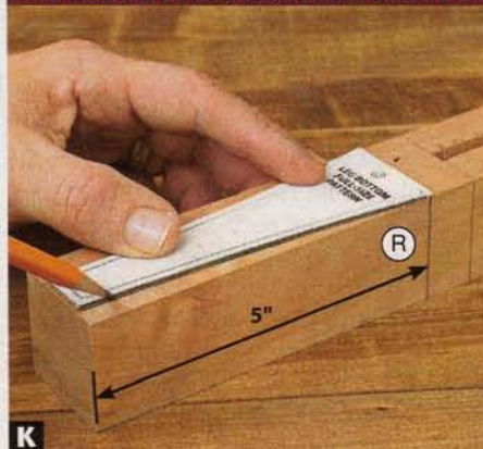
K Trace the tapers on to one face of each leg (R) (left), then cut them on the bandsaw staying just outside the lines. Sand these faces smooth on a drum sander (middle). Then trace the remaining tapers on to a freshly sanded face (right), and repeat the process.
