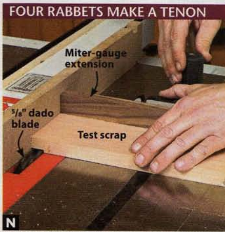
N Cut rabbets on all four edges of a test piece to create a tenon that fits the mortise; then cut tenons on the rails (S, T, U).
