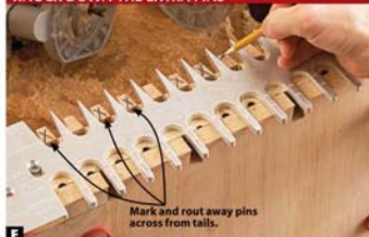
E Mark pins for removal. Those across from a tail get an "X." Leave any pin directly across from a space between tails.
