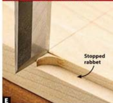
E Straight router bits work fast, but they don't square corners. A sharp chisel completes the rabbet in two quick cuts.
