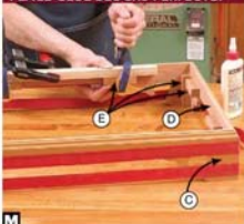
Use a scrap of plywood the same thickness as the bottom (F) to position the glue blocks (E) below the top edge of the base (C/D).
