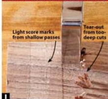
I Test shoulder-plane-blade depth by making passes against the grain on scrap until it leaves light score marks with no tear-out.
