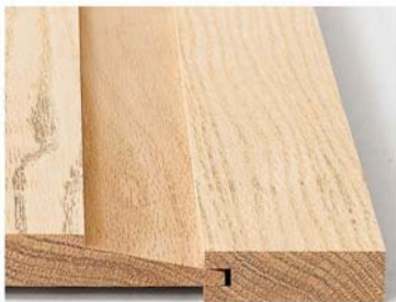
The wedge shape of a tablesawn raised panel is less forgiving of wood movement without planning for its effects.
