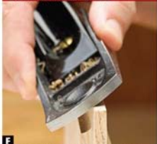
F Help raised panels slide into stile and rail grooves by making a light chamfer on the edges, working from the edges to the center.
