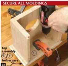
H Clamp the top and case (A-F) to your bench. Then, drill holes to secure the top assembly (E/F), avoiding the handle counterbores.
