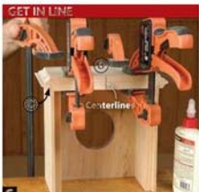
G Centerlines on the back edges of the case molding (D) and top (C) make it easy to align the pieces during glue-up.
