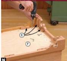
Drill countersunk shank holes through the bottom (F), then screw the base assembly (C-F) to the case (A/B).
