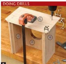
F Align marks on the edge of the top (C) with the edges of the case (A/B). Drill for the two screws along each line on top of the case top.
