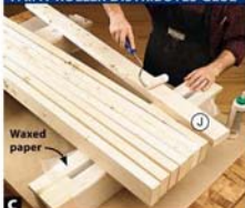
C A foam mini roller quickly spreads glue on the eight top (J) pieces. Waxed paper keeps glue-up hold the top pieces (J) flush while you attach clamps above and below.
