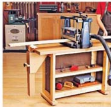
A planer lets you thickness lumber to the needs of the project rather than conforming the project to over- or undersize lumber.
