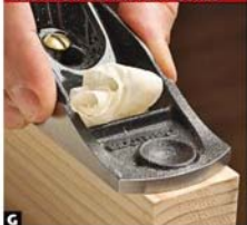
G Passes on the edge of a scrap block should produce light curls of even thickness from side to side.
