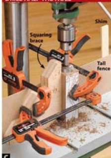
C In addition to making sure the table rests 90° to the bit, use shims to ensure the tall fence holds the workpiece 90° to the table.
