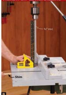
B Add shims to make the drill press table 90° to a rod in the chuck. Check the alignment in all directions using a square.
