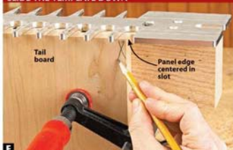
F After repositioning the template and clamping the panels to the spacer, lay out the remaining dovetail cuts.
