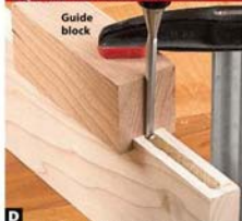
D Clamping a guide block—this one with a grooved underside—to your workpiece helps keep the chisel 90° to the edge.
