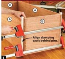
Clamps and cauls apply pressure on the front and back (A), pressing the dovetails tightly to the sides (B).
