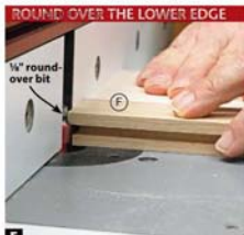
E To provide more support for the handle block (F) as you rout the \frac{1}{4} " round-overs, align the fence with the bearing of the bit.
