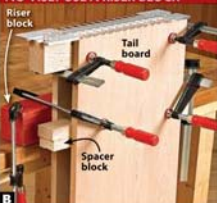
B Clamp the panels and jig to a riser block clamped to your bench. Sandpaper on the riser-block face keeps things from slipping.
