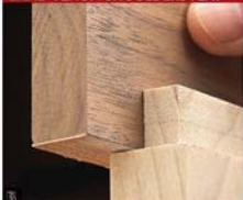
B This block sands the tenon shoulder but leaves the cheek untouched. Check blocks for square between the edges and faces.
