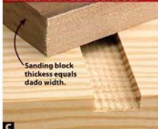
C To flatten dados cut with a saw blade, attach sandpaper to a block of scrap and sand away the ridges.
