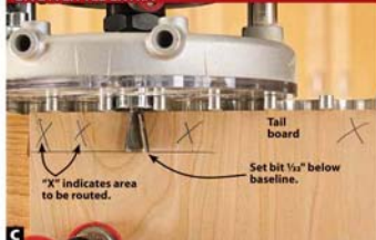
C Mark the waste between the tails. Then set each bit so the pins and tails stand proud of the panels. Sand them flush after assembly.
