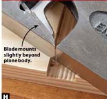
H With a blade that cuts just wider than the plane body, a shoulder plane takes shavings right up to the walls of a dado or grooves.
