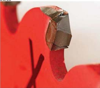
Hidden damage could equal dangerous shrapnel if this broken blade is used again before being properly repaired.
