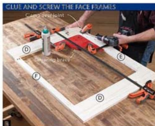
Clamp the face-frame rails (E, F) and stiles (D) while driving the pocket screws. A clamp on top of the joint holds the pieces flush.
