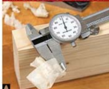
A “Paper-thin” takes on new meaning with a well-tuned plane. This shaving thickness equals that of the paper on this page.
