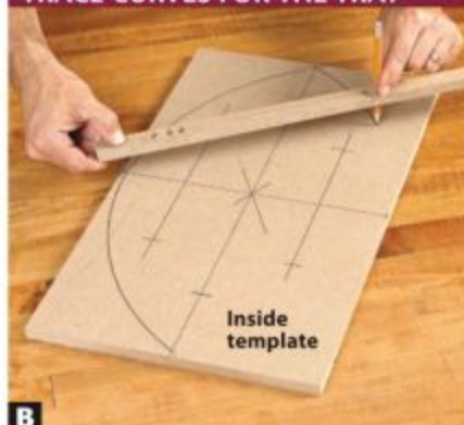
B After marking centerlines on the templates, mark the centers of curves. Use the beam compass to draw connected arcs.
