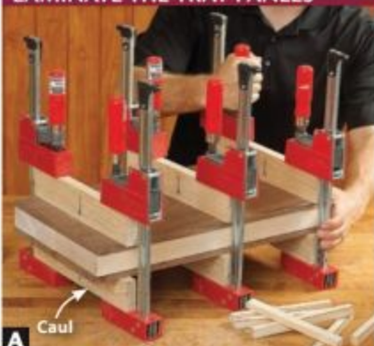
A Cauls evenly distribute clamping pressure from the edges to the center of the glue-up. Arrows on the cauls mark the curved edges.
