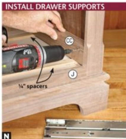
N Place \frac{1}{4} " spacers below the drawer supports (CC) to bring them flush with the top face of the bottom trim (J).
