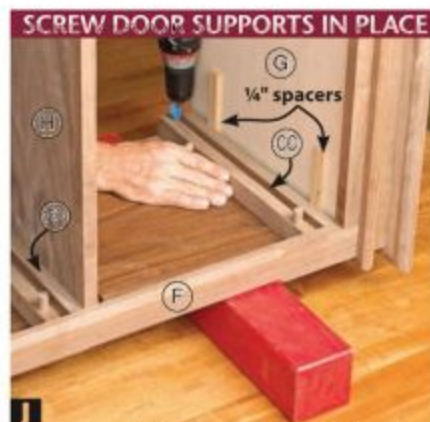
J Secure the middle door supports (CC) against the bottom of the shelf (H). Use \frac{1}{4} " spacers to position the upper door supports.
