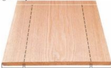
Riftsawn grain Flatsawn cathedral grain Riftsawn grain
