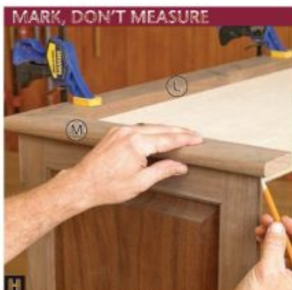
H With the trim front (L) clamped to the case, place the mitered end of a side (M) against it and mark the final length of the side.
