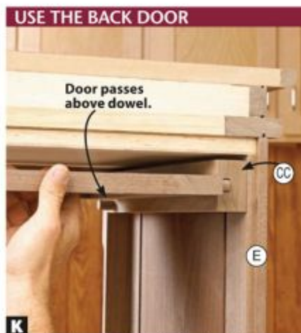
K Slide the doors in from the back of the case, bottom edge first, so the door passes above the dowel in the door support (CC).
