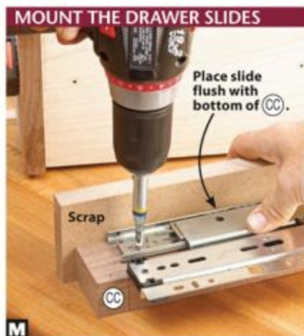
M Using a scrap and the mark on the drawer support (CC) for alignment, screw the drawer slide to the drawer support.
