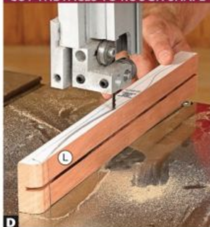
D On the bandsaw, cut just outside the pattern line on each drawer face (L, M, N); then sand up to the line on a drum sander.
