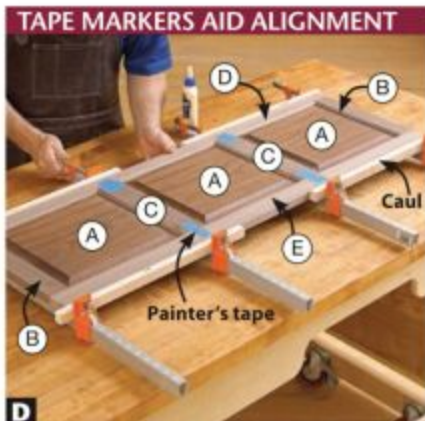
D Line up the pieces of painter's tape to position the rails (C) quickly during glue-up. Cauls protect the edges of the stiles (D, E).
