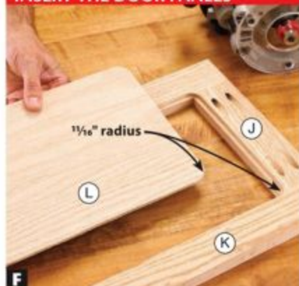
F Sanding the panels (L) before they're glued in place eliminates the problem of sanding in tight corners.
