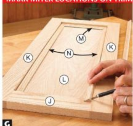
G By scribing the outside edge of the door trim (N) with a crafts knife instead of a pencil, you can miter the end for an exact fit.
