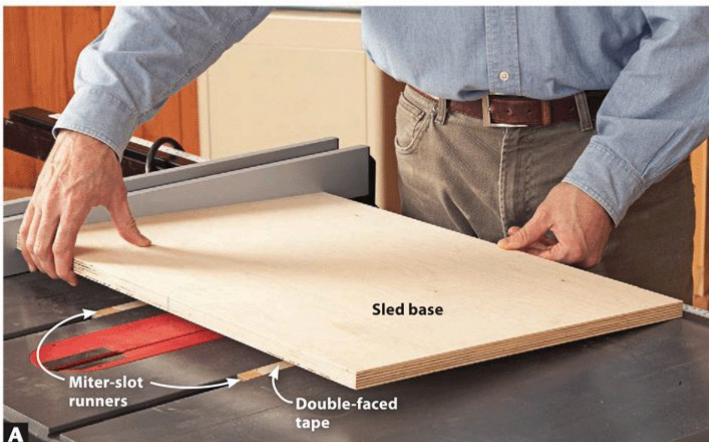
A Attach double-faced tape to the miter-slot runners and align them with the front edge of the saw table. Press one edge of the sled base against the rip fence as you tilt the sled down against the table and press it against the miter-slot runners.
