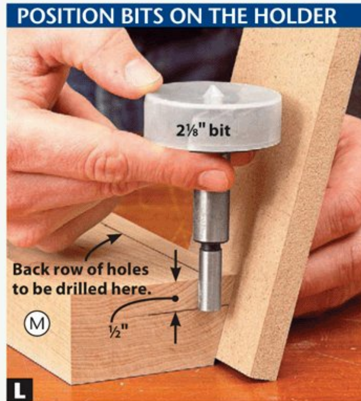
L Mark one end of a Forstner bit holder (M) 1/2" from the top face for the bit hole depth. Hold a scrap against the bevel and position your largest Forstner bit (2 1/8" in our set) with the shank bottom on the line on the end of the bit holder and the top clear of the scrap. The bit shank center indicates where to mark a line for the back row of holes.
