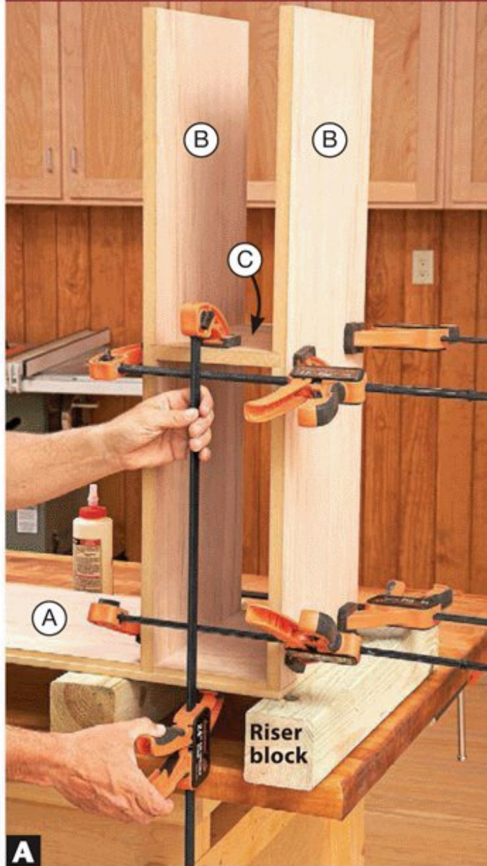
A Rest one upper case side (A) on riser blocks for clamp clearance and glue the upper shelf, bottom (B), and divider (C).
