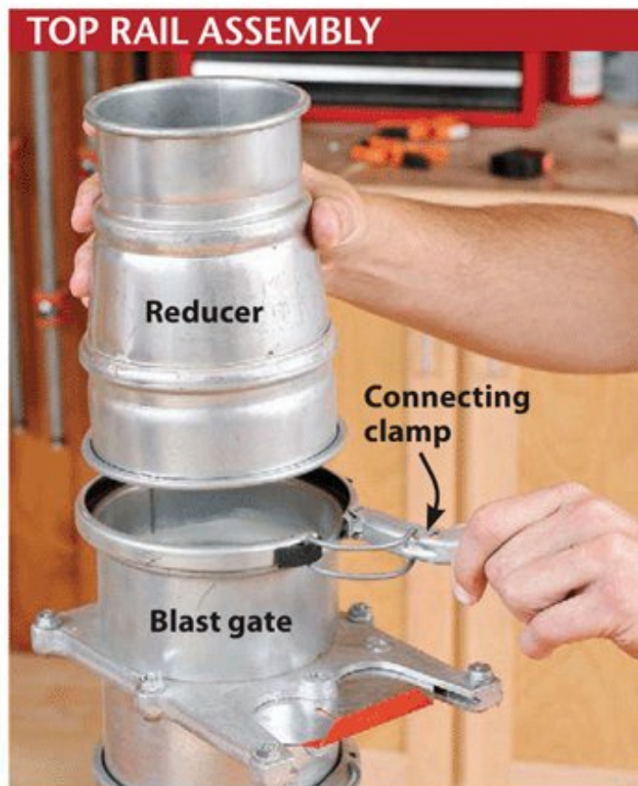
This reducer connects to corrugated hose or narrower duct. Connecting clamps let you reconfigure this type of metal duct.
