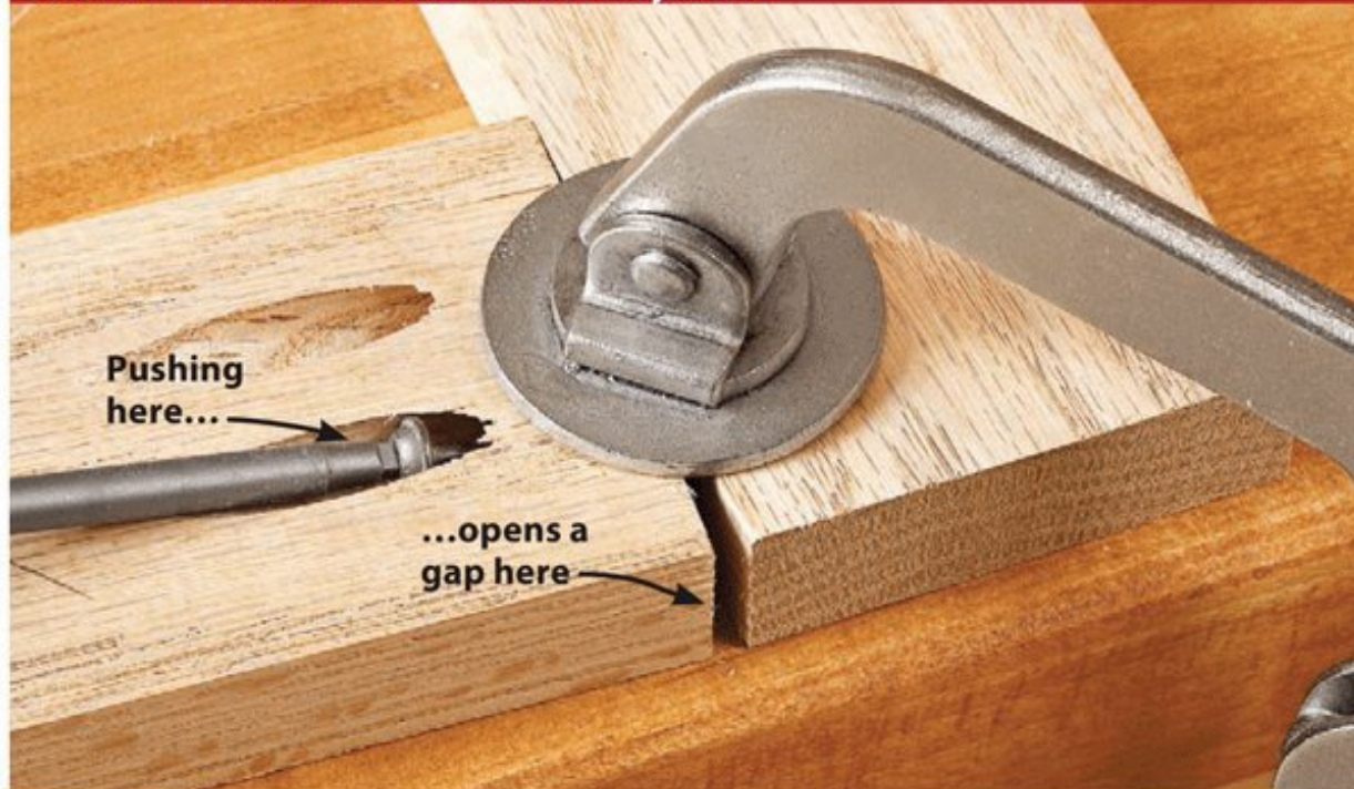
Driving the screw separates a poorly clamped joint, throwing off the part alignment even if the screw pulls the joint back together.
