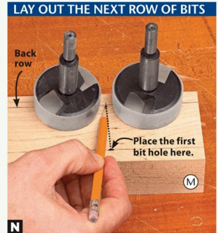
N To lay out the front row of Forstner bits, position the back row of bits with their spurs on each centerline marked in the previous step. Parallel to the center of the spaces between the bits, mark centerlines on the front row line. At each centerline, on both rows, drill a 1/2"-deep hole the shank diameter of the bit to go there.
