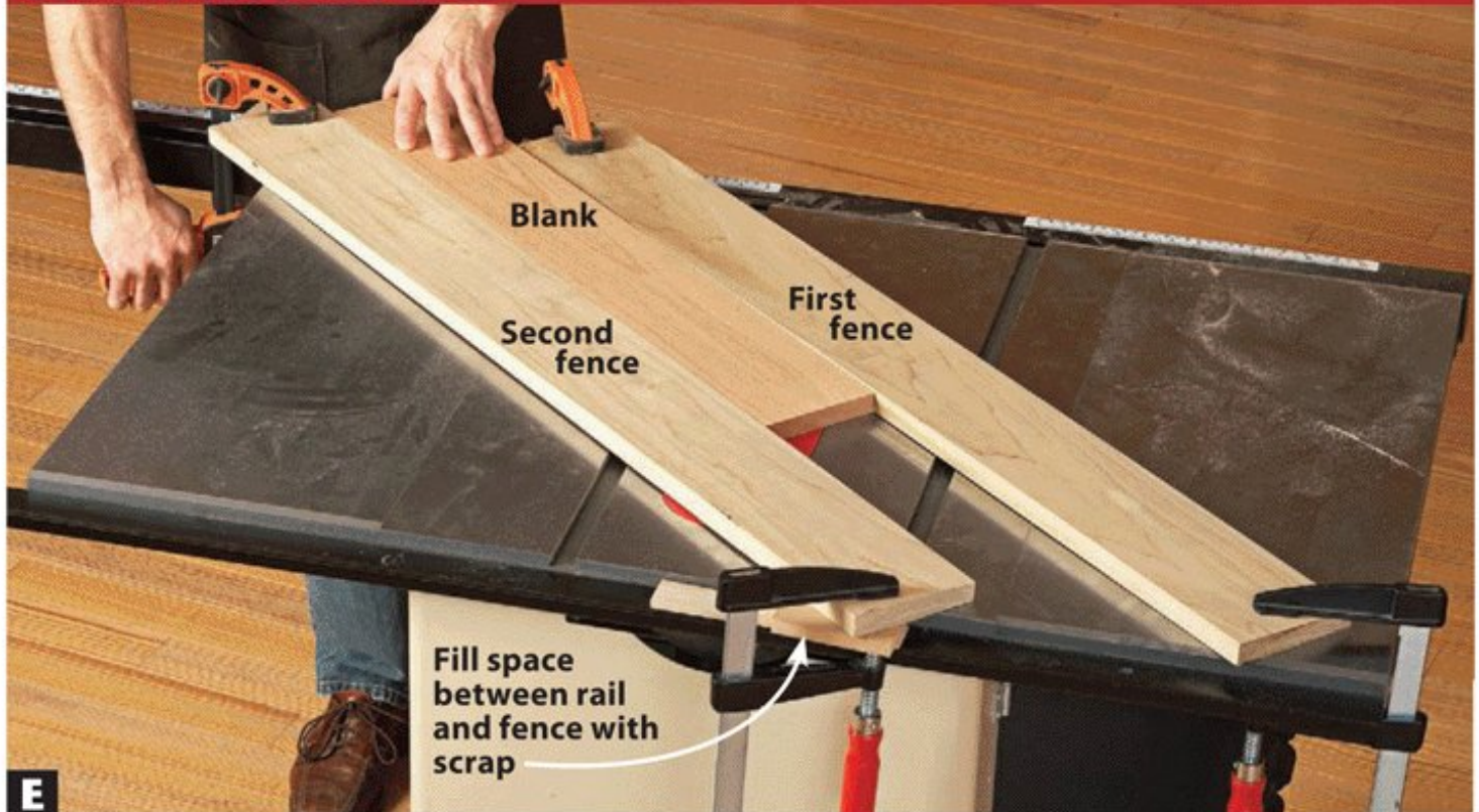
E Place a molding blank against the first fence to position the second fence. The blank must slide between the fences without binding.
