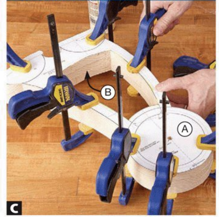
C While gluing up the body front (A) and back (B), align the outlines as closely as possible to minimize sanding.
