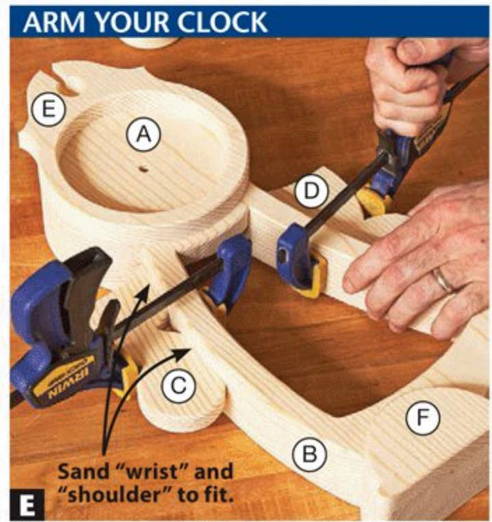
E Sand "wrist" and "shoulder" to fit. Glue the arms (C, D) to the body (A/B/E/F/G) centered on the thickness of the body. Use glue sparingly to minimize squeeze-out.
