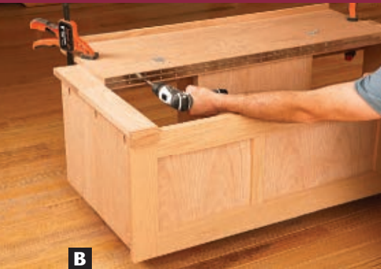
B Double-faced tape the hinge with the barrel centered between the window-seat lid and the top back and screw the hinge in place.
