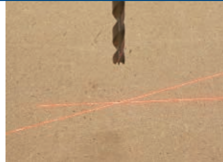
General International's lasers overlap for more than ⅓", making it difficult to pinpoint an exact drilling location.
