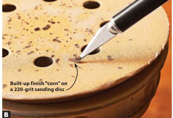
B When finish heats and softens, it can stick to itself to form corns on an abrasive. Remove these or change pads frequently.
