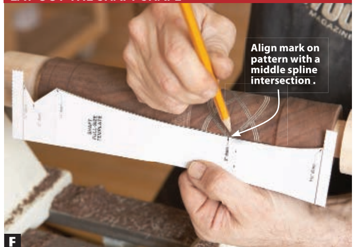
F To lay out the shape of the lamp shaft, align the "2" diam." mark on the pattern with the middle intersection of two rings.
