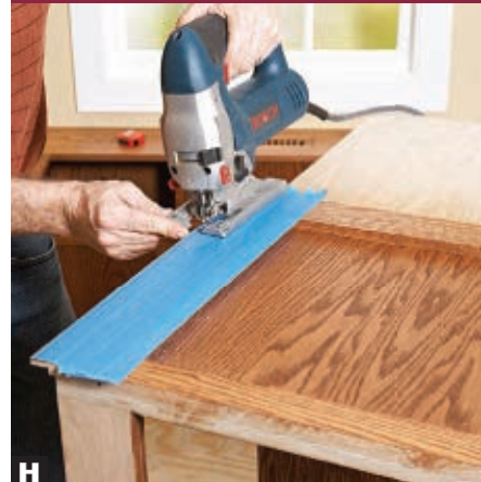
H By angling the jigsaw cut slightly, it's easier to sand or plane the stile to your scribe line. Tape protects the wood finish.
