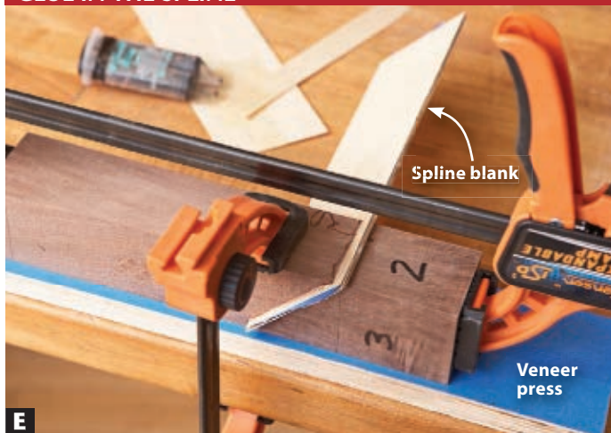
E Place the trued-up edge of the spline against the kerf bottom. Clamp the blank as shown. The veneer press catches any epoxy drips.
