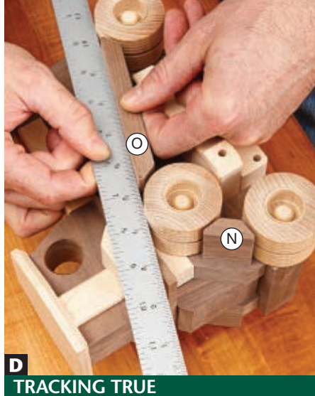
D TRACKING TRUE Bridge two wheels with a straightedge to position the upper face of the tracks (N, O). Hold them in place for a couple of minutes.
