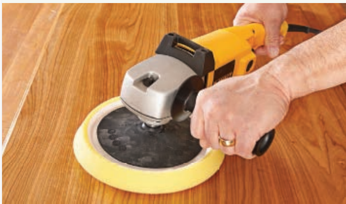
C Stop sanding immediately if you notice circular patterns in the sanding dust caused by corns on the sanding disc.
