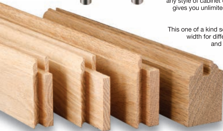
Standard stub tenons in regular 3/4" stock
