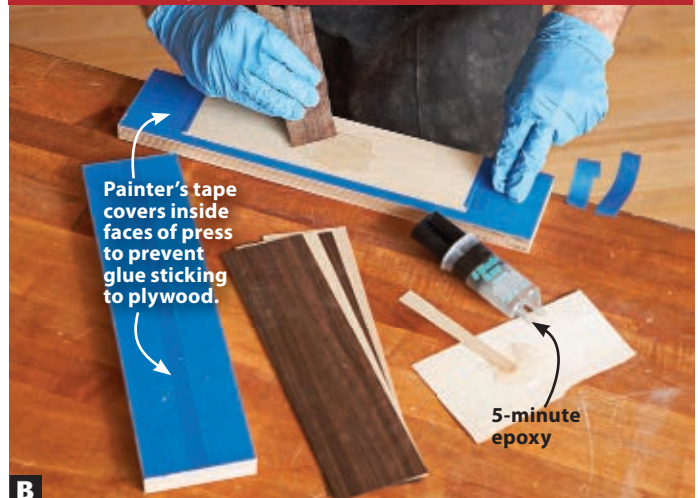
B Tape a layer of veneer to the press, spread five-minute epoxy, and tape the next layer down. Work quickly before the epoxy sets.
