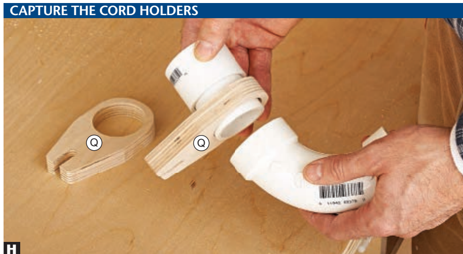
H Cord holders (Q) slip around pipes between fittings. Epoxy and pressure from the fittings against the holders keep them in position.
