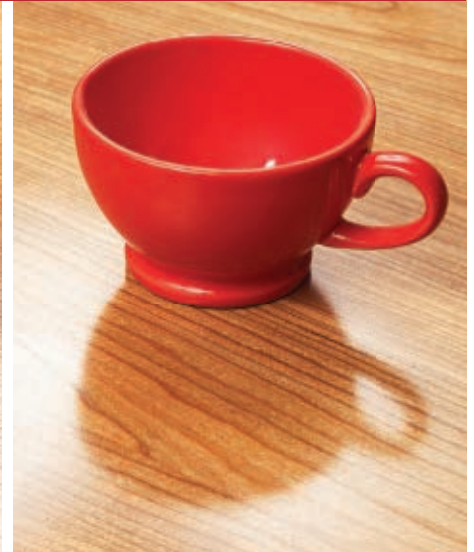
Before it was rubbed out, the satin finish (left) blurred objects and highlighted surface flaws. After rubbing (right), the sheen becomes more even in reflected light despite not being glossy.
