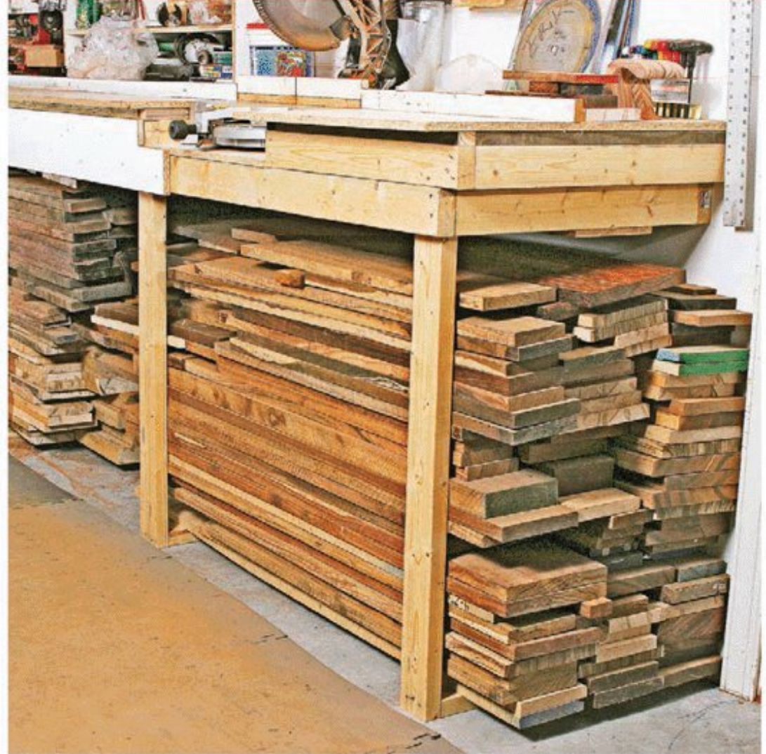
Space beneath this miter saw bench houses short to medium-length lumber, keeping it flat and off of the floor.
