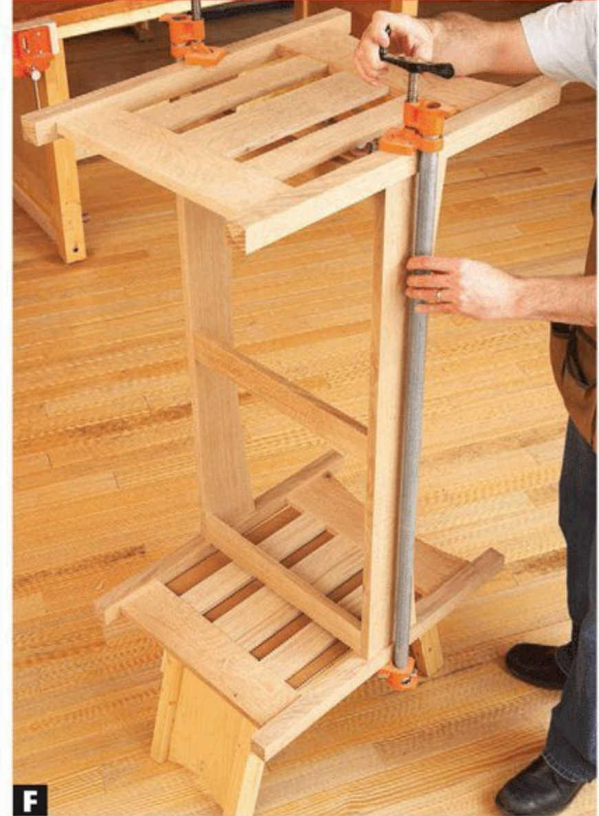
F Elevating the bottom side assembly provides clamp clearance. After clamping, rest all four legs on a level surface and check for square.
