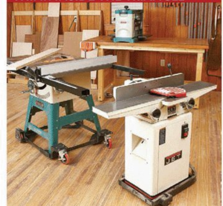
Size and square project parts quickly by placing the table saw, jointer, and planer within steps of each other.
