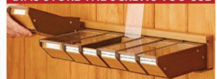
Put this on your to-do list: Removable shop-made bins keep your most popular fasteners organized, dust-free, and accessible.
