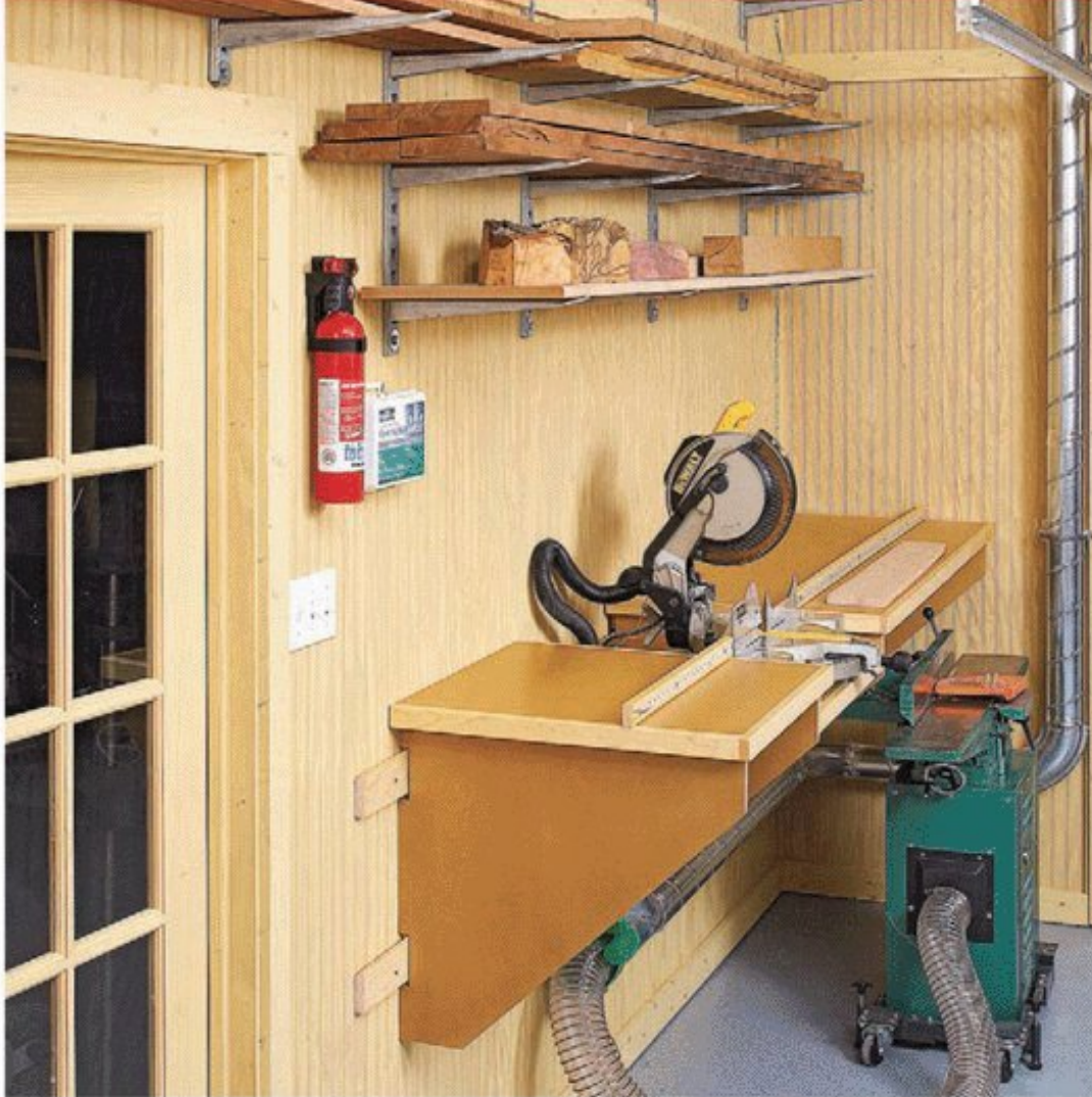
This garage shop's storage system organizes lumber over a cutting center with space below to park the jointer when it's off-duty.
