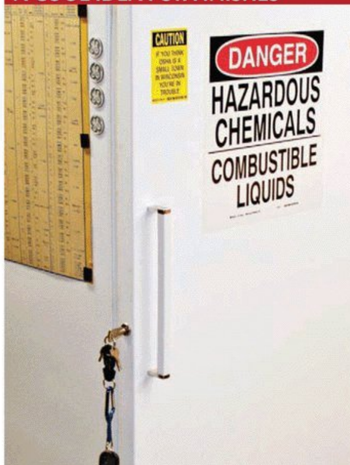
A discarded freezer, minus its refrigeration unit, provides lockable, insulated, and airtight storage for finishes.
