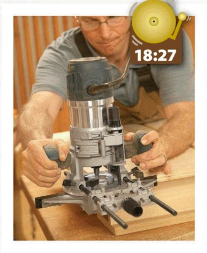
Jeff routs the first of the two 1/4" back rabbets. Job completed at 19:44.
