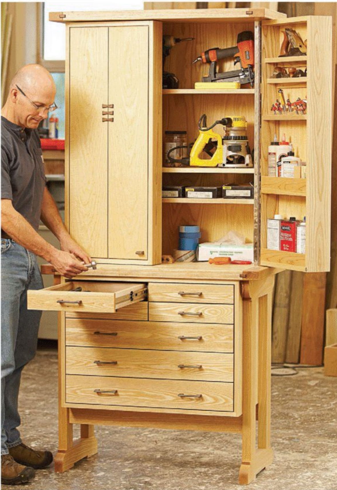
Heirloom Tool Chest Organize tools and supplies in a cabinet handsome enough for the house, but meant to work hard in the shop. Simple drawer and door joints, cut on the tablesaw, speed construction.
