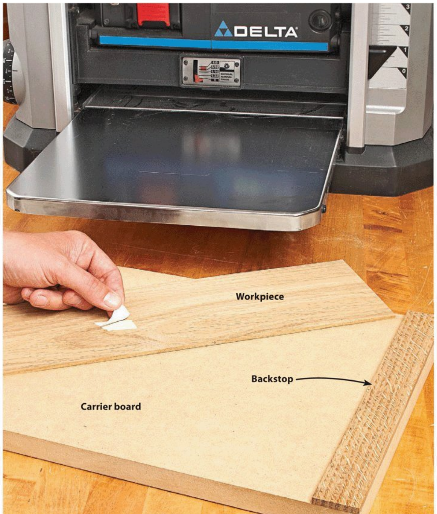
The backstop prevents slipping, while the planer's rollers hold the workpiece against the carrier board. All that's needed is a small piece of tape to prevent side-to-side motion.
