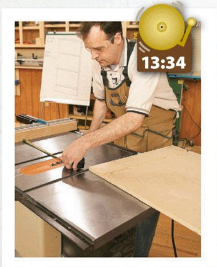
Because the stacked dado set and auxiliary fence nullify the fence scale, Kevin uses a measuring tape to set the rip fence to the correct position for the third dado.
