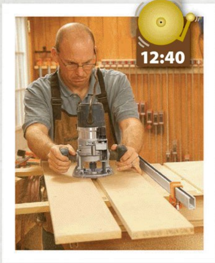
Jeff begins his third dado in the actual workpiece. (He cut the 3/4" top rabbet earlier using the guide bushing and jig.)
