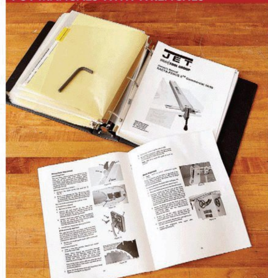
In addition to tool owner's manuals and service information, this binder stores setup wrenches for each tool.
