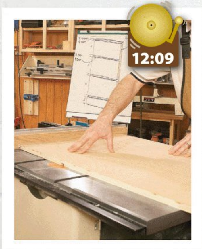
After resetting the rip fence, Kevin cuts his first dado, second cut overall.
