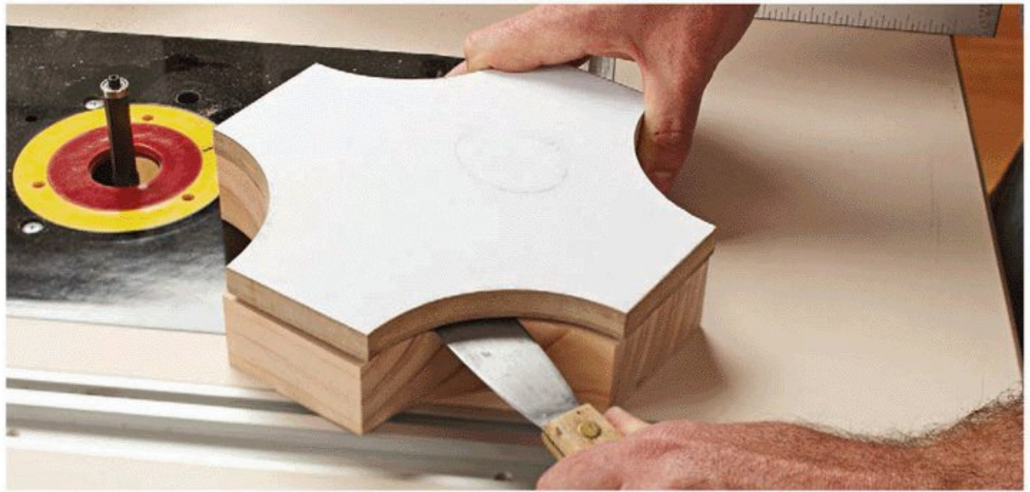
After routing with a template, slip the thin, broad, steel blade of a putty-knife between the workpiece and the template, and then twist to pop them apart.
