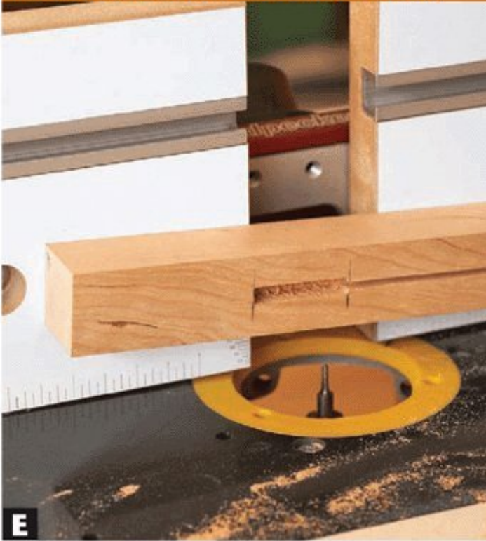
E Begin the groove by dropping the mortise over the straight bit. Stop when the bit reaches the opposite mortise.
