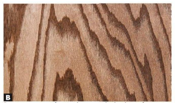
Rotary-cut veneer often produces an unbroken layer of veneer across an entire sheet of plywood that can look unnatural.
