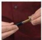
Step 2: Mount pen blanks onto the lathe blanks to desired with pen mandrel
