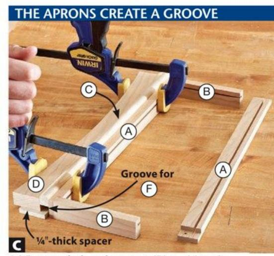
A ¼" spacer below the apron (D) positions it. The apron, bead (C), and bottom (A) create a groove that the bottom (F) fits into later.
