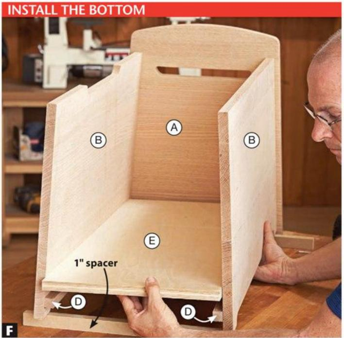
Gently spread the front and back (B) apart to slide the bottom (E) above the cleats (D) without smearing the glue beads.
