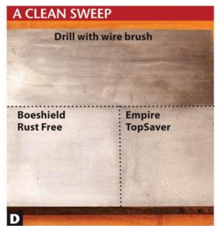
All three methods removed the rust on our set of cast-iron tablesaw wings, each requiring about 5 minutes.
