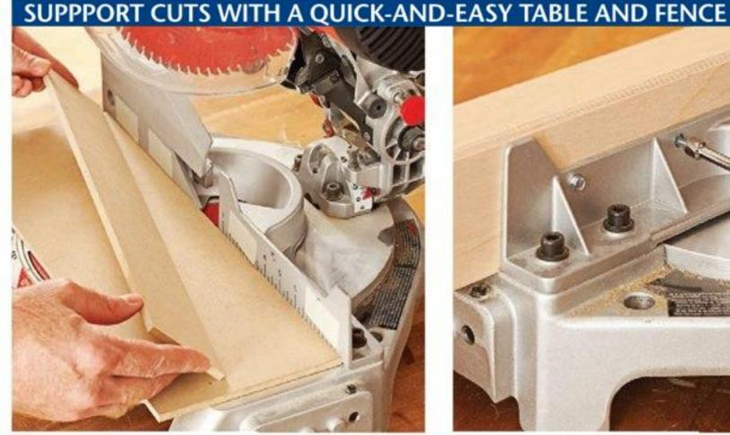
For the quickest setup, use double-faced tape to attach an auxiliary table and fence to the saw's table and fence.
