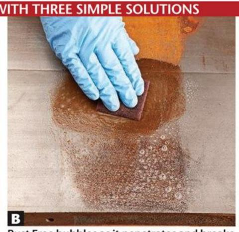
Rust Free bubbles as it penetrates and breaks down the rust. It also emits a strong odor, so work in a well-ventilated area.
