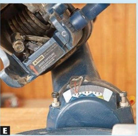
The fat cursor line and closeness of Ryobi's bevel-angle markings make it difficult to accurately set an angle without a stop.
