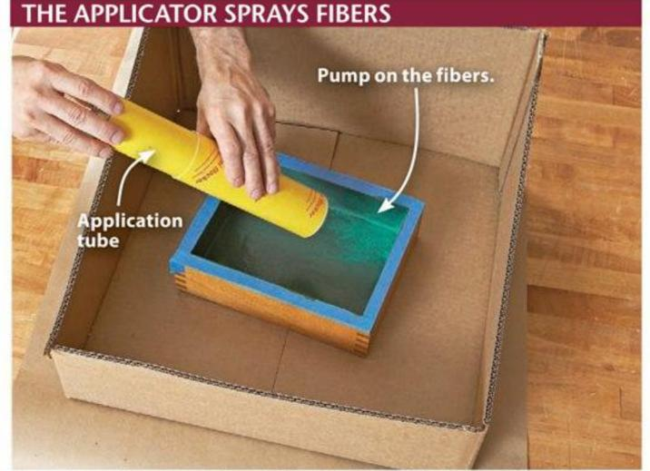
A cardboard box contains drifting flocking. Apply the fibers generously. After the adhesive dries, collect excess fibers for reuse.
