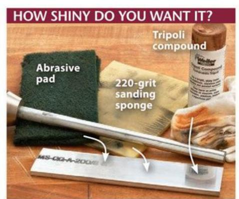
Polish rods quickly by spinning them in a drill. Buff on tripoli compound with a soft rag. For flat aluminum, use a buffing wheel.
