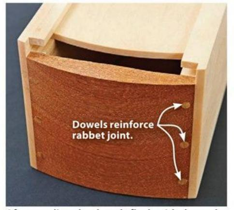
After sanding the dowels flush with the end panel and applying a finish, the end-grain provides a subtle accent.
