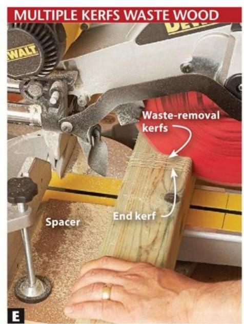
Holding the workpiece against the spacer, remove much of the wood waste from the joint with kerfs spaced about every 3/16".
