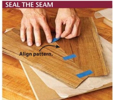
Painter's tape holds the joint together during glue-up. Clamp the substrate and veneer between ¾" MDF or plywood platens.
