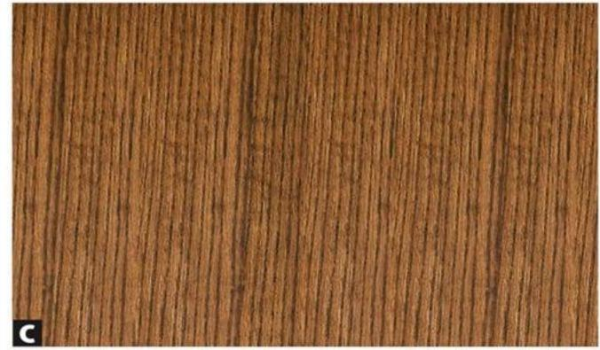
In a slip-matched face, subsequent pieces of veneer from the log are "slipped" out side-by-side to form a repeating grain pattern.
