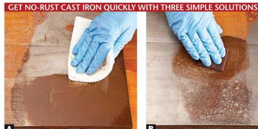
Apply TopSaver, then wipe away the rusty residue before the solvent dries, which typically happens in 3 to 5 minutes.
