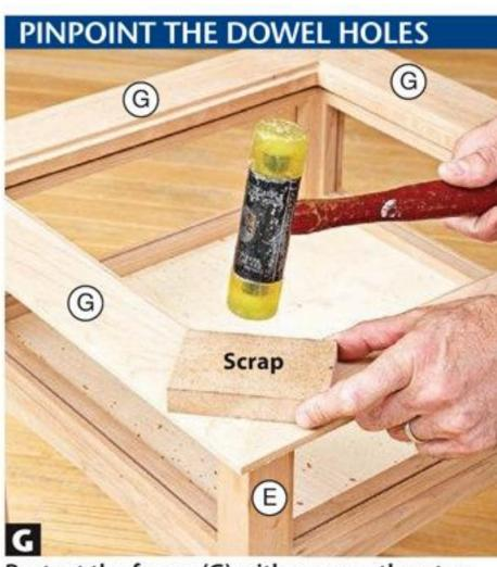
Protect the frame (G) with a scrap, then tap each corner directly above the leg so the brads leave a dimple on the underside.
