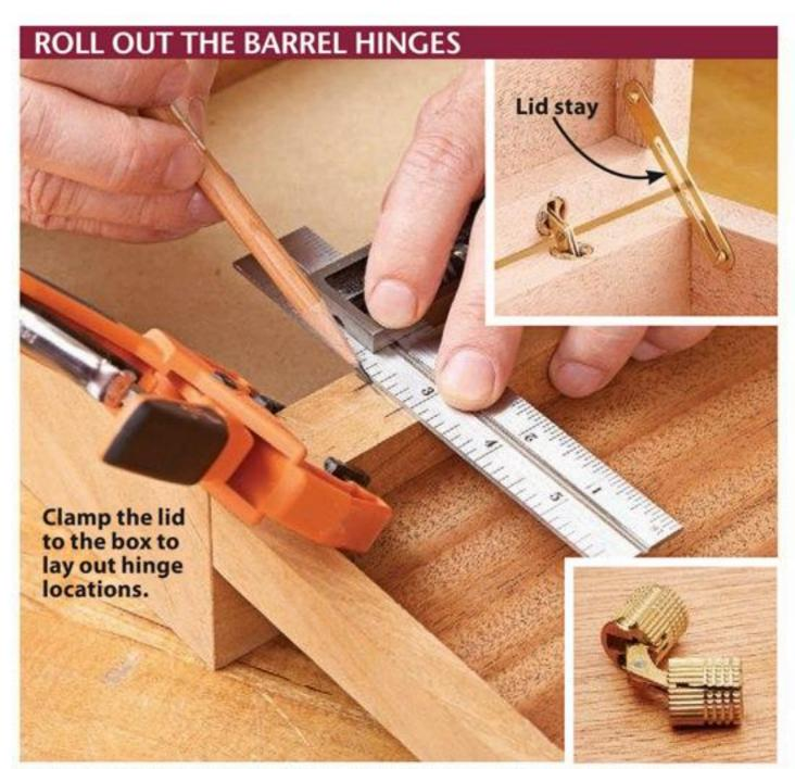
Bore 10mm holes centered on the thickness of the lid and box, then seat the hinges. Add a lid stay, top inset, to hold the lid open.
