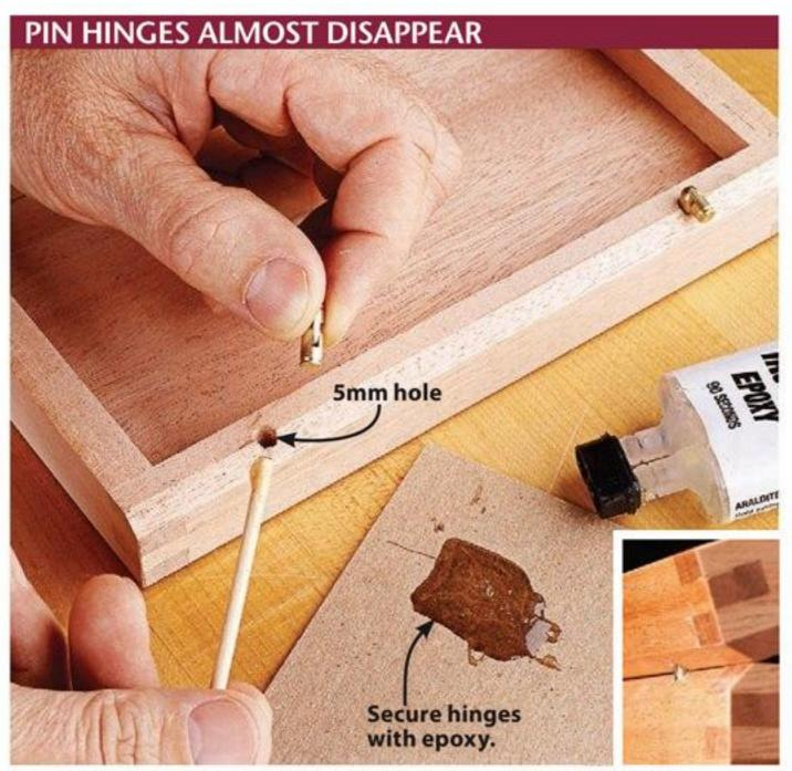
Bore 5mm holes centered on the thickness of the edges of the lid and box. The chamfered edges serve as a stop to hold the lid at 90°, inset.
