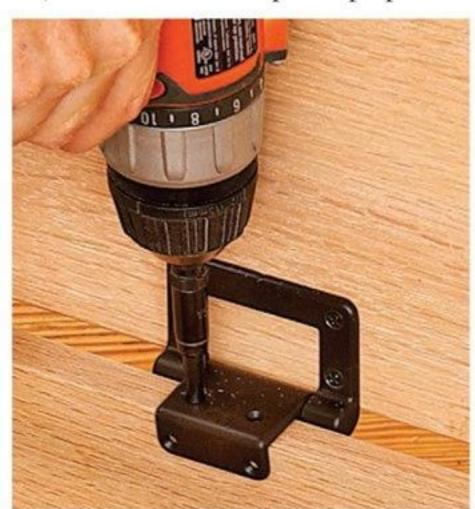
computer hinges, these Lid-Stays hold a lid in place at any angle, preventing it from dropping onto the chest. That's especially valuable when children reach into a toy box to retrieve toys.
