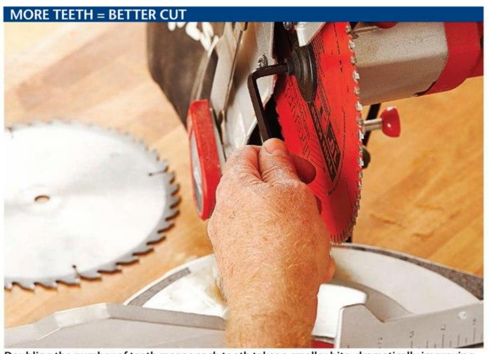
Doubling the number of teeth means each tooth takes a smaller bite, dramatically improving the quality of cut. And using a blade with sharp, clean teeth nets a cleaner cut.
