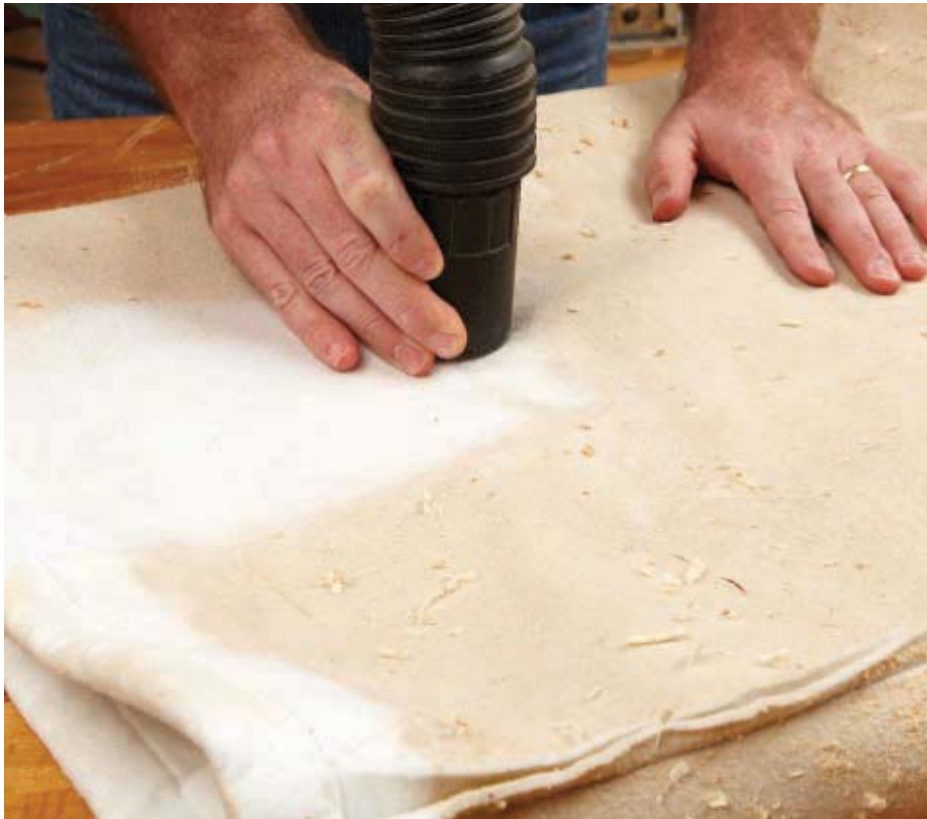
Vacuuming the inside of your dust filter bag will remove most of the built-up dust cake that can clog the fabric.
