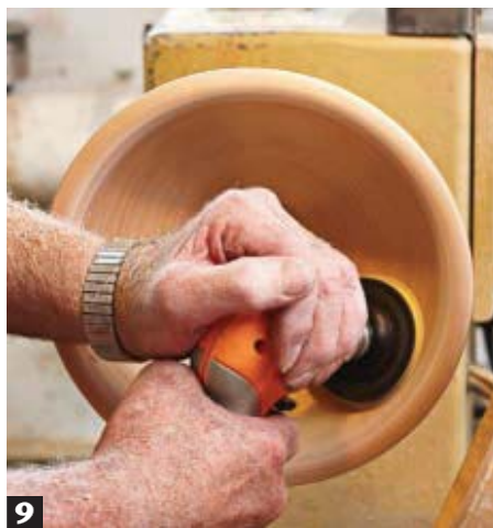
9 After rounding over the rim, turning away the stump, and cutting to final shape, sand the inner wall smooth. A right-angle sander like this helps hide sanding scratches.
