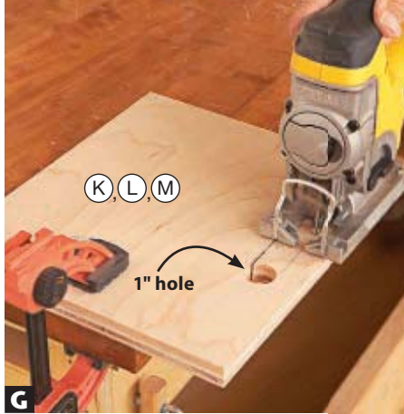
G Using your jigsaw, cut along the inside of the lines on the fronts/backs (K, L, M) to remove the waste and complete the openings.
