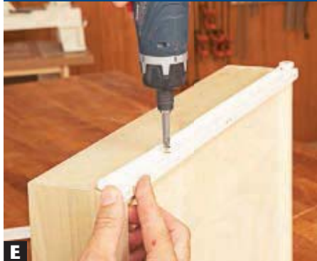
C Measure at the front and rear of the cabinet to make certain the slide runs parallel to the cabinet side.
