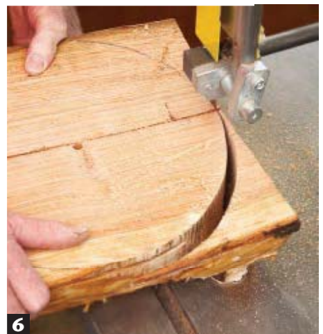
6 Bandsaw the blank round. Don't suck the moist debris into your dust collector—it could plug the filter. After sawing, clean your bandsaw to prevent tabletop rust.
