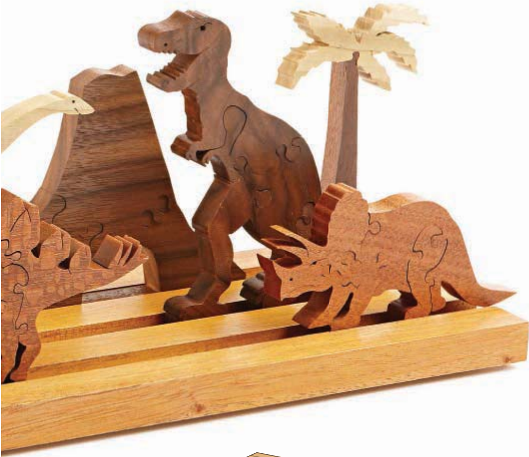
A Align the patterns on the treetop (B) and tree trunk (C), then stack-cut both pieces to shape. Keep them together until you finish cutting the lobe that connects the two parts.
