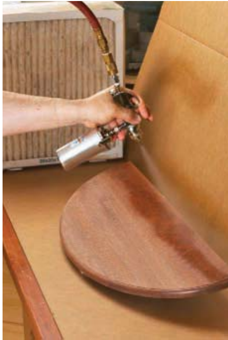
For spraying water-based finishes, a box fan with a furnace filter taped to the intake side directs odors toward the nearest window.
