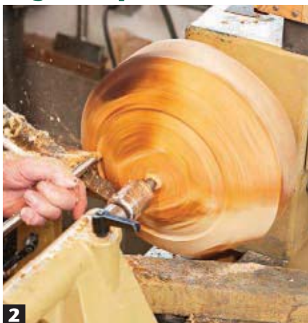
2 With the tailstock and live center helping to support the blank and the lathe running at its slowest speed, use a \frac{1}{2} " bowl gouge to begin shaping the outer surface.
