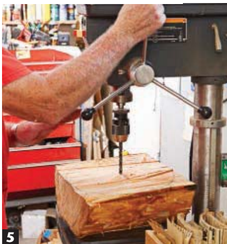
5 Drill a pilot hole for the screw-chuck threads in the center of the blank. Or, if you use a faceplate, drill pilot holes where needed for the mounting screws.
