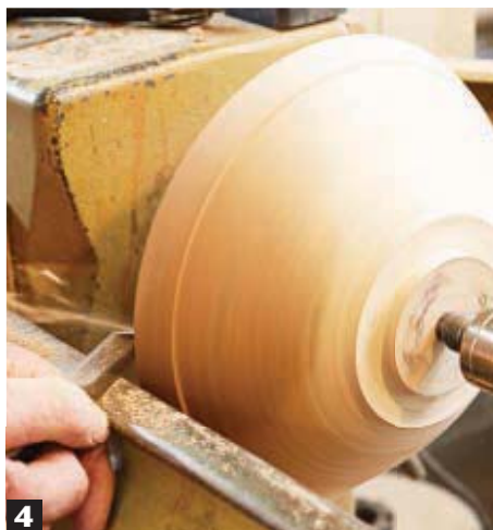
4 As you did with the green bowl, use the parting tool to define the rim. Continue cutting until you have a rim that's true around the entire bowl.
