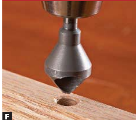
F A 1/16" countersink keeps the hole edges from swelling and pushing the joint apart.
