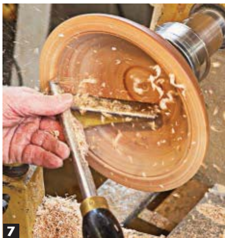
7 Holding the gouge as shown, push into the spinning bowl, removing about \frac{1}{8} " per pass. Hold the gouge's beveled edge against the bowl wall and chase the shape to the center.
