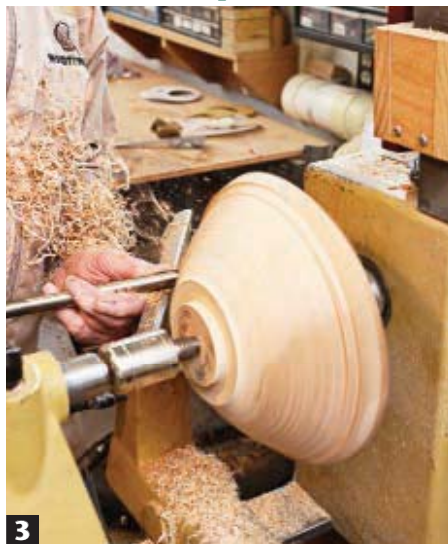
3 Turn the outer surface of the bowl to make it round again. Place the gouge's bevel against the wood near the foot and push-cut toward the rim. Use ultralight cuts to finish the shape.
