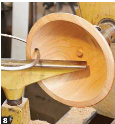
8 Measure the wall thickness until reaching your desired amount. Leaving the "stump" in the center serves as a gauge of how much material you've removed since starting.
