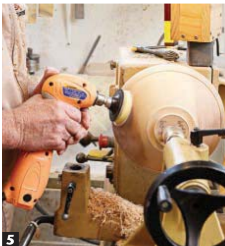
5 With the bowl's outer shape to your satisfaction, sand it smooth, beginning with 120-grit sandpaper and continuing through 320 or 400. Apply finish to the bowl's outside.
