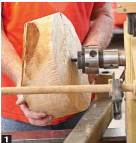
1 Thread the bowl blank onto your screw-chuck with the drive spindle locked. Snug the blank up so it sits flat against the jaws around the entire chuck.
