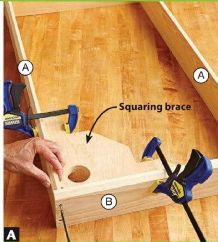
A SCREW THE SLAT FRAMES Clamp the front/back slats (A) between the side slats (B), drill two countersunk pilot holes at each joint, then assemble the frames.
