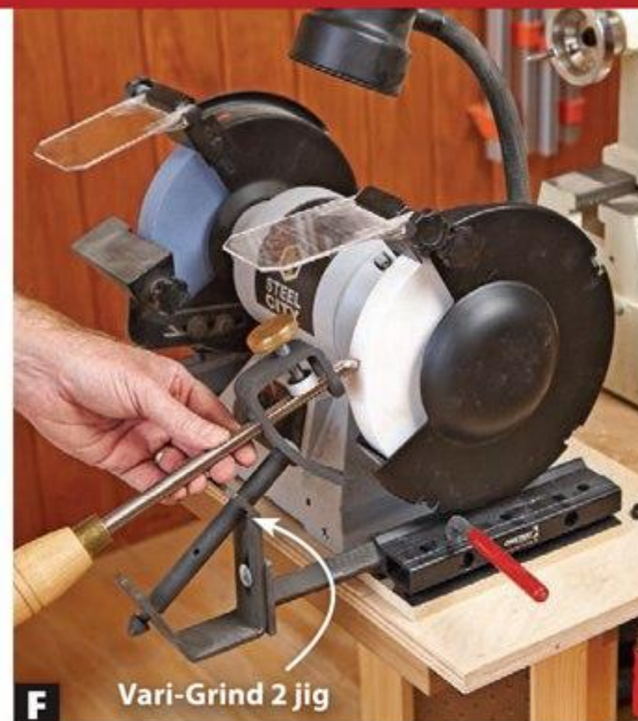
F Replace the basic rest with one designed for woodturning chisels; then quickly and repeatably put a sharp edge on any gouge.
