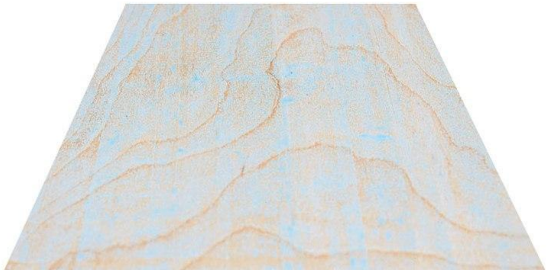
Blue chalk reveals the slight linear peaks—separated by shallow valleys—caused by the convex blades of a spiral cutterhead.
