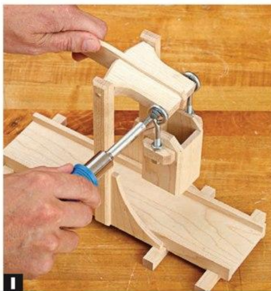
I Tighten the wood screws in the arm brackets (G) enough to secure the bucket assembly while ensuring that it pivots freely.
