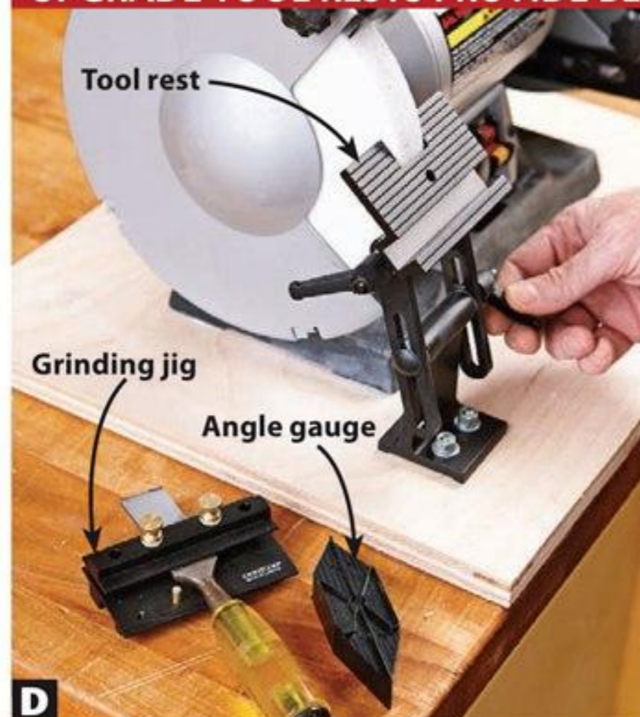
D Veritas’ tool rest adjusts at two points, so experiment with it in multiple positions to find the best mounting location.
