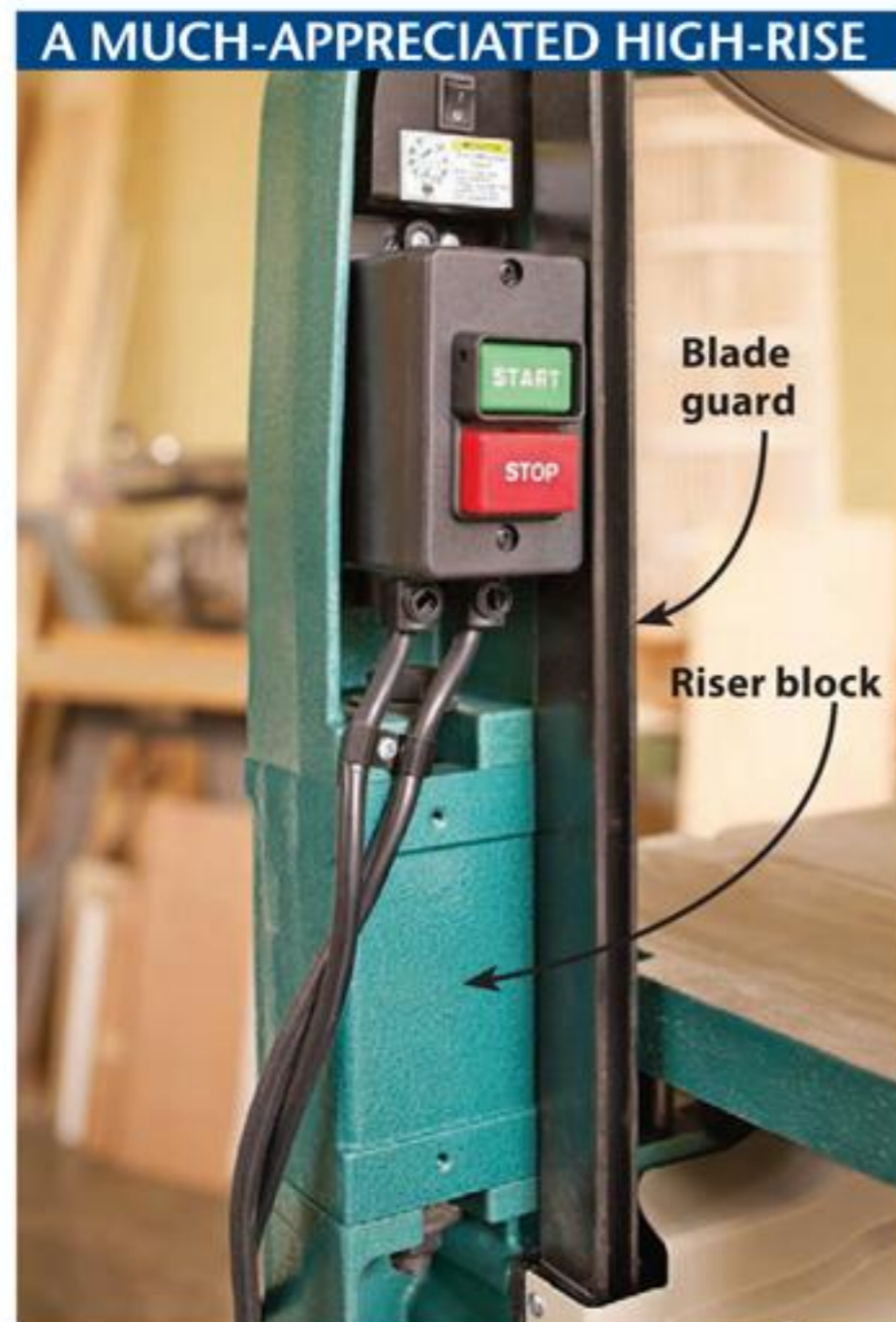
A riser-block kit comes with the block, a connecting bolt, and extended blade guards. It takes about 20 minutes to install.
