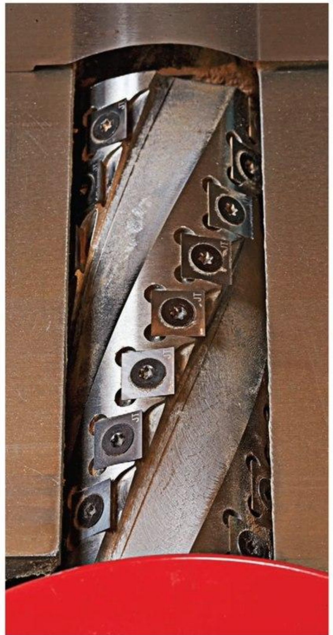
The many square cutters on a spiral cutterhead make adjustments easy but typically leave a slightly less-finished board.
