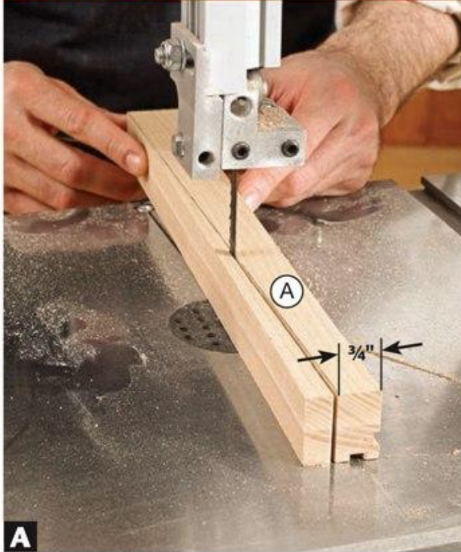
A Taper one face of each column corner (A). After cutting and smoothing this taper, lay out the second taper on the newly cut face.
