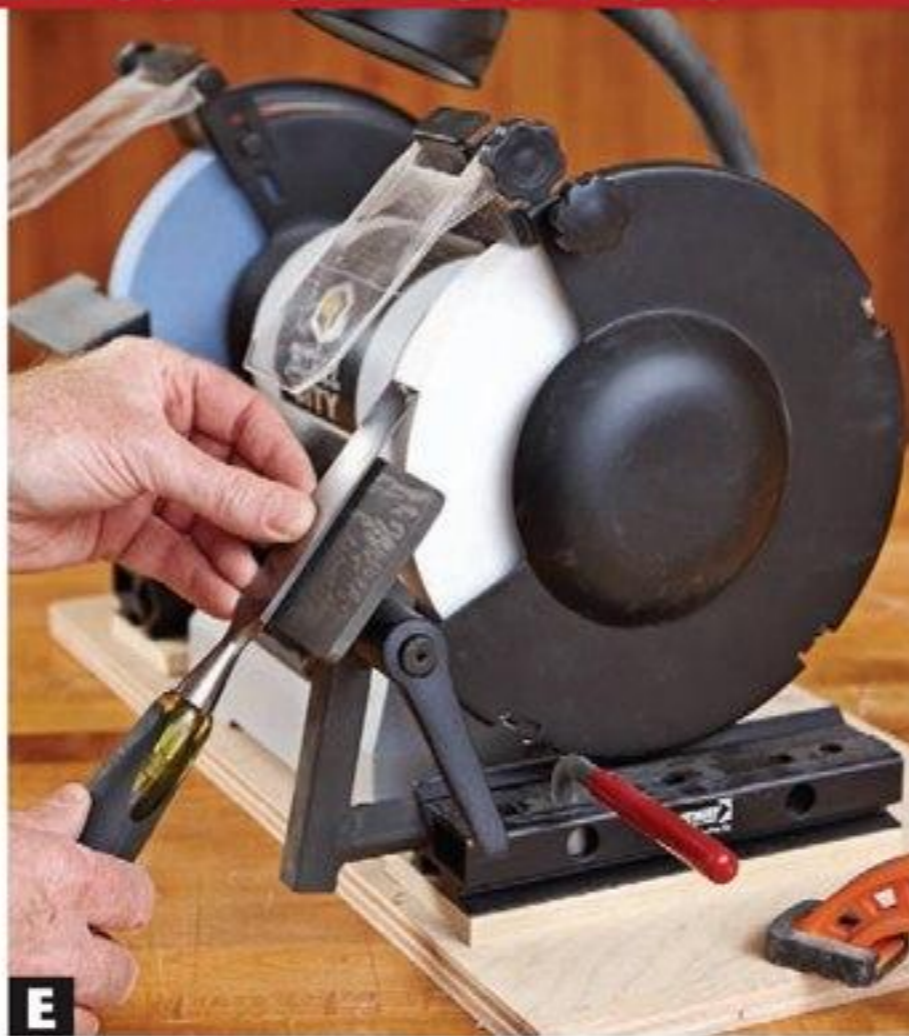
E Use the Wolverine’s basic tool rest to sharpen chisels and plane irons. The shelf adjusts 90° for any bevel you’ll need.
