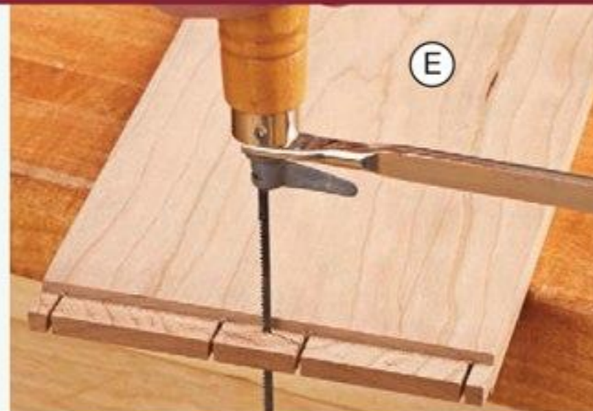
Make the first coping-saw cut angling from one kerf to the back corner of the other. Then saw out the remaining waste.
