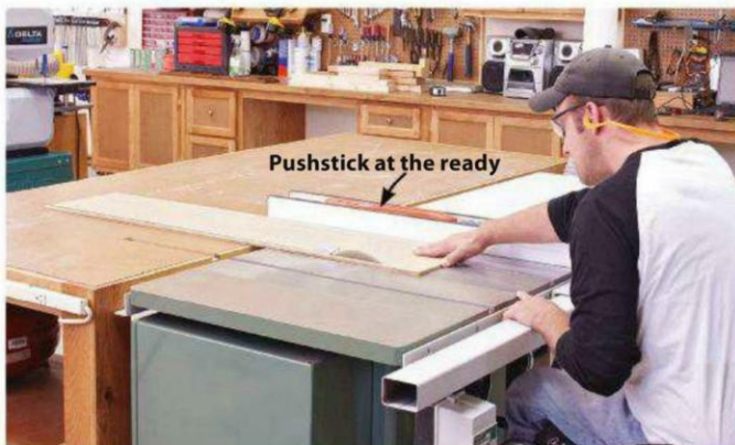
D Finally, Chuck completes the cut, relying on his ample outfeed table to support the workpiece. For narrow pieces, he finishes with a pushstick.
