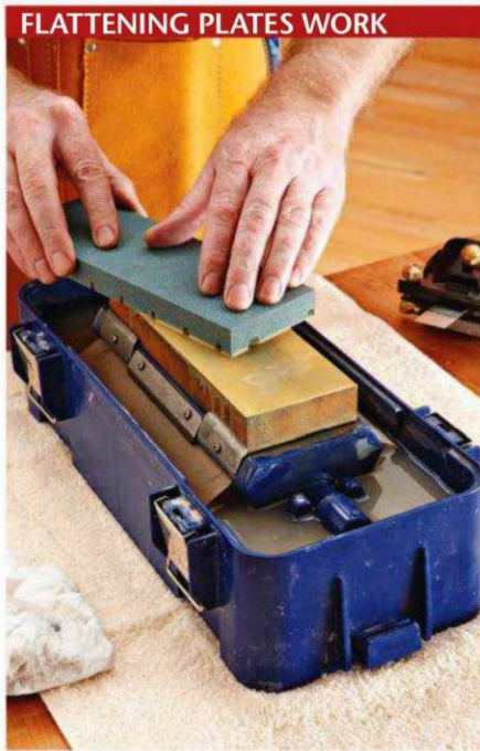
FLATTENING PLATES WORK Rub the flattening plate until the stone's darker low spot disappears. Grooves in the plate channel away waste material.
