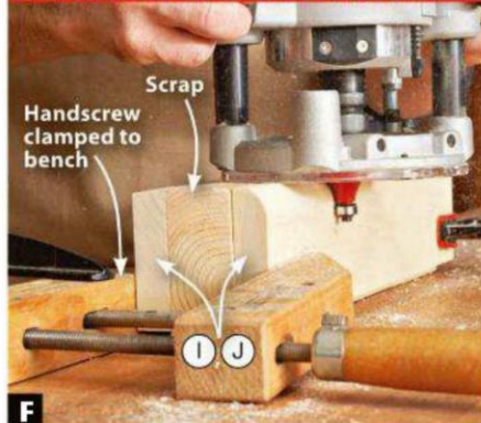
F Sandwich a wide scrap with the top moldings (I, J), clamp the assembly to your bench, then rout the partial round-over.
