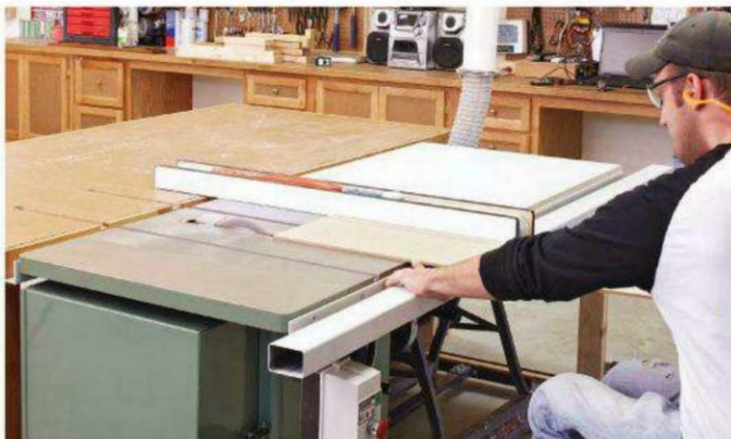
A Positioned an arm's length from the tablesaw, with the brakes of his chair partially engaged to hold him in place, Chuck begins guiding the workpiece through the blade.
