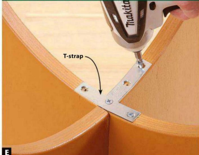
E Bend a 3 x 3" T-strap to fit the curve at the bottom intersection of the legs (A). Drill pilot holes and screw the strap in place.
