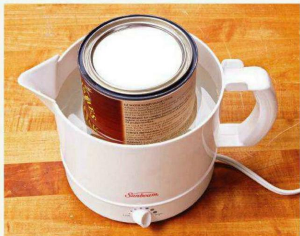
An electric beverage warmer gently warms a cold can of finish to room temperature. Loosen the can lid before heating.
