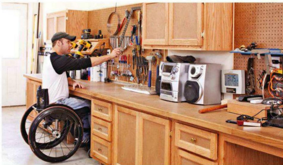
Chuck's shop displays a distinct "waterline" showing the extent of his 6' reach from a sitting position. Wide roll-under spaces keep him close to tools and workpieces.
