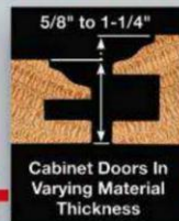
Adjustable Grooves For Variable Panel Thickness
