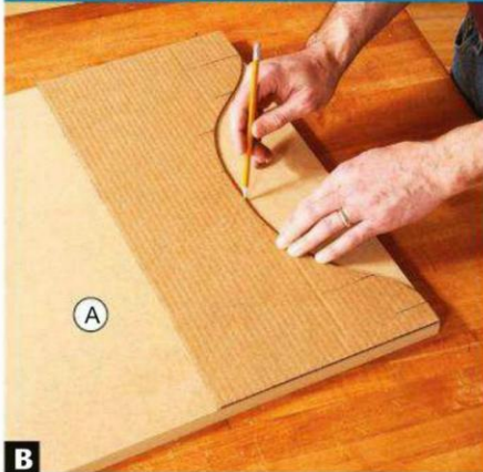
B Align the template flush with the ends and an edge of each leg (A). Trace the curve, then flip the template to lay out the other edge.
