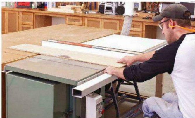
B Seated on the edge of his chair, Chuck leans forward as he feeds the workpiece until it is fully supported by the table and at the limit of his reach.
