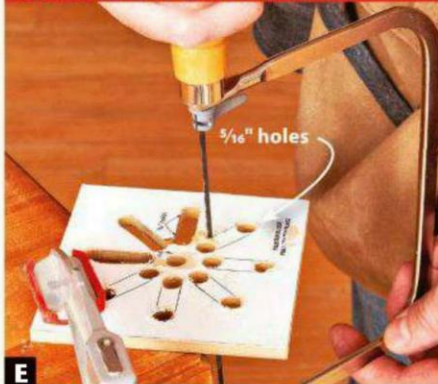
E Assemble the coping saw so the teeth cut on the downstroke. Cut inside the lines, then smooth the edges up to the lines.
