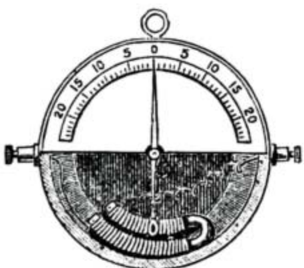
Fig. 2.—Small Electro-Magnetic Pendulum Ammeter: Lower half of Dial removed to show Magnet and Pendulum.
