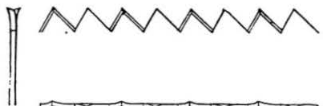
Fig. 9.—Teeth of Hand Saw for Hard Wood.
