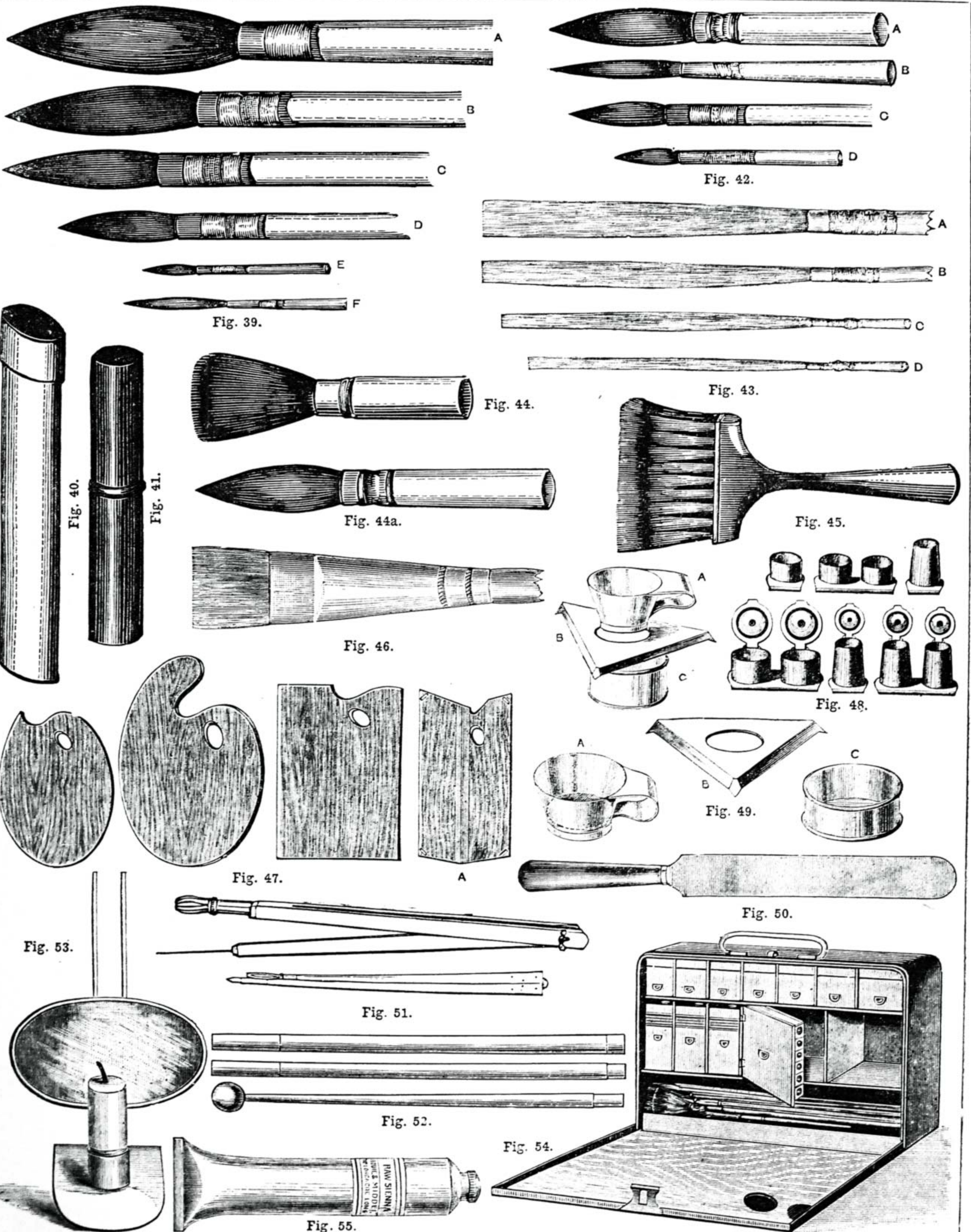
Fig. 39.—Writers—A, Large Swan; B, Small Swan; C, Goose; D, Duck; E, Lark; F, Crow. Fig. 40.—Oval Pencil Case. Fig. 41.—Round Pencil Case. Fig. 42.—Riggers—A, Goose Short Pencil; B, Duck Short Pencil; C, Crow; D, Lark. Fig. 43.—Liners or Tracers—A, Goose; B, Duck; C, Crow; D, Lark. Fig. 44.—Short Hair or Filling-in Brush. Fig. 44a.—Filling-in Brush with Tin Ferrule. Fig. 45.—Badger Hair Softener or Blender. Fig. 46.—Writer's Sable Blender. Fig. 47.—Mahogany Palettes. Fig. 48.—Dippers, Single and Double. Fig. 49.—Sign Writer's Paint Strainer—A, Strainer; B, Stroddle; C, Water Dish. Fig. 50.—Palette Knife. Fig. 51.—Divider and Compasses. Fig. 52.—Jointed Mahl or Rest Stick. Fig. 53.—Sign Writer's Candlestick with Shifting Reflector. Fig. 54.—Brodie and Middleton's Sign Writer's Complete Outfit in Japanned Tin Box. Fig. 55.—Tube Colour for Sign Writer.
