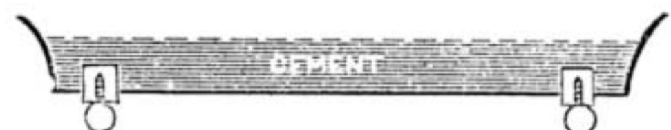
Fig. 5.—Mode of Pocketing Castors before Rockwork is put on. Castors are subsequently bedded in Cement.
