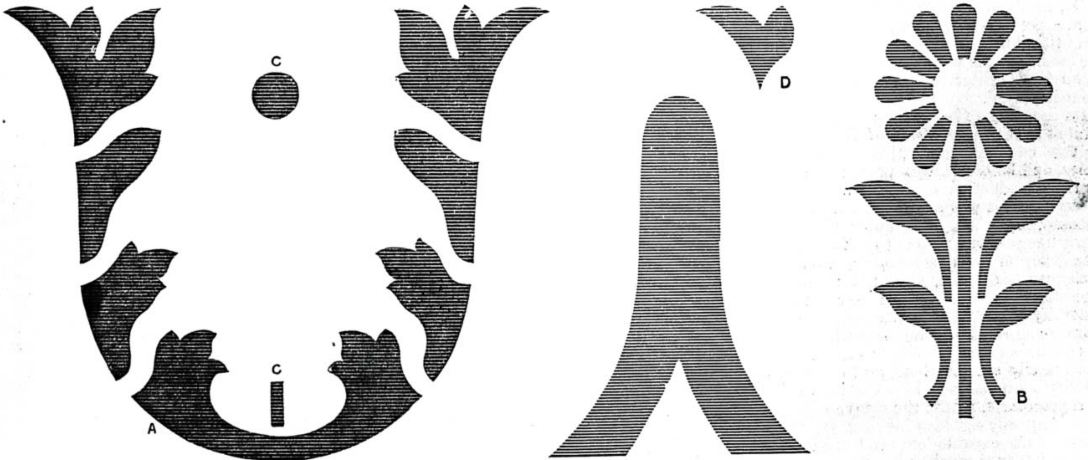
Fig. 4.—Example of Stencil in Two Colours, requiring Two Plates as above.
