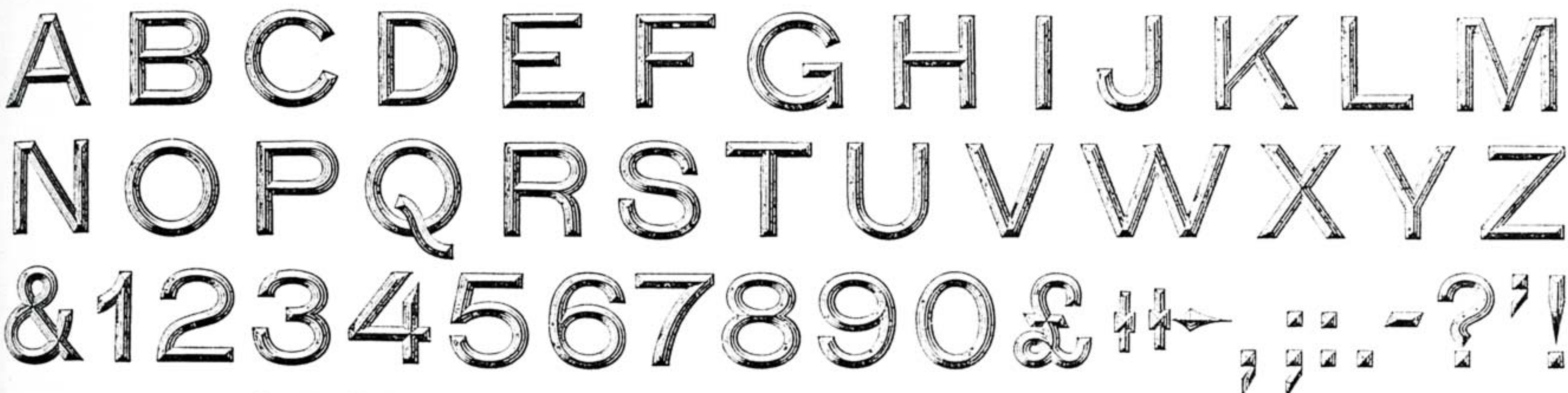
Fig. 67.—Tablet Alphabet, Capitals, Numerals, Points, etc., to Illustrate Method of Shading Letters.
