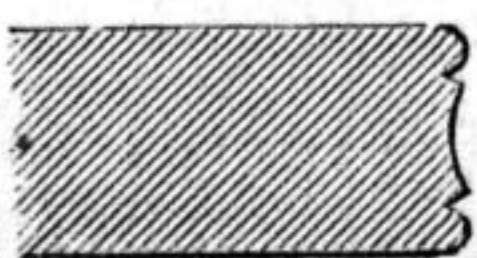
Fig. 5.—Section of Top, Bottom, and Shelves.
