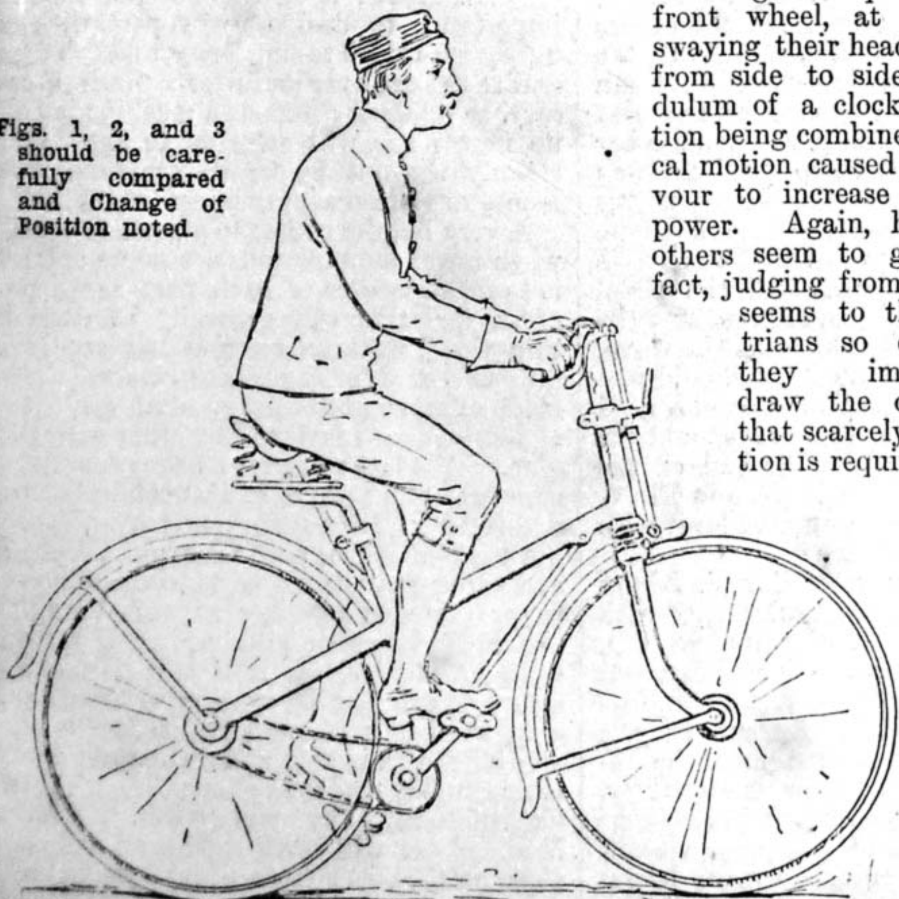
Fig. 2.—Rider on Seat too far back, but not so much as in Fig. 1.
