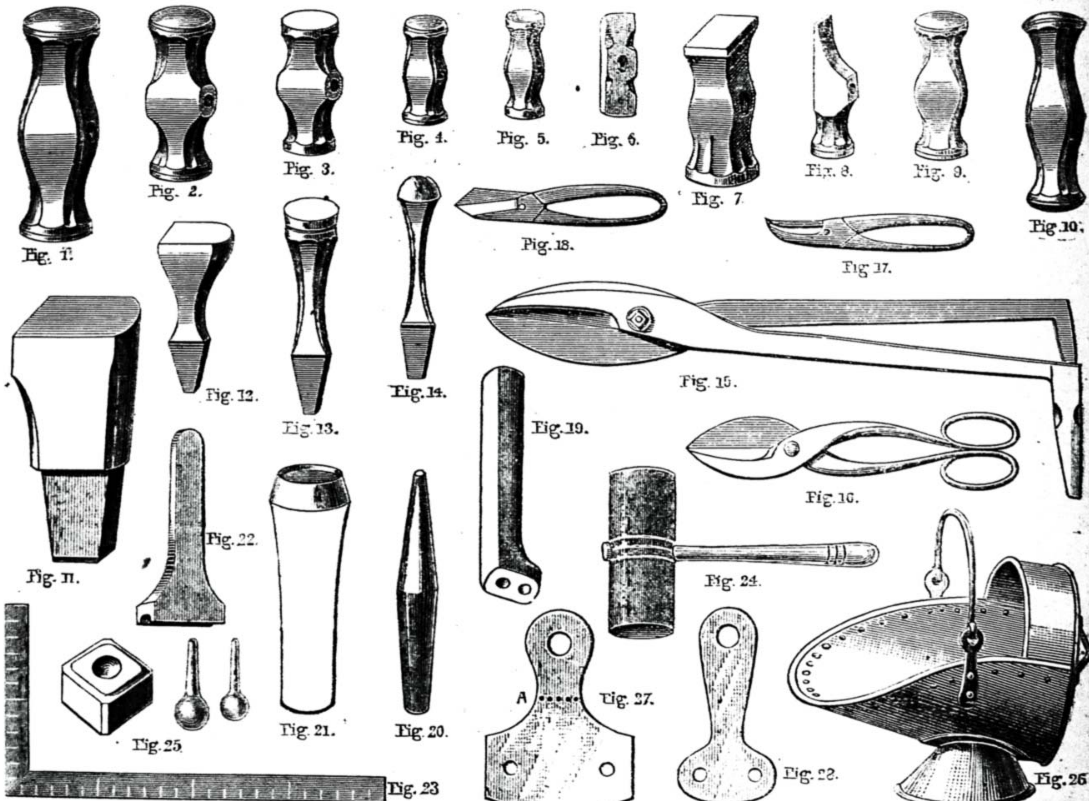
Figs. 1, 2.—Block Hammers. Fig. 3.—Planishing Hammer. Fig. 4.—Convex Hammer. Fig. 5.—Concave Hammer. Fig. 6.—Creasing Hammer. Fig. 7.—Square-faced Hammer. Fig. 8.—Rivetting Hammer. Fig. 9.—Block Hammer. Fig. 10.—Hollowing Hammer. Fig. 11.—Tinman's Anvil. Fig. 12.—Anvil Stake. Fig. 13.—Round Bottom Stake. Fig. 14.—Pepper-box Head. Fig. 15.—Stock Shears. Fig. 16.—Scotch Shears. Fig. 17.—Bent Snips. Fig. 18.—Straight Snips. Fig. 19.—Rivet Set. Fig. 20.—Solid Punch. Fig. 21.—Hollow Punch. Fig. 22.—Groove Punch or Groover. Fig. 23.—Tinman's Square. Fig. 24.—Tinman's Mallet. Fig. 25.—Stud Boss and Punches. Fig. 26.—Mode of re-lining Coal Scuttle. Fig. 27.—Stamped Ear. Fig. 28.—Forged Ear.
