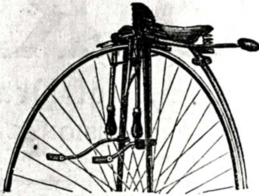
Fig. 5. — Perspective View of Bicycle, showing Fore Handle-bars depressed or hanging down, and the Rear Handle-bar up in Position for steering with.
