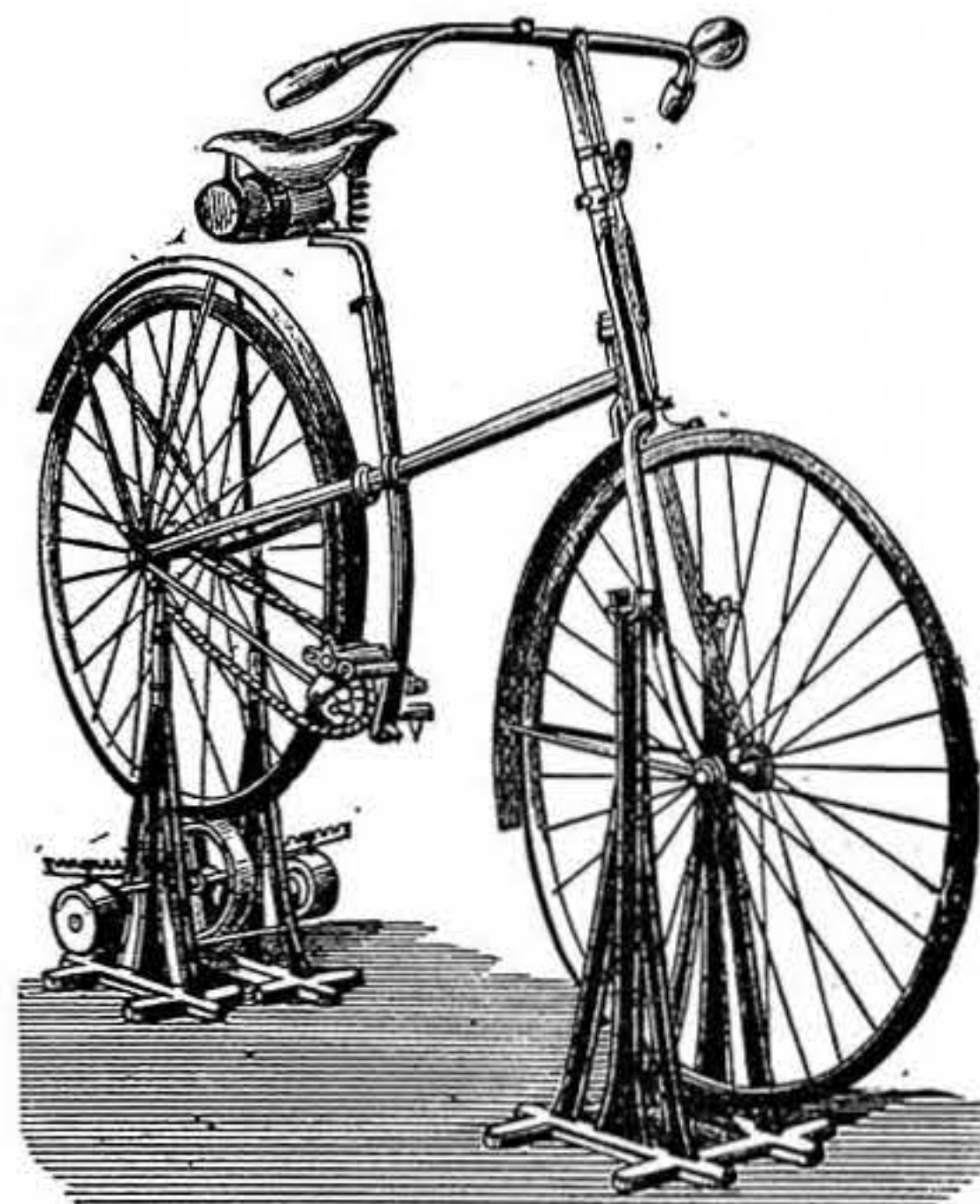
Fig. 1.—Bicycle on Hollier's Safety Stand.
