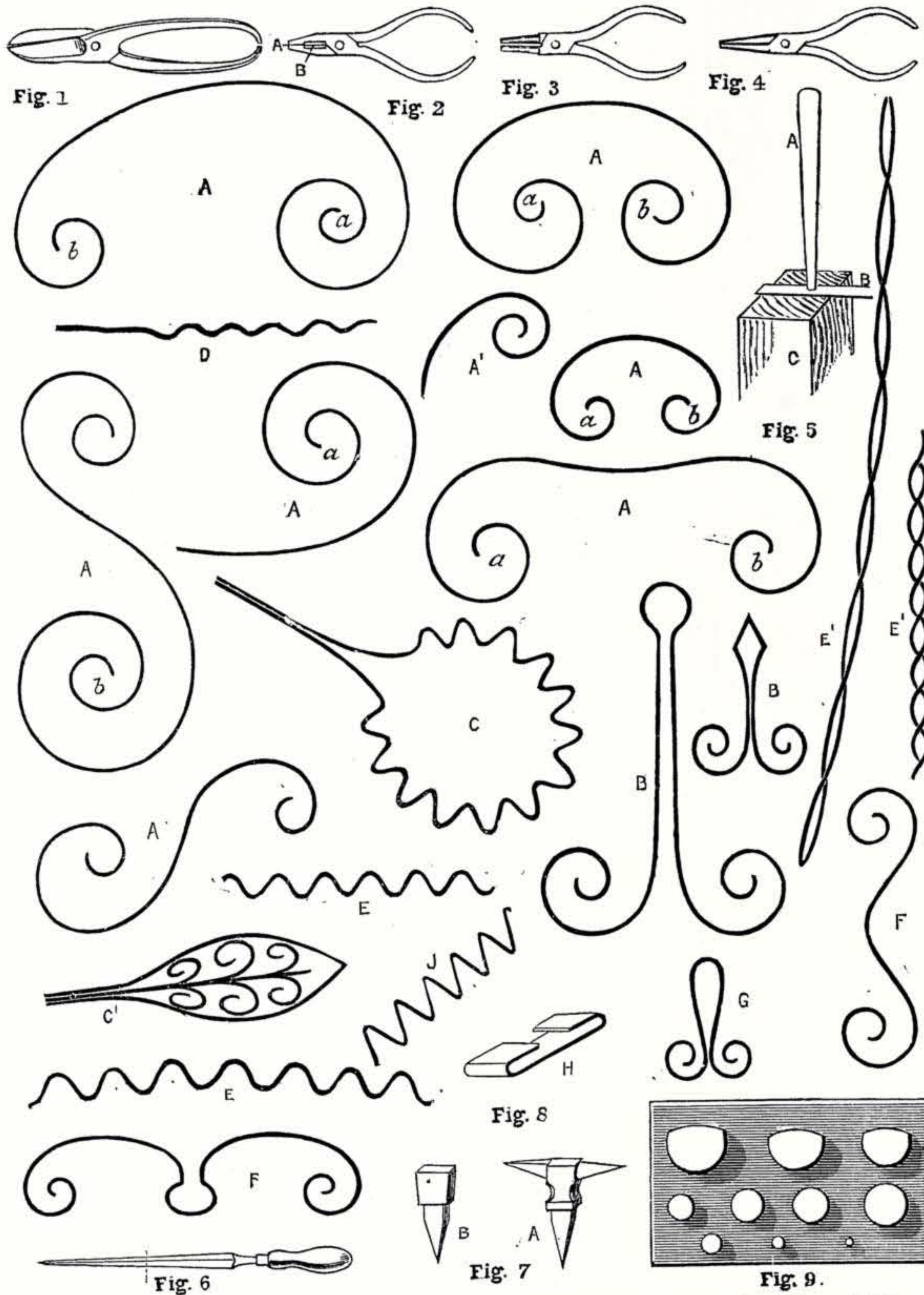
Bent Iron Work. Fig. 1.—Tinmen's Snips. Fig. 2.—Cutting Pliers. Fig. 3.—Round-nosed Pliers. Fig. 4.—Long-nosed Flat Pliers. Fig. 5.—Punching Holes in Iron. Fig. 6.—Rymer. Fig. 7.—Small Anvil and Stake. Fig. 8.—Elementary Curves and Forms. Fig. 9.—Templet Pins.
