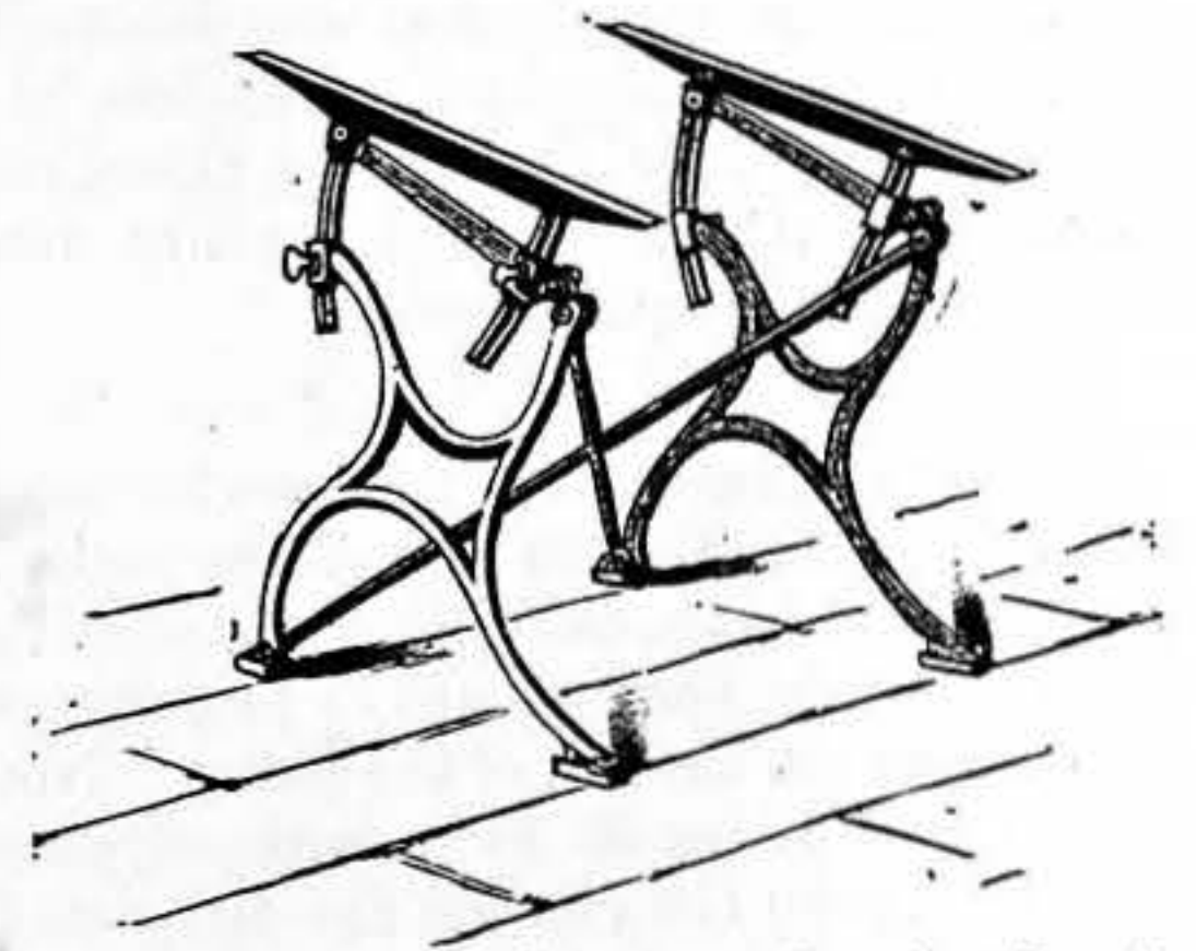
Fig. 3.—Adjustable Stand for Drawing-Board.
